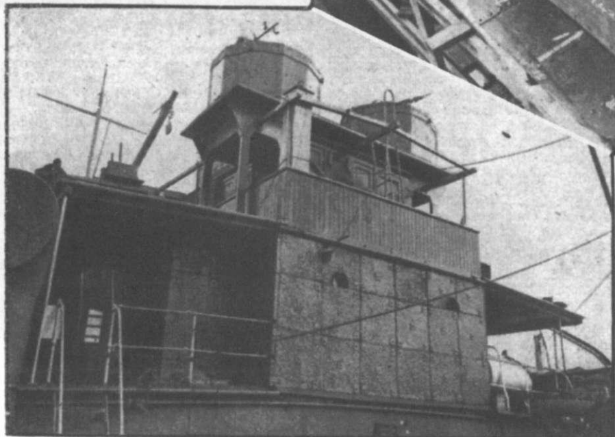
PLASTIC ARMOUR , a wartime innovation, details of which are still on the secret list, was successfully employed on our merchant ships against air attack. Above, it is being bolted over the well-deck of a vessel in the West India Docks, London. Gun-nests (left) on the ship's bridge were similarly reinforced.
