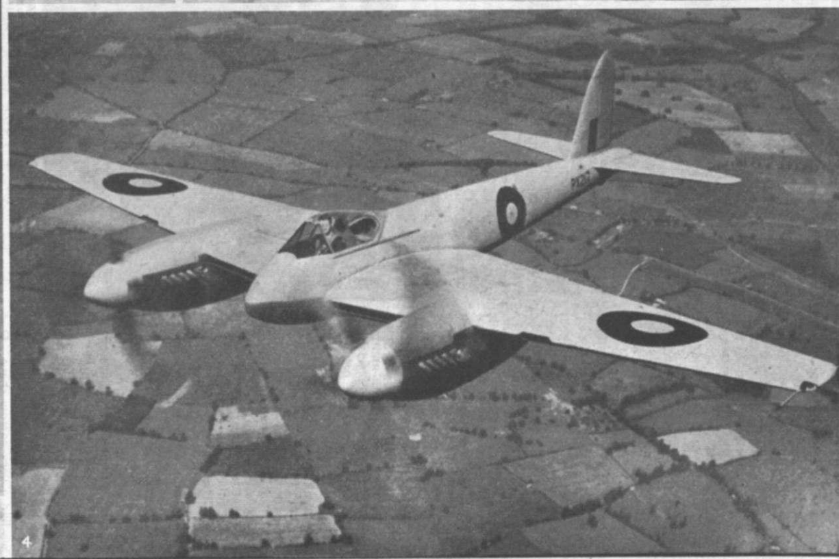
CLAIMED TO BE THE WORLD'S FASTEST FIGHTER is Britain's jet-propelled de Havilland Vampire (1) which first appeared over London on September 16, 1945. A single-seater, its speed is described as "handsomely in excess of 500 m.p.h." It is powered with a single gas turbine and was intended as an answer to the latest German jet-propelled aircraft. Designed for battle in the stratosphere is the Westland Welkin (2), the world's biggest single-seater fighter with a speed of 385 m.p.h. Off the secret list (September) is the Blackburn Firebrand (3), our Naval Air Arm's most formidable attack aircraft and fastest single-engined (2,580 h.p.) torpedo-carrying aircraft, with a speed of 350 m.p.h. Believed to be the fastest propeller-driven aircraft is the de Havilland Hornet (4), capable of over 470 m.p.h. Photos, Charles E. Brown
