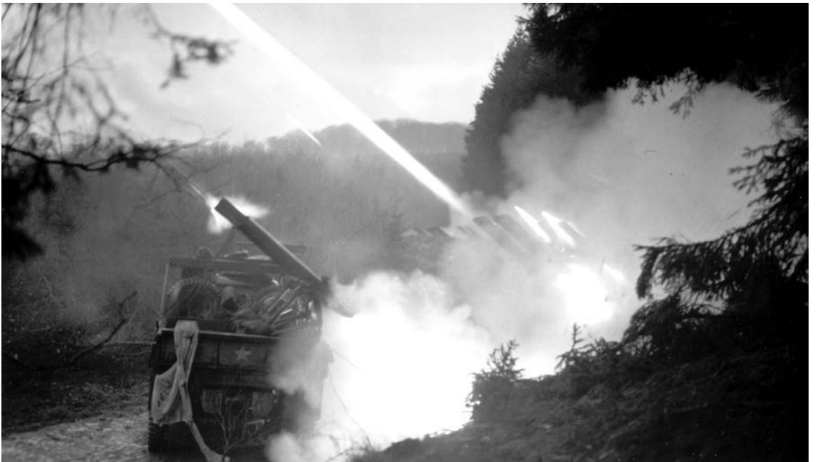
FIRING ROCKETS during the fighting in the Huertgen Forest area. In the above pictures 4.5-inch multiple rocket launchers T27 are mounted on 2½-ton trucks and consist of eight tubes in a single bank. Two banks are mounted on each of the trucks with the rockets being fired at half-second intervals.
