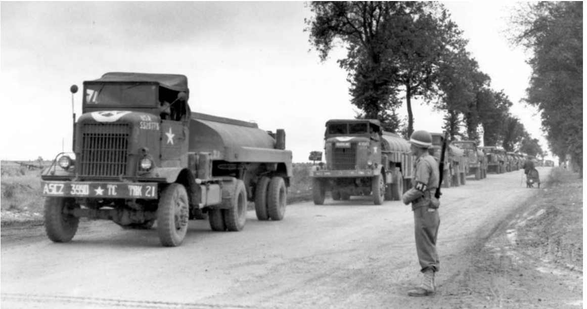
CONVOY CARRYING GASOLINE ALONG RED BALL HIGHWAY. These are 4–5-ton trucks (tractors) towing 2,000-gallon semitrailers (top). A 12-ton truck towing a 45-ton trailer loaded with ammunition, stops along Red Ball Highway (bottom). With the resistance offered by the retreating enemy at a minimum during this period, fuel was a more vital requisite than ammunition. Approximately a million gallons of gasoline were needed at the front every day to enable the armored columns to maintain their headlong rate of advance.
