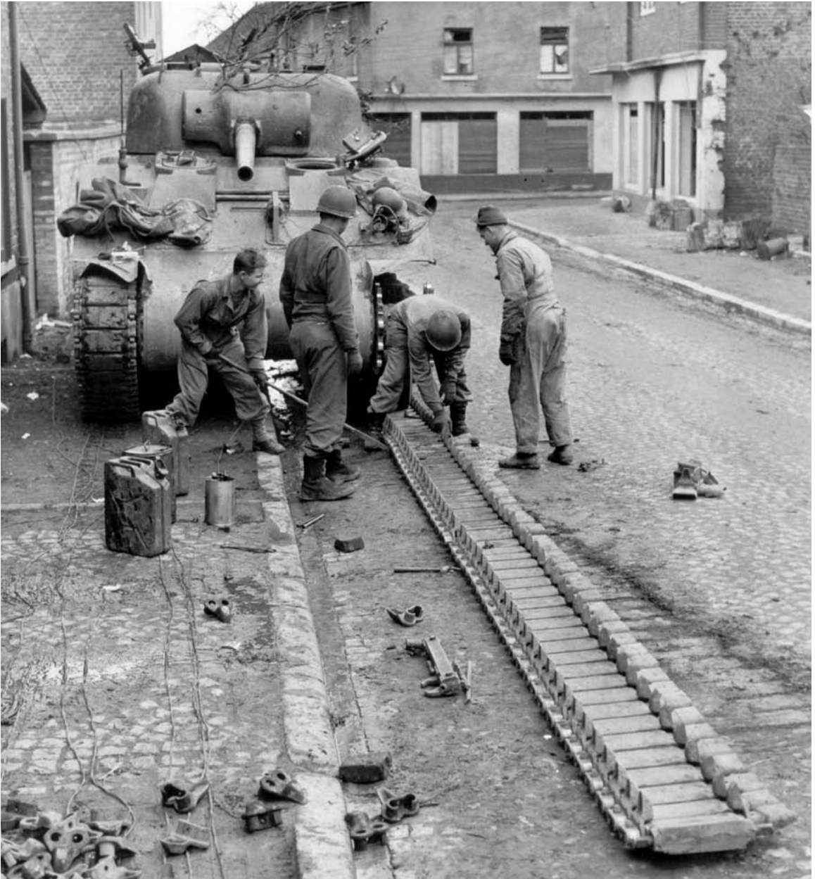
TRACK EXTENSIONS being put on the track of a medium tank. The maneuverability of tanks and other tracked vehicles was greatly hampered by mud along the front lines. Confronted by a problem more serious than anticipated, Ordnance personnel quickly designed and started production of track extensions at the rate of 156 separate pieces for each tank. Civilian manufacturing facilities were utilized in France and Belgium and before the program was completed 1,500,000 extensions had been made and welded to the tank tracks.
