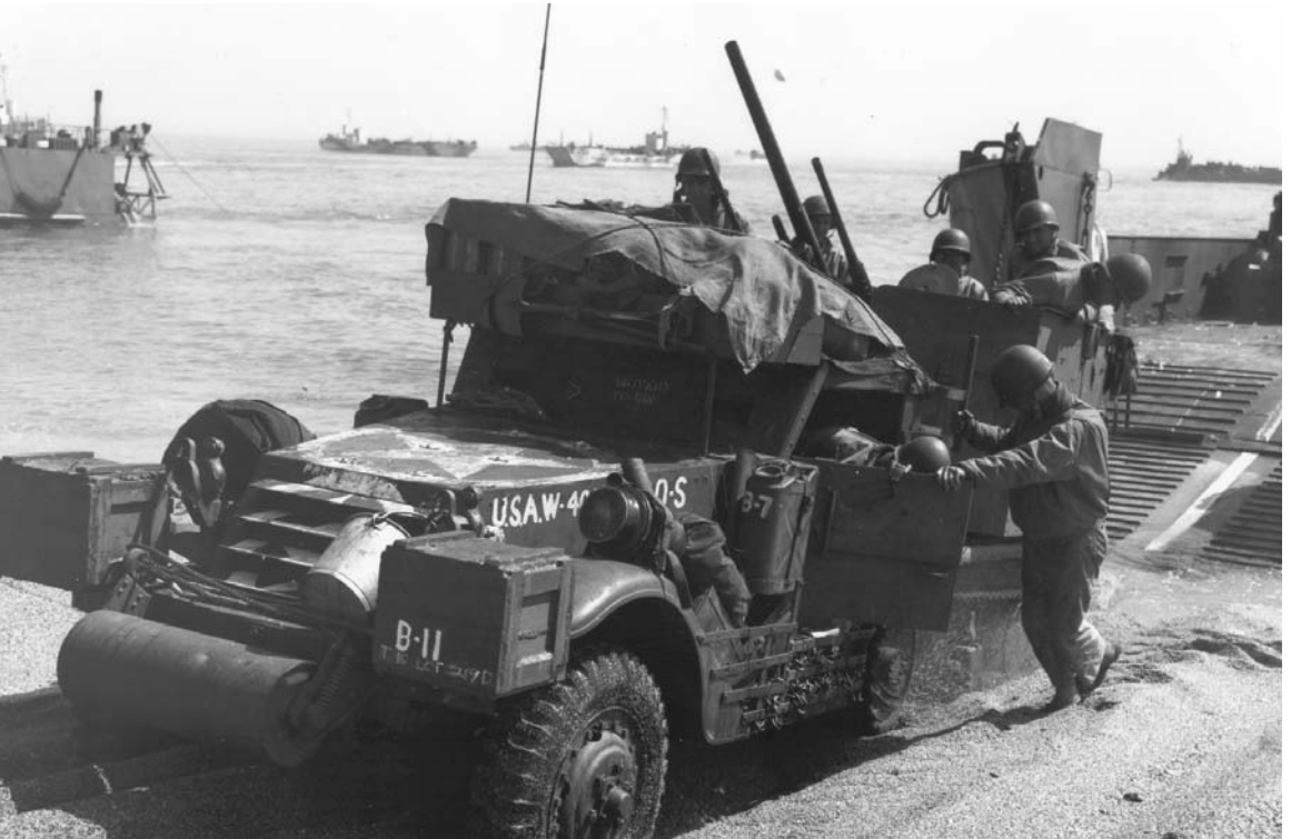
LANDING MANEUVERS. During late April and early May 1944 these were held for the invasion troops. Infantrymen landing from an LGI(L) (top). A combination gun motor carriage M15A1 landing on the beach from an LCT (bottom). This was a highly mobile weapon, capable of a concentration of rapid fire, and designed for anti-aircraft defense.
