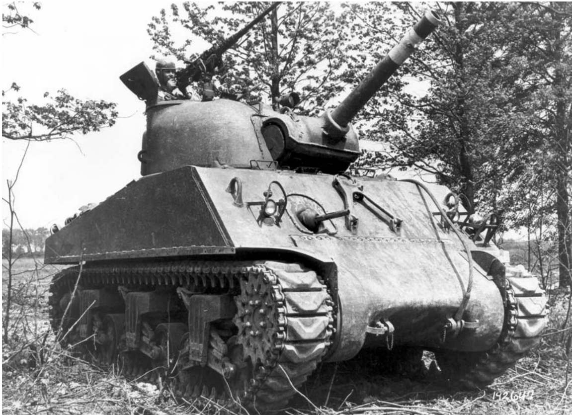
TWO TYPES OF U. S. TRACKED VEHICLES, each mounting a 105-mm. howitzer. 105-mm. howitzer motor carriage M7 (top); medium tank M4A3 with 105-mm. howitzer (bottom).
