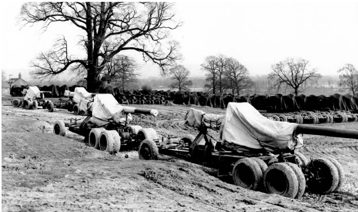
155-MM. GUNS AND 105-MM. HOWITZERS (top and bottom respectively) stored in England, 1944. After about 2,250 rounds had been fired, the barrel of the 155-mm. gun had to be replaced; in howitzers the number of rounds was higher.
