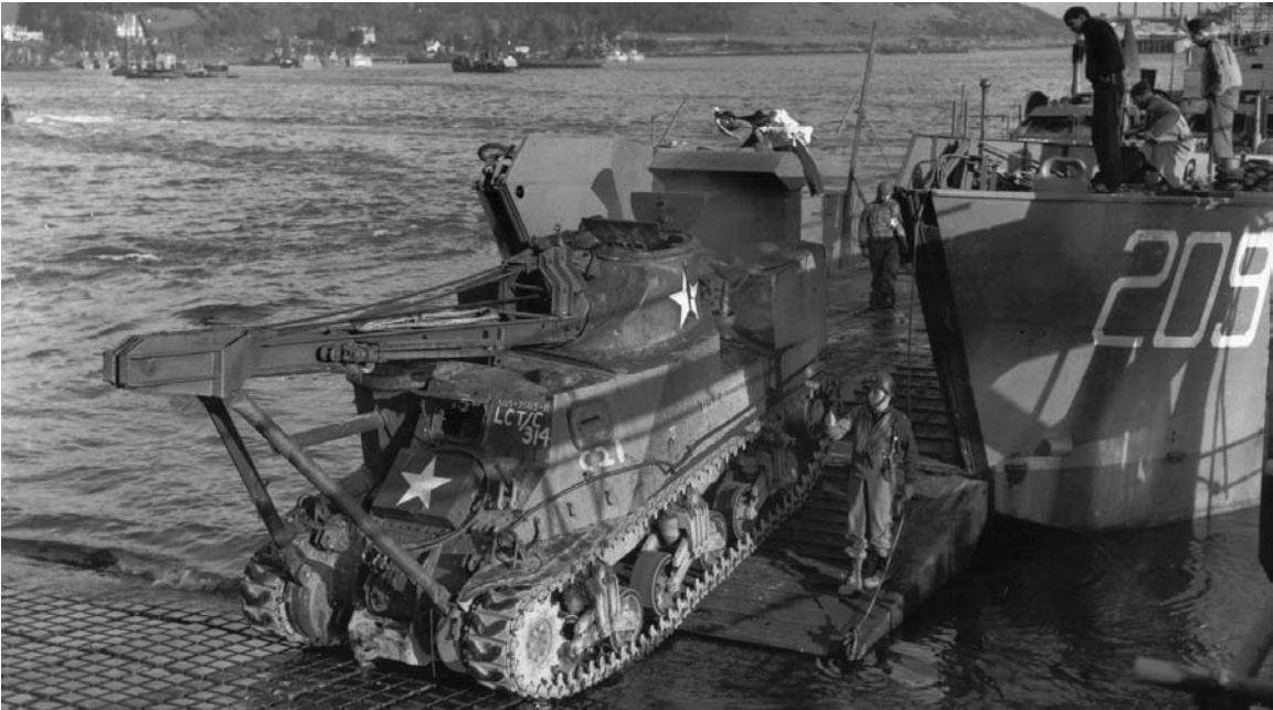
WATERPROOFED TANK RECOVERY VEHICLE M31 being loaded on an LCT during training along the English coast (top). For camouflage purposes, the normal appearance of the tank was retained as far as possible. A simulated turret without cupola was used and dummy 75-mm. and 37-mm. guns were mounted in place of the real guns. Actual armament was limited to two .30-caliber machine guns. A half-track 81-mm. mortar carrier M21 maneuvering on a road in England (bottom) . The mortar could be used on the vehicle or separate from it.
