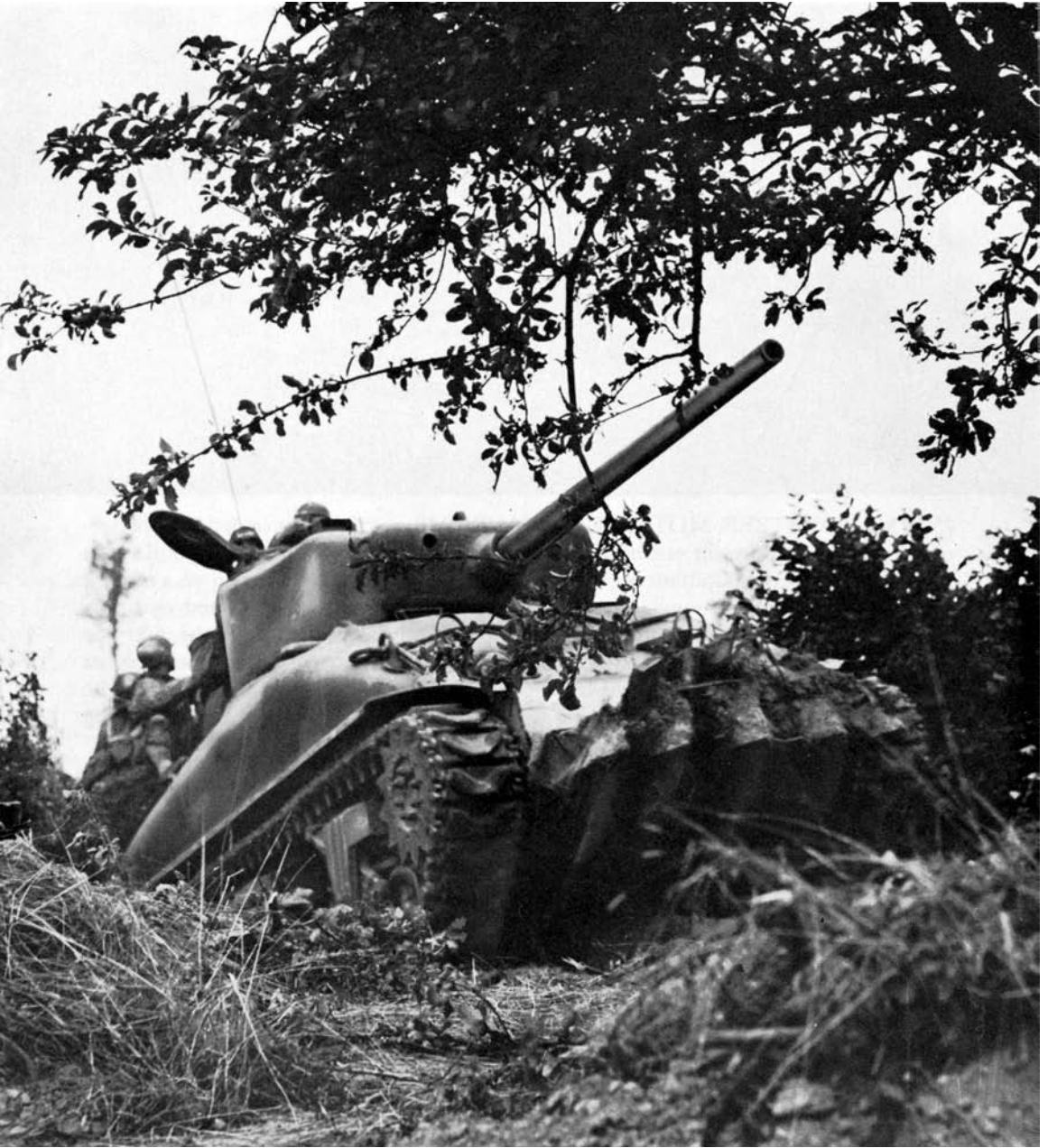
MEDIUM TANK M4A1, equipped with a hedgerow cutter, breaking through a hedgerow. The build-up was continuing generally as anticipated and the destruction of the enemy forces progressed. On 23 July 1944 the Canadian First Army became operational on the left flank of the Allied line. The Third U. S. Army had begun moving to the Cotentin Peninsula on 5 July and was proceeding on the right flank of the Allied line.
