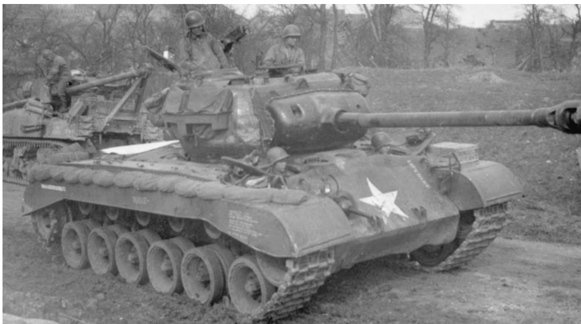
MEDIUM TANK M26 WITH A 90-MM. GUN equipped with a muzzle brake, introduced in combat early in 1945 (top). Both the light tank M24 and the medium tank M26 used a torsion bar type suspension which replaced the volute spring suspension of earlier models. Troops of the U. S. First Army approaching the Rhine (bottom). In the First Army area an attack was launched on 23 February simultaneously with that of the Ninth Army in the north. By 5 March First Army troops had secured all their initial objectives west of the Rhine.
