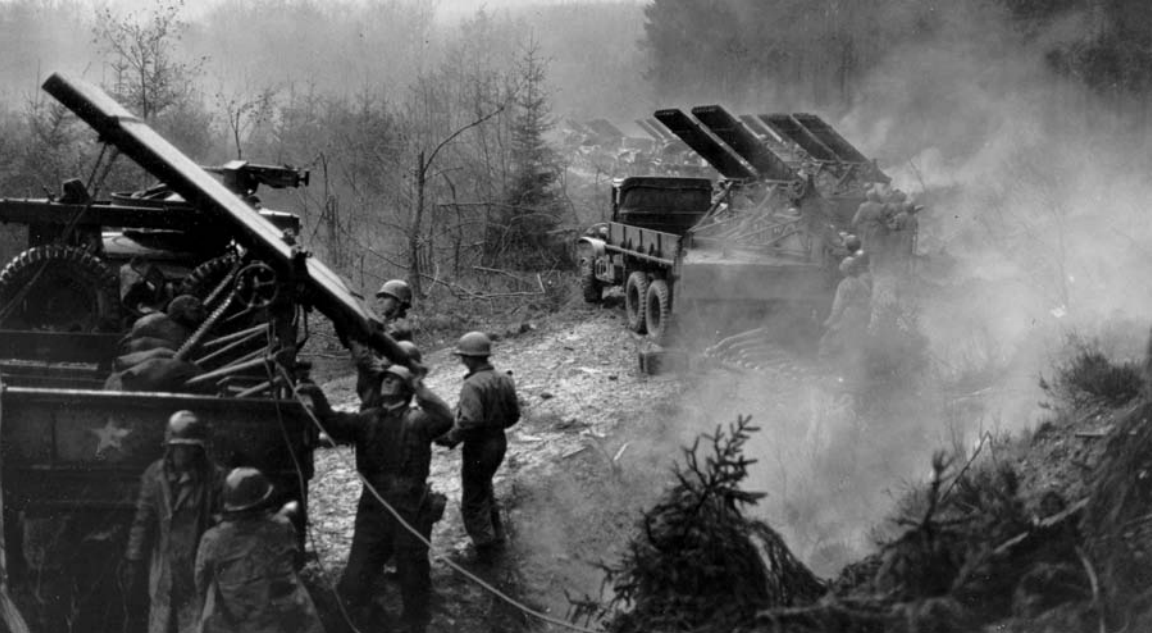
FIRING ROCKETS during the fighting in the Huertgen Forest area. In the above pictures 4.5-inch multiple rocket launchers T27 are mounted on 2½-ton trucks and consist of eight tubes in a single bank. Two banks are mounted on each of the trucks with the rockets being fired at half-second intervals.
