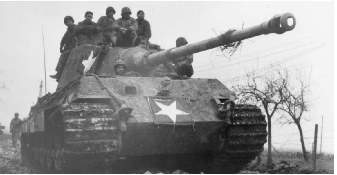
“KING TIGER” OR “ROYAL TIGER” ( Pz. Kpfw. VI (B) “Tiger” with 8.8-cm. Kw. K. 43) (top). This tank, weighing 75 tons and designed for defensive warfare or for penetrating strong lines of defense, made its appearance in combat in 1944. It had heavy frontal armor and an 88-mm. gun which could traverse 360 degrees. Germany heavy tank, the Panther ( Pz. Kpfw. with 7.5-cm. Kw. K. 42-L/70 ) (bottom). This tank, introduced in 1942, weighed 47 tons and had sloping frontal armor and a 75-mm. high-velocity gun.
