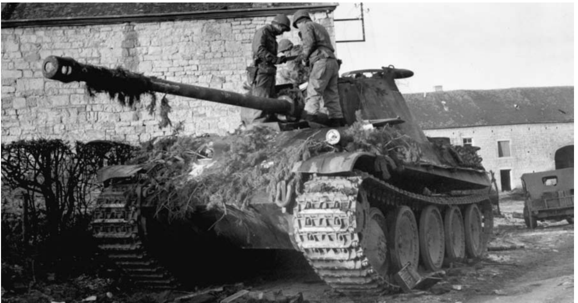
“KING TIGER” OR “ROYAL TIGER” ( Pz. Kpfw. VI (B) “Tiger” with 8.8-cm. Kw. K. 43) (top). This tank, weighing 75 tons and designed for defensive warfare or for penetrating strong lines of defense, made its appearance in combat in 1944. It had heavy frontal armor and an 88-mm. gun which could traverse 360 degrees. Germany heavy tank, the Panther ( Pz. Kpfw. with 7.5-cm. Kw. K. 42-L/70 ) (bottom). This tank, introduced in 1942, weighed 47 tons and had sloping frontal armor and a 75-mm. high-velocity gun.
