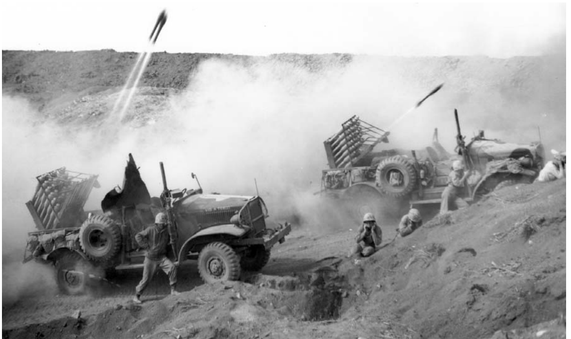
75-MM. GUN MOTOR CARRIAGES M3 FIRING at enemy positions on Iwo Jima (top). 4.5-inch automatic rocket launchers T45 mounted on two \frac{3}{4} -ton trucks, firing; this gravity-feed automatic launcher was developed as a Navy standard item for firing the 4.5-inch Navy barrage rocket (bottom)
