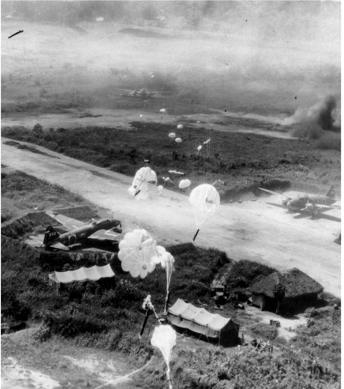
PARACHUTE BOMBS dropping from low-flying American planes during a raid over Rabaul. Parachute bombs were used to prevent self-destruction of the attacking low-flying bombers by the blasts of their own bombs. It was claimed that more than 200 enemy aircraft were destroyed or damaged on this raid, in addition to other materiel, ships, and installations.
