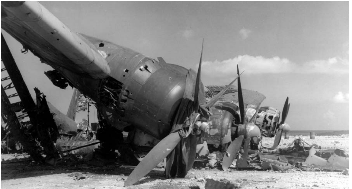
JAPANESE AIRCRAFT FOUND ON SAIPAN. A single-engine fighter plane (top) and the wreckage of bombers (bottom). Japanese aircraft markings usually consisted of a large red disc on the top and bottom of the outer section of each wing and on each side of the fuselage. The side marking was omitted on their Army aircraft but retained on Navy aircraft. Occasionally the red disc was surrounded by a narrow white line.
