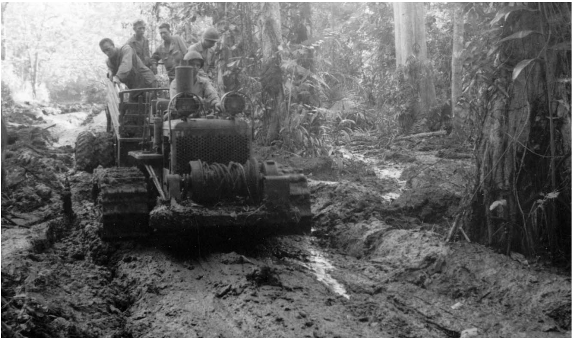
EQUIPMENT BEING FERRIED ACROSS A RIVER near Saidor (top). Crawler-type tractor with diesel engine plowing along a muddy road near Saidor; these tractors were mainly used to tow artillery and equipment over rough terrain (bottom). Tropical rains in this area greatly impeded the moving of supplies.
