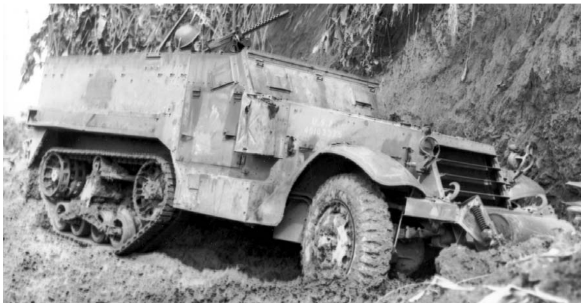
HALF-TRACK PERSONNEL CARRIER M3 mounting a .30-caliber machine gun parked at base of hill, its machine gun trained on a hillside target. This vehicle was used to bring men and supplies to the fighting lines and had seating capacity for thirteen men. The roller in front assisted in climbing out of ditches (top). Infantrymen, walking through a lane between barbed wire, carry 60-mm. mortar shells to the front lines (bottom).
