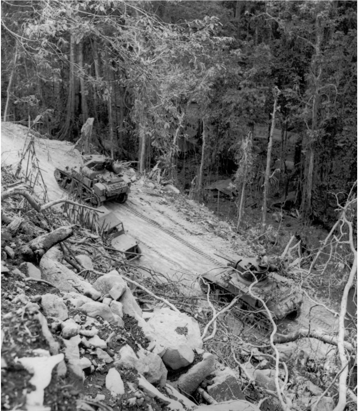
LIGHT TANKS M3A1, mounting 37-mm. guns and .30-caliber machine guns in a combination mount in the turret, going up a steep grade in an attempt to drive the Japanese from pillboxes on top of the hill, 9 March 1944. Between 8 and 25 March the enemy launched several major attacks against the Allied forces on Bougainville.
