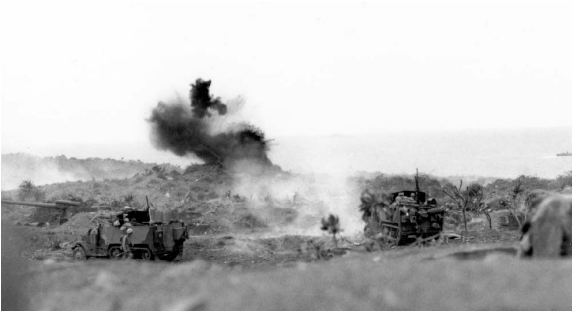
75-MM. GUN MOTOR CARRIAGES M3 FIRING at enemy positions on Iwo Jima (top). 4.5-inch automatic rocket launchers T45 mounted on two \frac{3}{4} -ton trucks, firing; this gravity-feed automatic launcher was developed as a Navy standard item for firing the 4.5-inch Navy barrage rocket (bottom)
