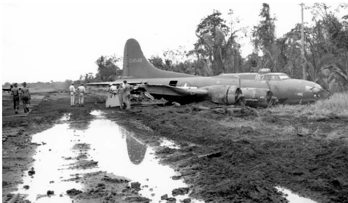
REMAINS OF A LIGHTNING FIGHTER PLANE P-38 which crashed during a landing (top), and a Flying Fortress B-17 which crashed when its right wheel gave way on an airstrip at Aitape (bottom). Since spare parts to maintain aircraft were difficult to obtain, maintenance men would strip crashed and crippled planes of usable parts almost before the engines cooled.
