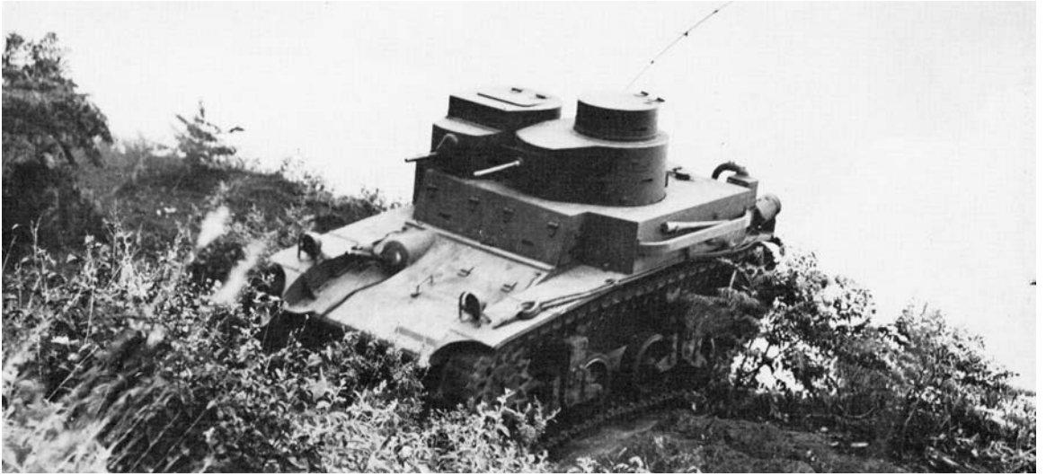
U.S. LIGHT TANK M2A2 during maneuvers on Oahu, 1942. This light tank with twin turrets, one containing a .50-caliber machine gun and the other a .30-caliber machine gun, was first manufactured in 1935. In December 1942, when it was declared obsolete, there were 234 left in the Army. The M2A2 light tank is a good example of the type of equipment available shortly after the entry of the United States into World War II.
