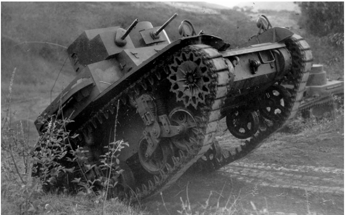
U.S. LIGHT TANK M2A2 during maneuvers on Oahu, 1942. This light tank with twin turrets, one containing a .50-caliber machine gun and the other a .30-caliber machine gun, was first manufactured in 1935. In December 1942, when it was declared obsolete, there were 234 left in the Army. The M2A2 light tank is a good example of the type of equipment available shortly after the entry of the United States into World War II.
