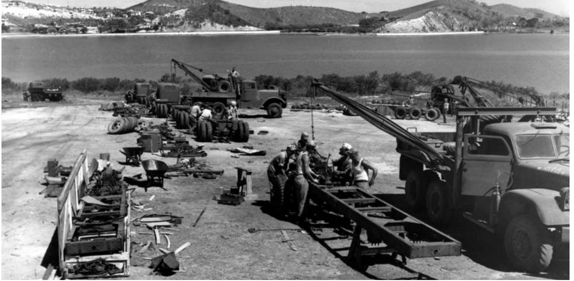
MEN OF AN ORDNANCE UNIT ASSEMBLING VEHICLES which had arrived crated in sections. By October 1942 twenty-five men were completing six vehicles a day on this assembly line.
