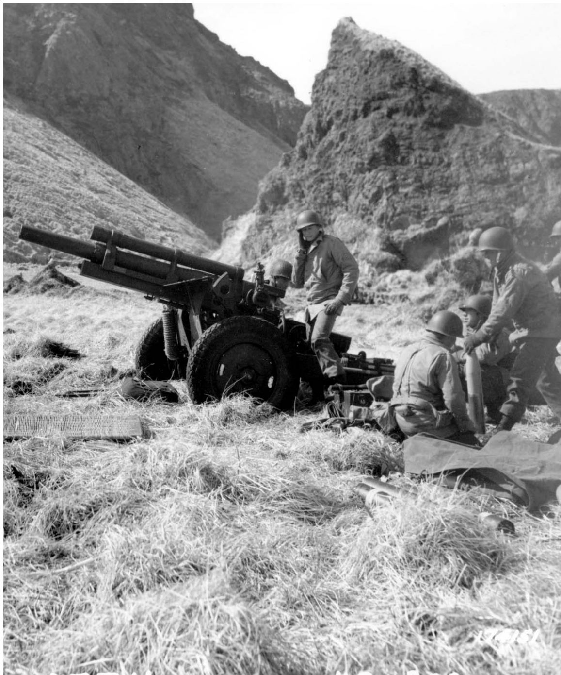
105-MM. HOWITZER M2A1 in position inland from the Holtz Bay beachhead. The gun crews worked in haste to set up their artillery pieces as contact was expected with the enemy at any moment.
