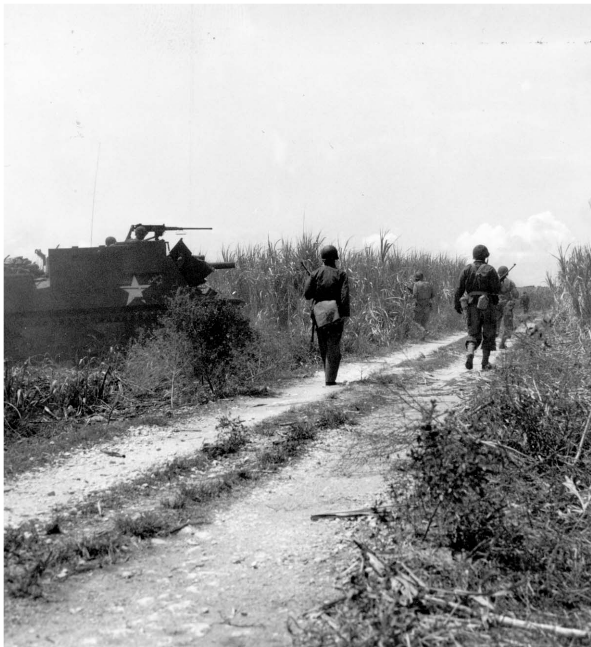
INFANTRYMEN ADVANCING ALONG A ROAD ON SAIPAN to blast an enemy pillbox beyond the next ridge. The 105-mm. howitzer motor carriage M7 in the left background was called the "Priest." This vehicle was based on a medium tank M3 chassis. During the night of 6-7 July the enemy made a massed counterattack which gained some ground and inflicted heavy losses on U.S. troops. The lost ground was recovered by the end of the 7th and the advance was renewed the next day.
