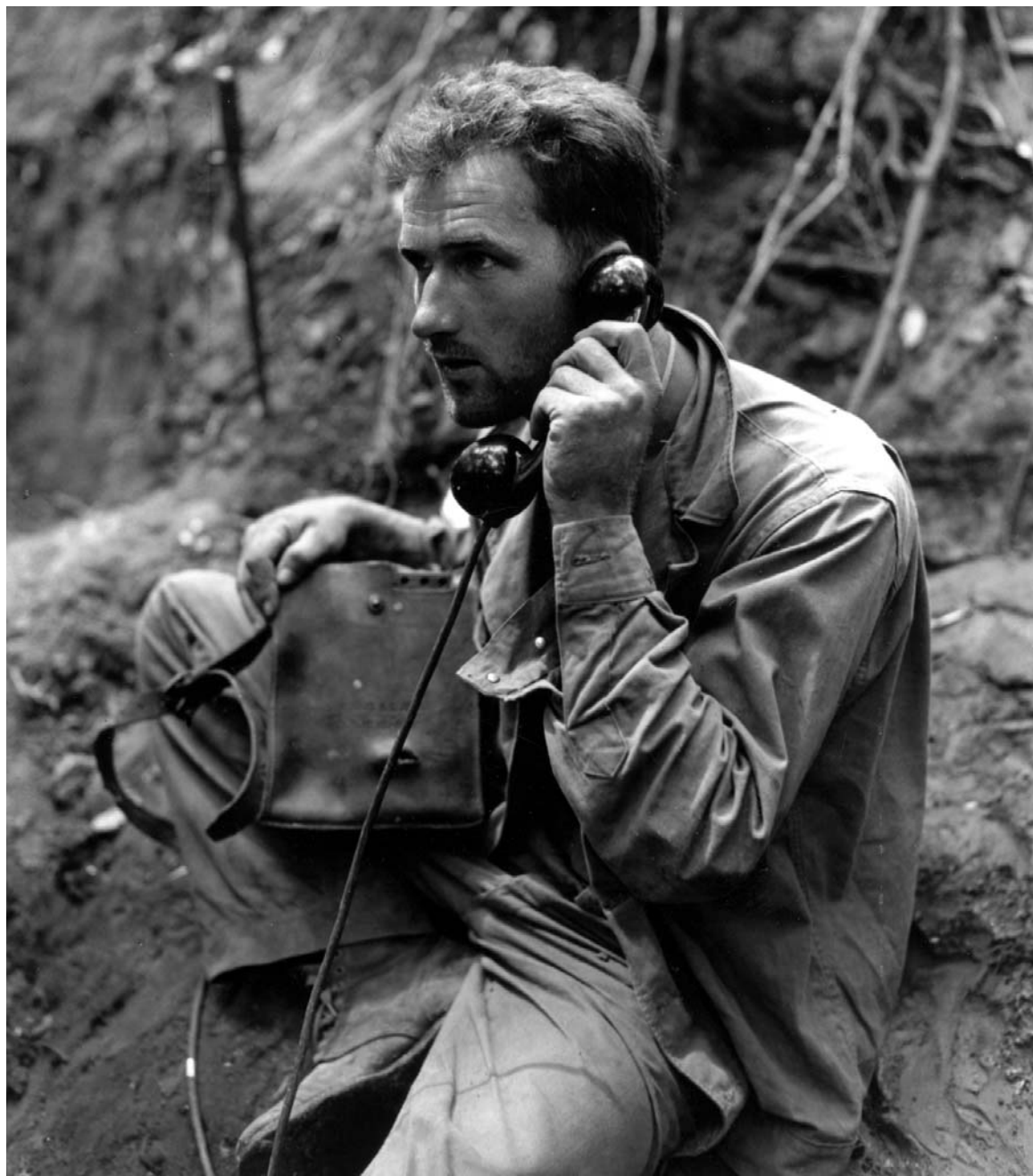
FIELD TELEPHONE, still in working order after being hit by a shell fragment when a Japanese “knee-mortar” shell landed six feet away. In the absence of reliable radio communications, wire communications were heavily relied upon. The EE-8 field telephone and the sound-powered telephone were used for long and short distances, respectively.
