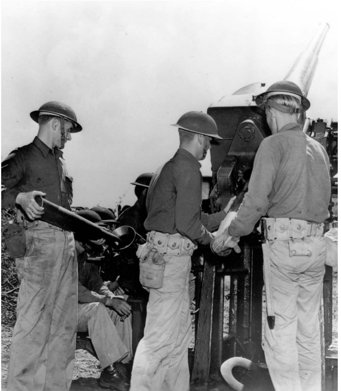
COAST ARTILLERY BATTERY training in Hawaii. Man at left is placing a round in the manual fuze setter of a 3-inch anti-aircraft gun M1917M2. A plan for the defense of the Hawaiian Islands had been set up and joint maneuvers (land, air, and naval forces) were held periodically to test the various security measures.
