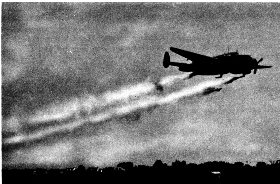
LOCKHEED A-29 SPRAYING SMOKE FROM M33 SMOKE TANKS visible under wings of craft. Smoke tank protruding from bomb bay is the M33 A-1.
