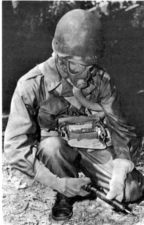
M9 CHEMICAL DETECTOR KIT. Developed at Edgewood Arsenal in 1944, the M9 kit was one of several devices used to determine presence and type of toxic chemicals.
