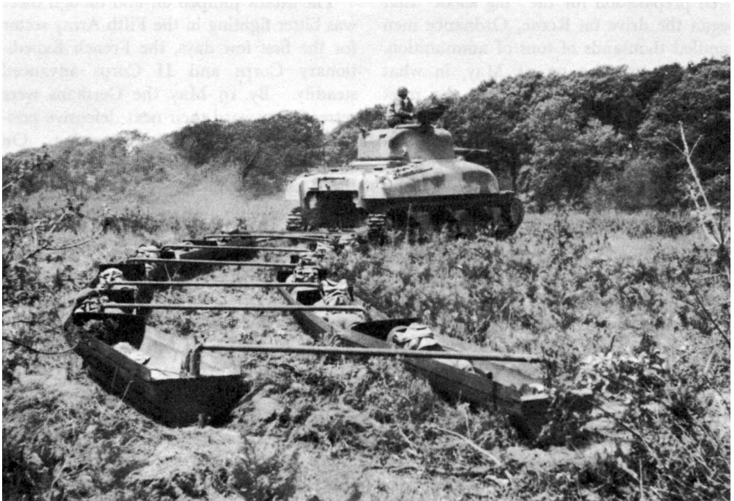
M4 TANK PULLING BATTLE SLEDS AROUND A CURVE to demonstrate sleds' flexibility, Nettuno, Italy.
