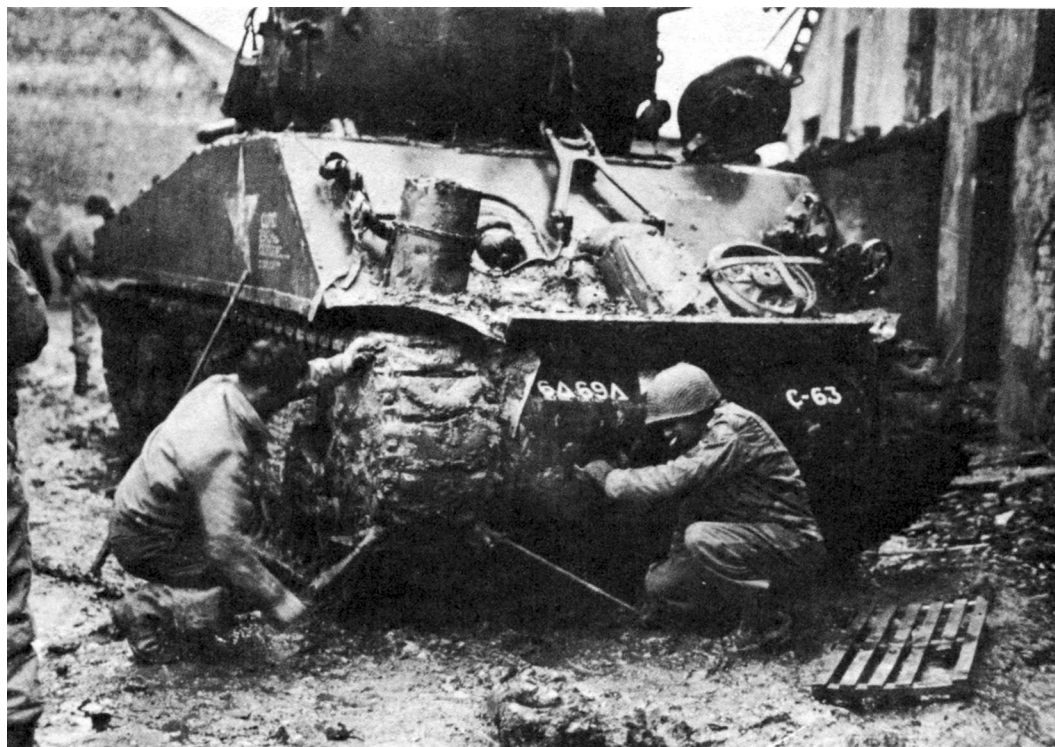
REPLACING TRACKS ON A SHERMAN TANK
