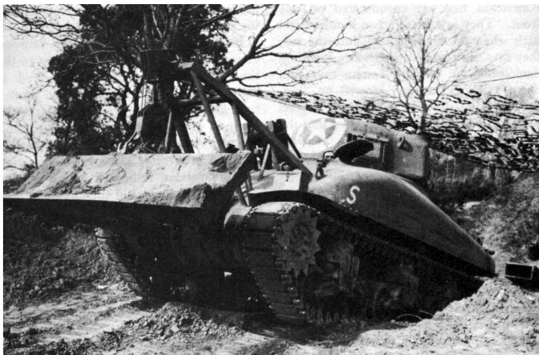
TANKDOZER USED TO FIGHT AMMUNITION DUMP FIRES, ANZIO
