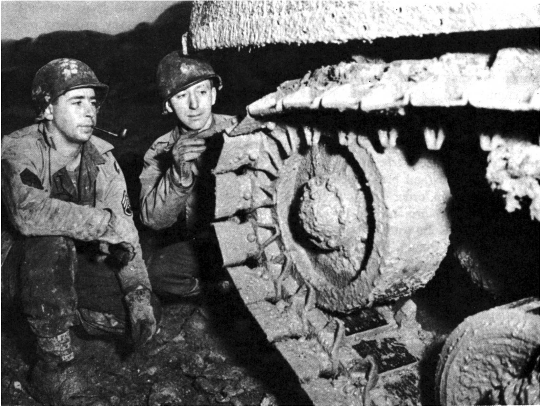
INSPECTING DUCKBILL EXTENSIONS ON TANK TRACKS
