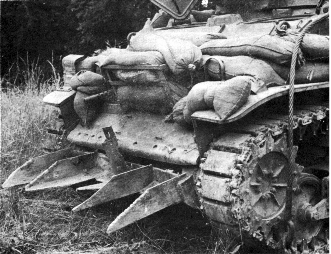
TANK WITH HEDGEROW CUTTER AND SANDBAGS
