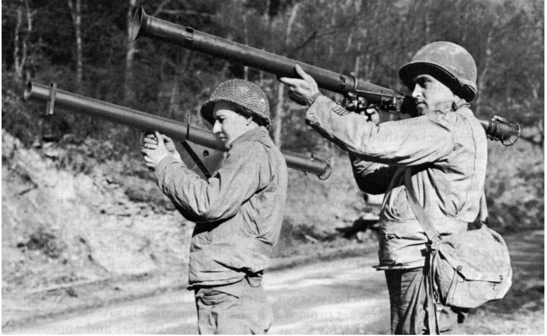
THE BAZOOKA. The original 2.36-inch model M1 is shown at left, the improved model M9 at right.
