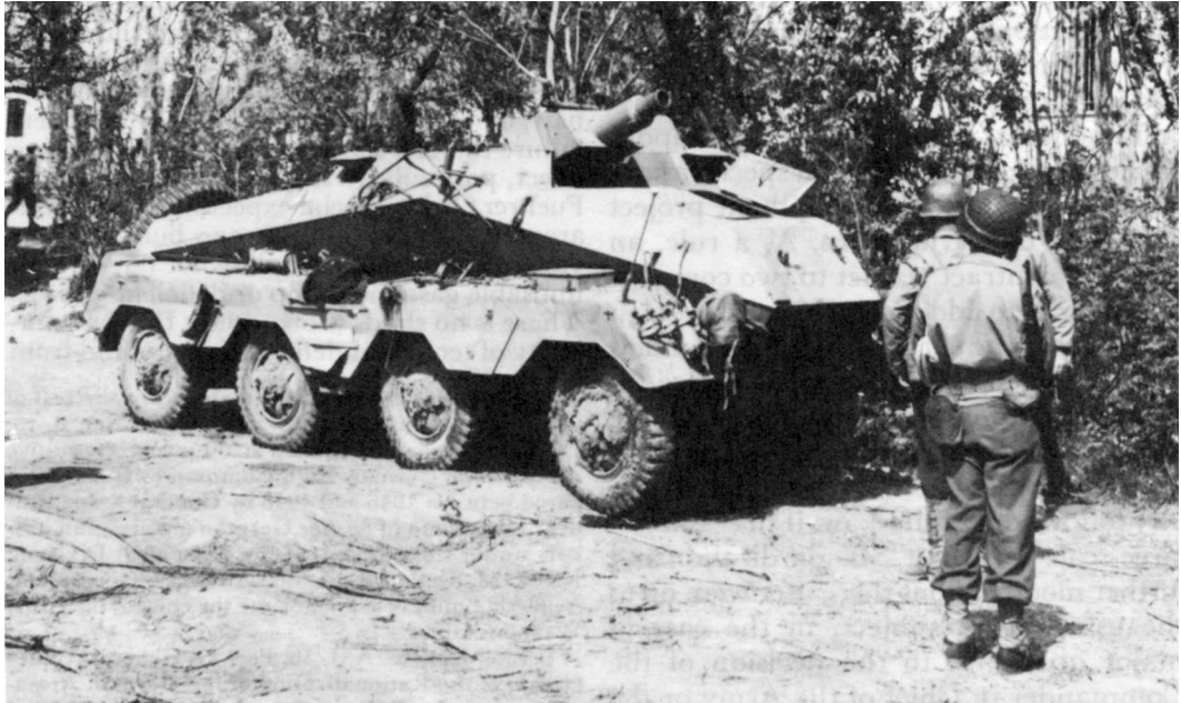
8 RAD PANZERSPAHWAGEN, mounting the 7.5-cm. short-barreled gun.
