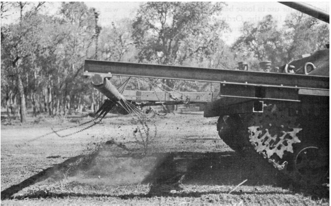
MINE EXPLODERS. The driven-disc type T1E3 (above), and the "Scorpion" type (below).
