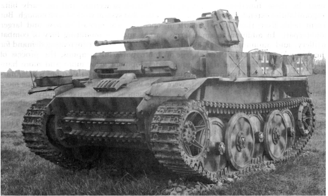
PANZER II, THE "LYNX," mounting a 2-cm. gun.
