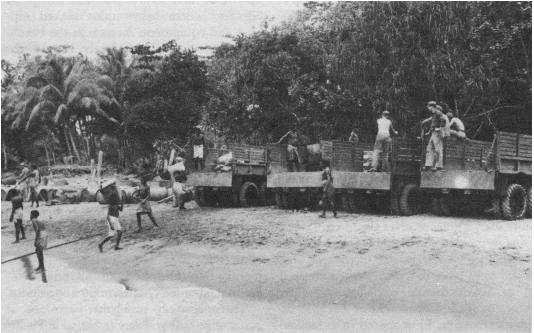
TRUCKS OPERATING FROM THE BEACHES rapidly became unserviceable owing to the action of salt water and sand on the moving parts.
