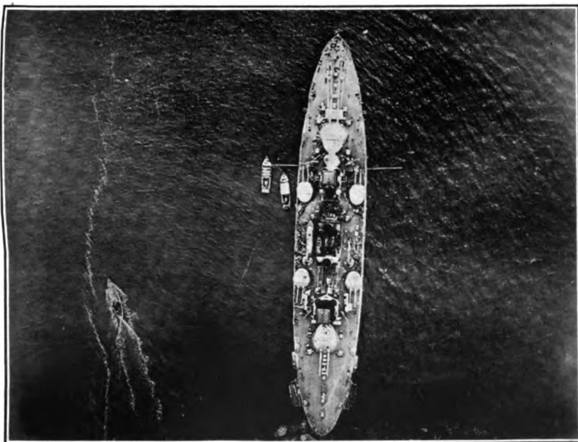
VIEW OF A BATTLESHIP FROM A HYDROPLANE, SHOWING 12-INCH AND 8-INCH TURRETS.
