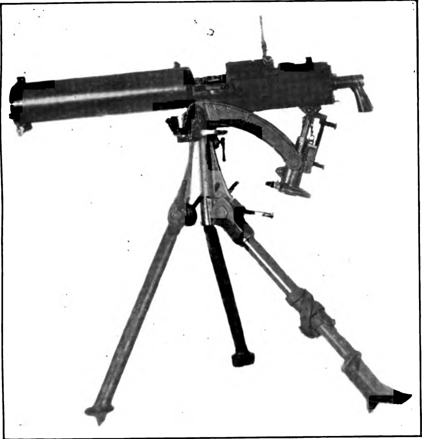
HEAVY BROWNING MACHINE GUN.
