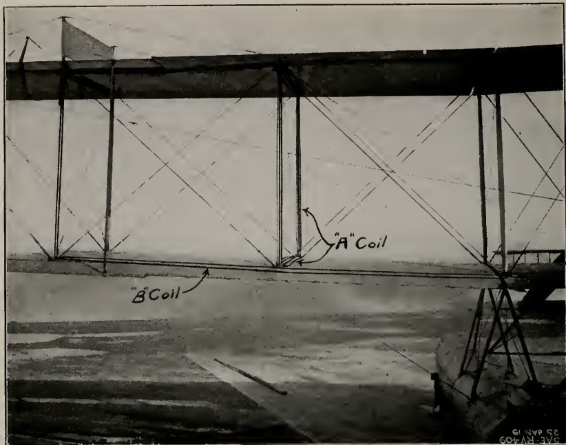
FIG. 19.—RADIO COMPASS COILS IN WINGS OF AIRPLANE.
