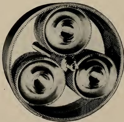
REDUCTION GEAR FOR EAGLE ENGINES.
