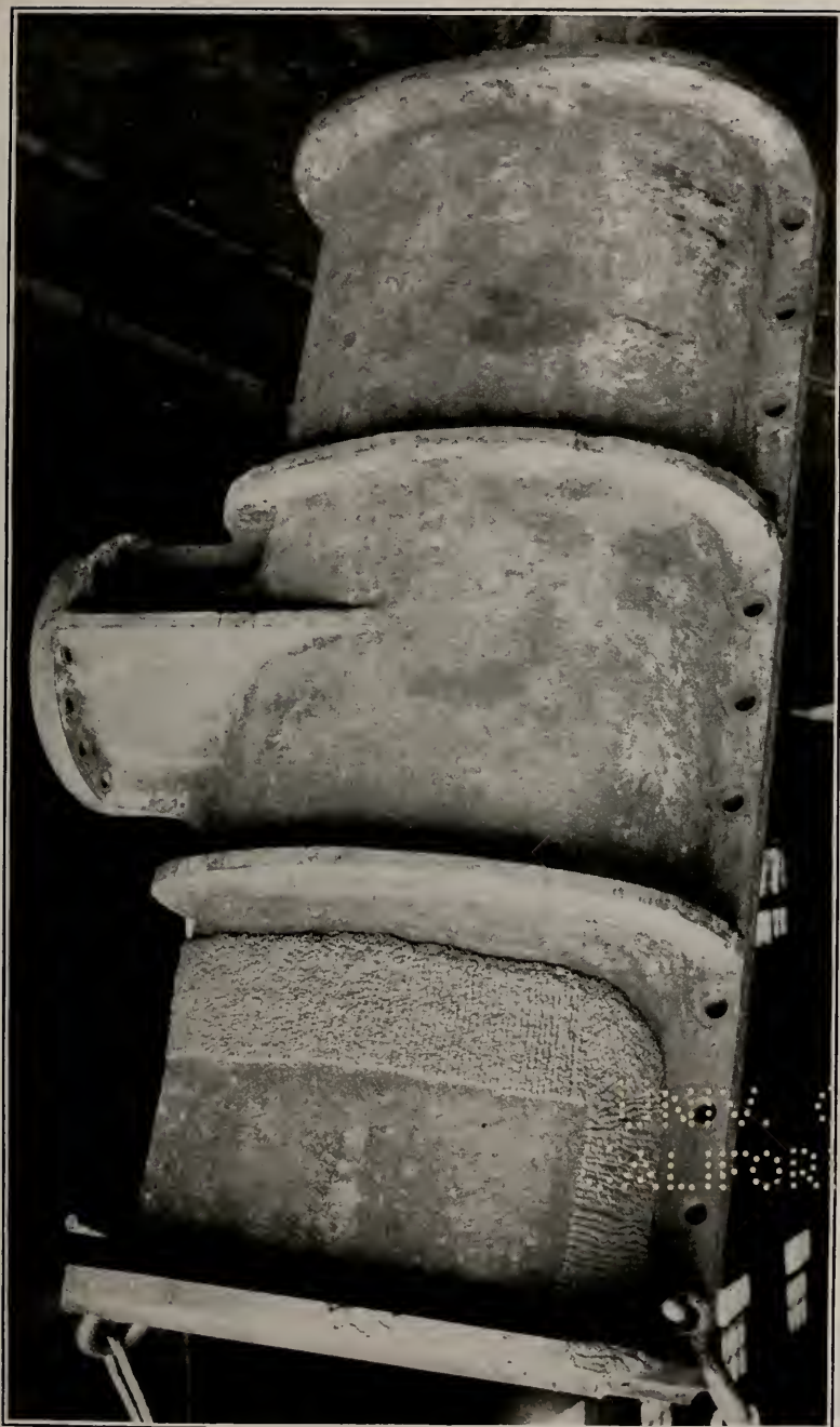
S. S. SANTOS: SECOND I. P. VALVE CHEST AFTER WELDING AT NAVY YARD, PHILADELPHIA, PA.
