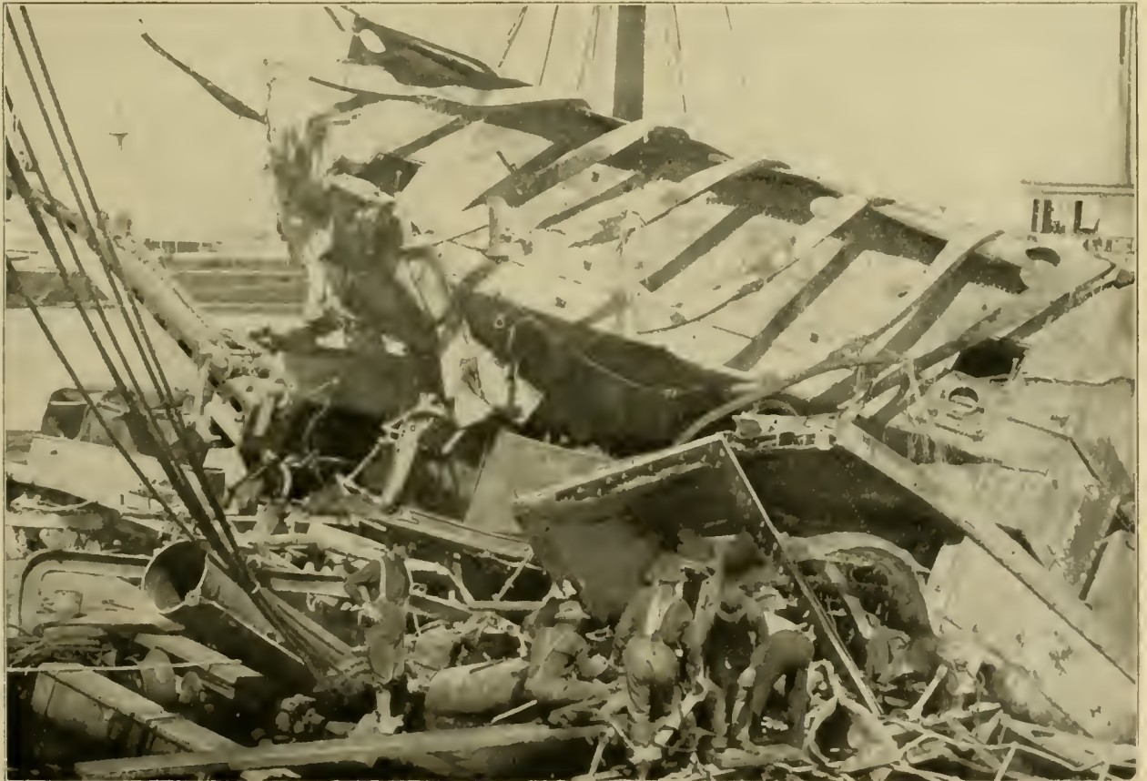
Wreck of the Battleship Maine—View Amidships, Showing the Upheaval of Armor-plate and the Destruction Wrought
