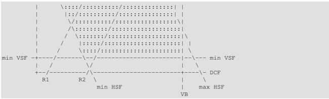
This is a generic monitor mode diagram. The x axis of the diagram shows the clock rate (DCF), the y axis represents the refresh rate (RR). The filled region of the diagram describes the monitor's capabilities: every point within this region is a possible video mode.
