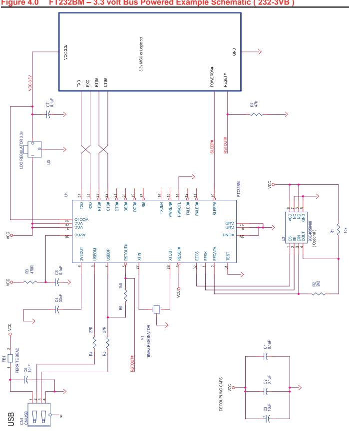
FT232BM – 3.3 volt Bus Powered Example Schematic (232-3VB) Figure 4.0
