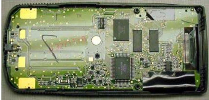
Component side of PCB with shield removed
