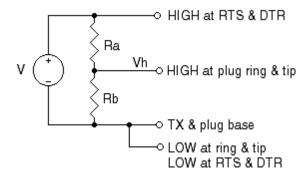
The voltage source V may be a power supply or even a 9V battery. The two resistor Ra and Rb set voltage Vh, and simulate the 10K source impedance of the calculator data lines. For a desired source impedance Rs and output voltage Vh, use these equations to find Ra and Rb:
