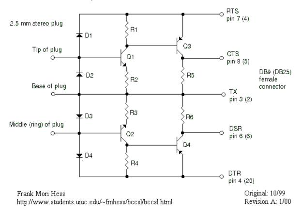
The schematic for the original cable is shown above. The connection to the computer may be either a DB9 or a DB25 connector; the DB25 pin numbers are shown in parentheses. The GraphLink plug which connects to the calculator is a 3-conductor (stereo) 2.5 mm connector. The three conductors are named like this:
