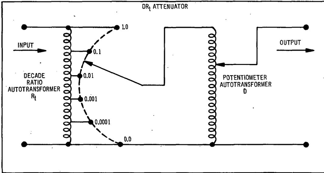
Fig. 4-4. Schematic showing components in the  $DR_t$  attenuator.
