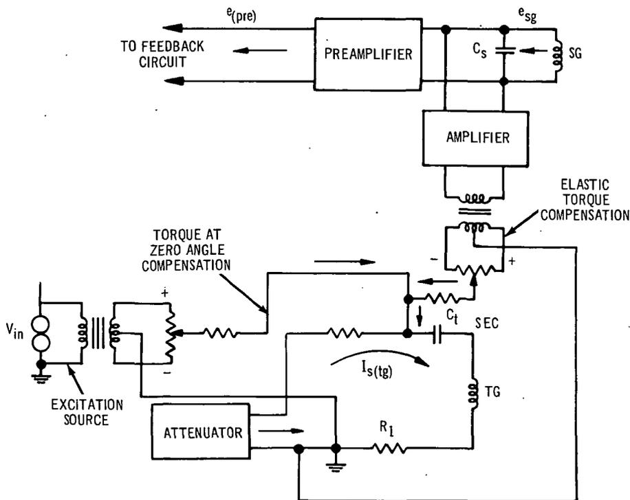
Fig. 6-3. Schematic diagram for the reactor torque compensation.
