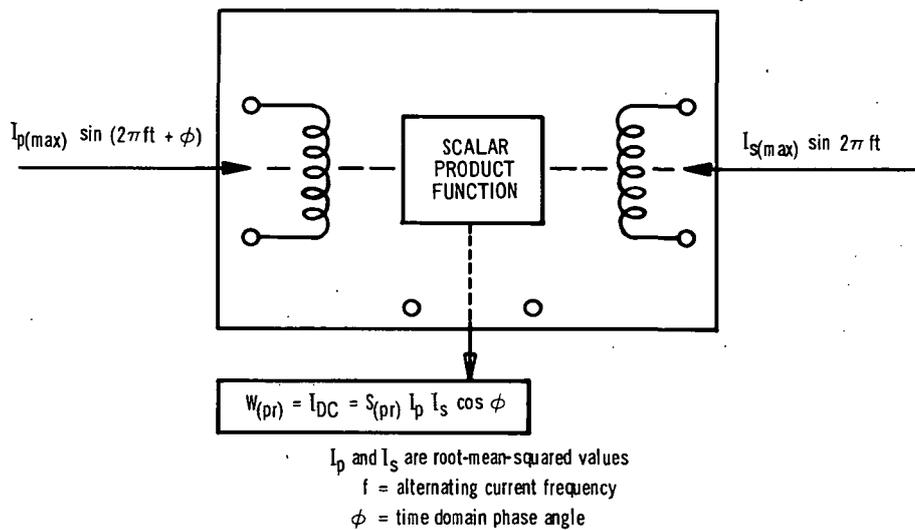
Fig. 4-3. Current-product resolver functional schematic.
