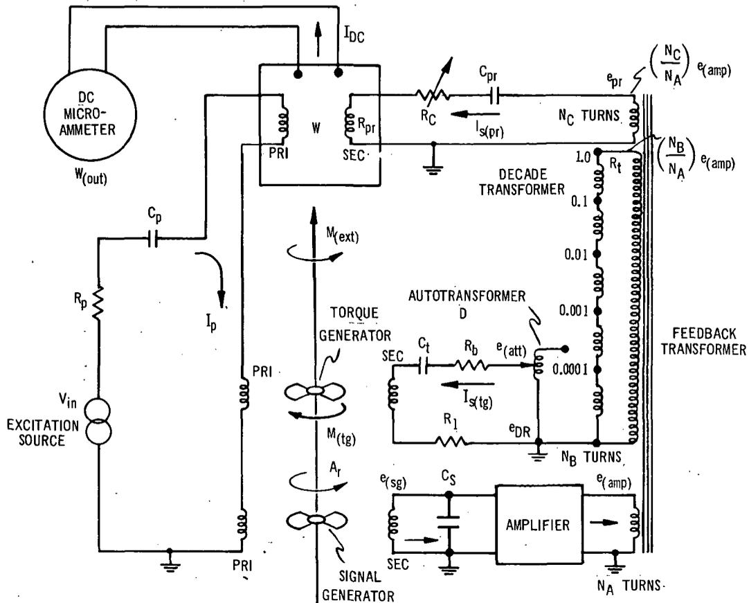
Fig. 4-1. Measuring torque by the proportional elastance method, with current-product readout.
