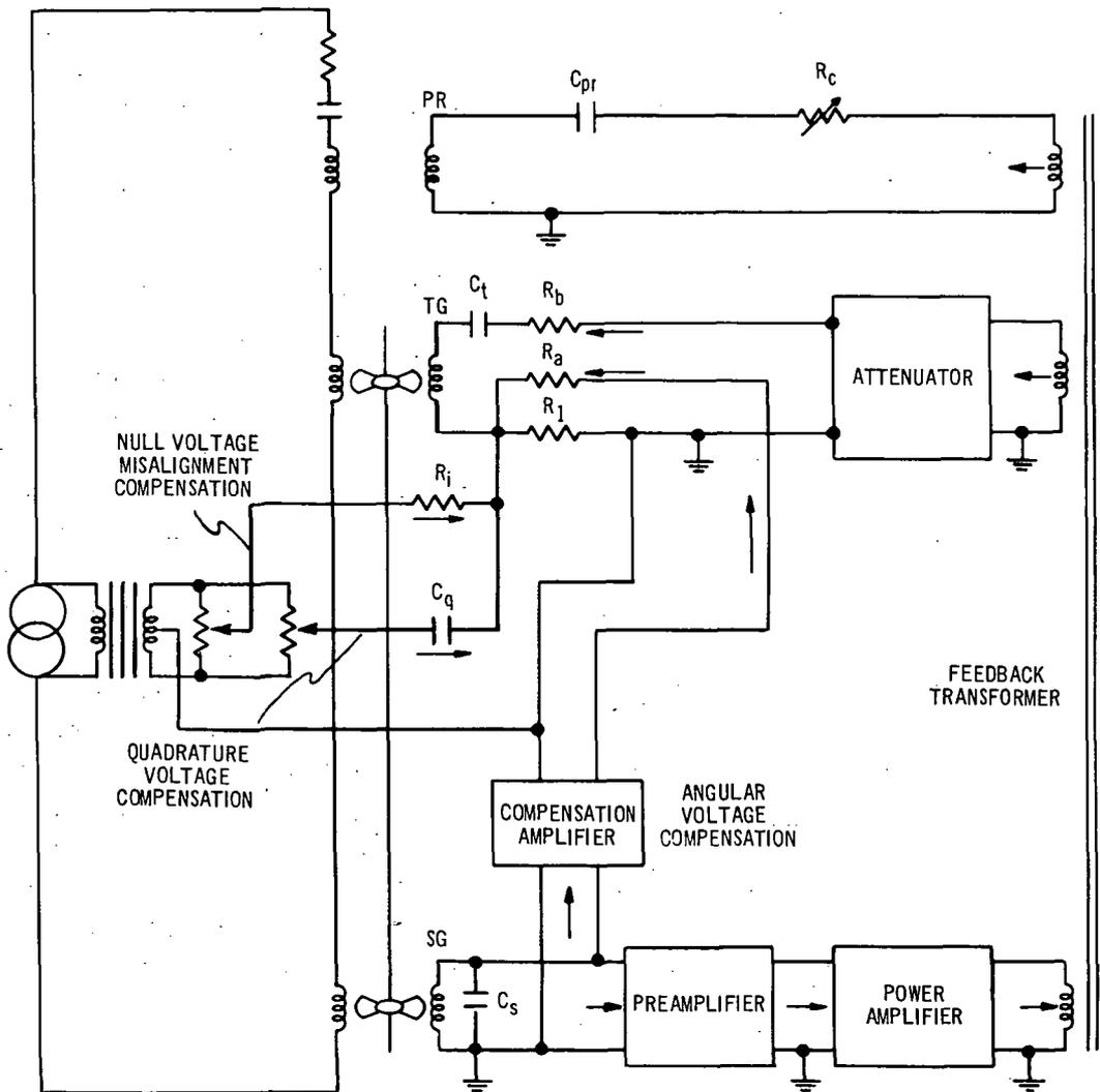
Fig. 6-5. Torque generator back-emf compensation.
