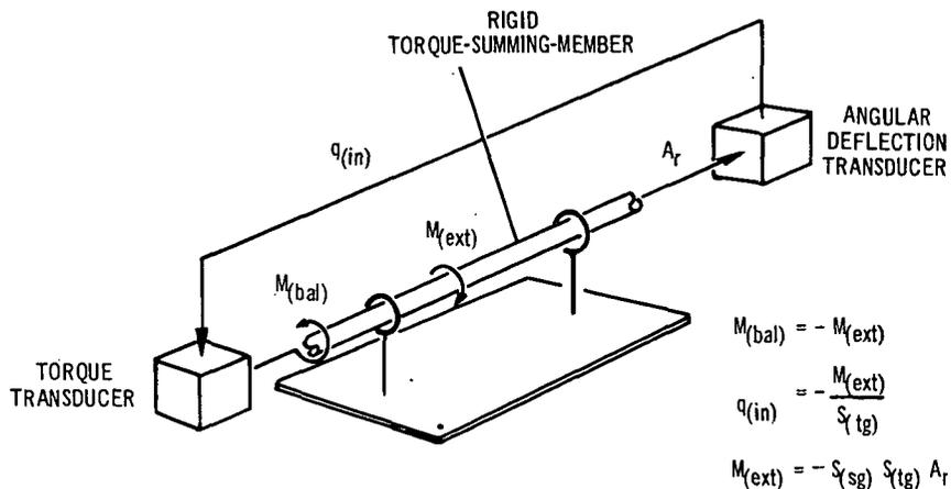
Fig. 1-2. Schematic showing general torque measuring feedback loop.
