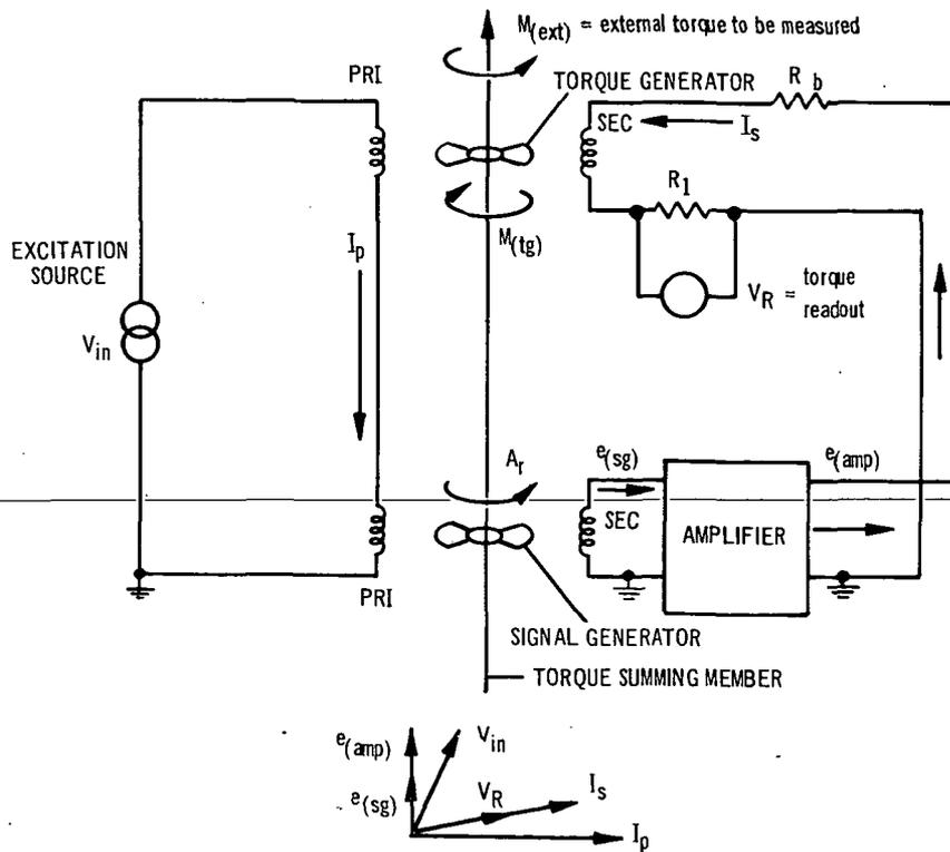
Fig. 2-1. Torque measuring by the constant elastance method, with RMS current readout.
