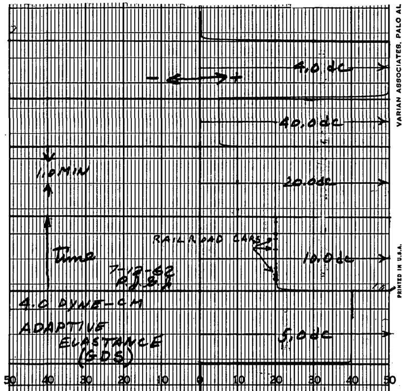
Fig. 9-5. A torque of 4.0 dyne-centimeters on five different torque scales.
