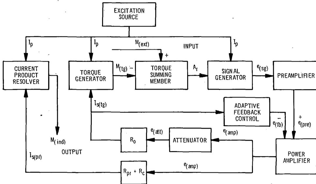
Fig. 5-4. Negative current feedback for adaptive elastance system.
