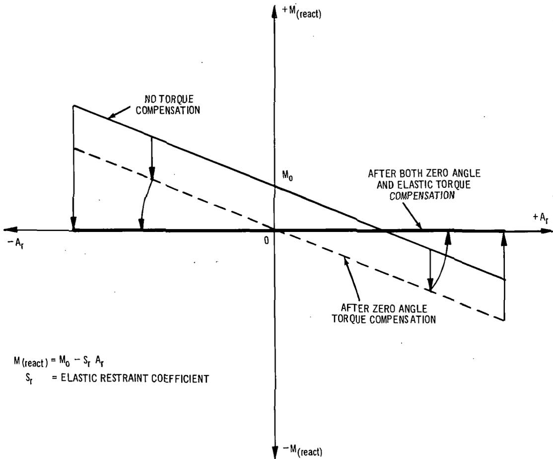
Fig. 6-2. Microsyn reaction torque and its compensation.
