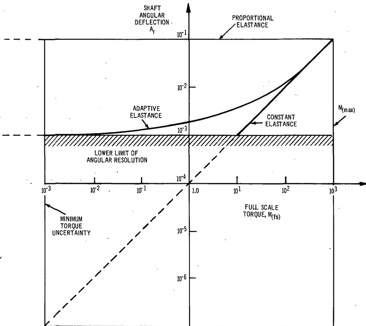
Fig. 5-6. Torque-angular deflection for various types of elastance.
