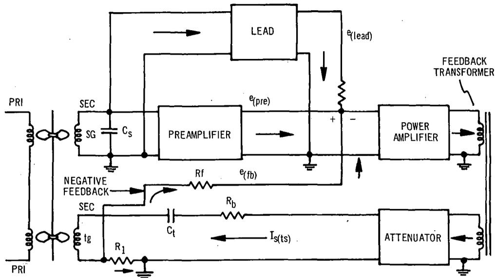
Fig. 5-3. Negative current feedback for adaptive elastance control.
