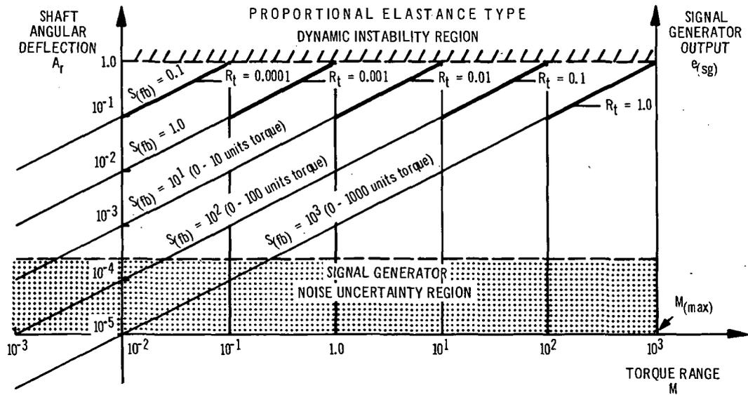
Fig. 4-5. Constant vs. proportional elastance torque systems.
