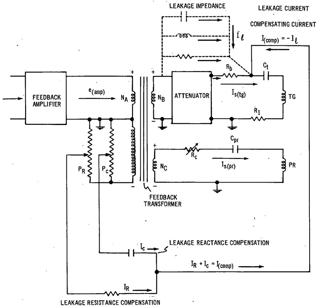
Fig. 6-6. Torque generator secondary leakage impedance compensator.
