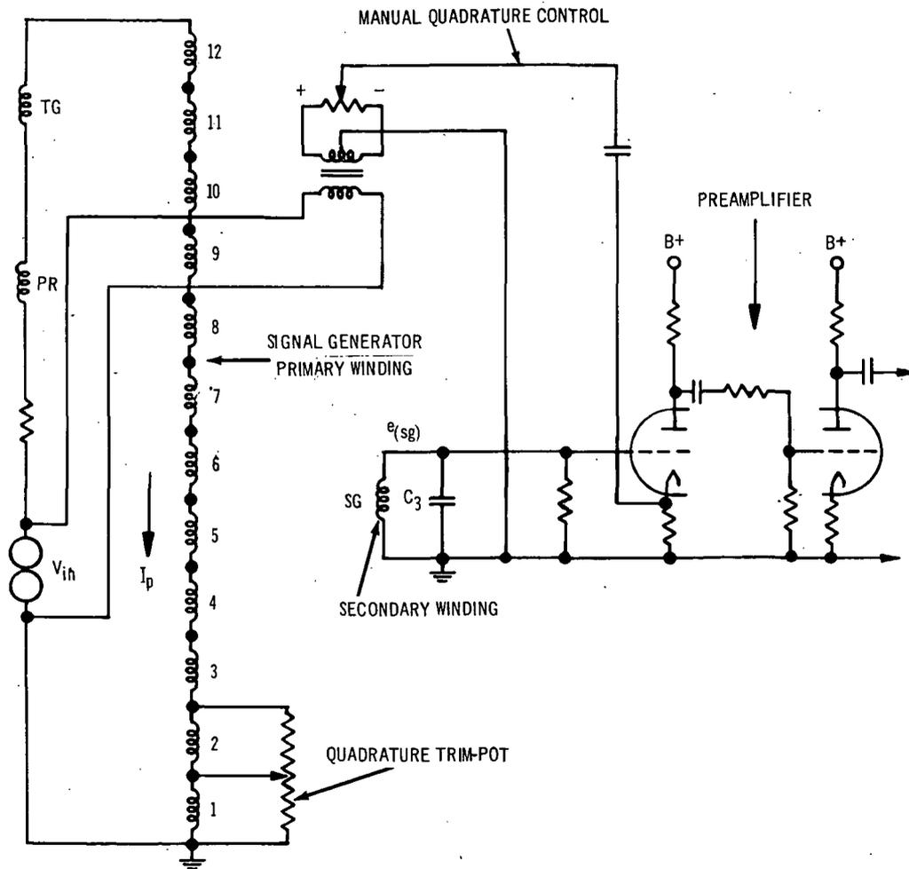
Fig. 6-4. Quadrature voltage compensation in a 12-pole microsyn.
