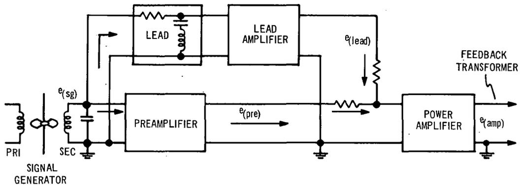
Fig. 4-6. A method for obtaining rate stabilization in an a-c system.
