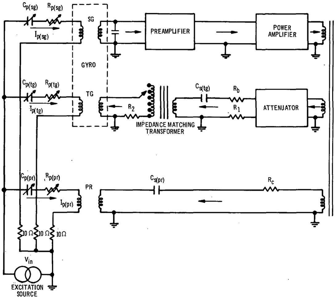
Fig. 8-2. Parallel excitation of gyro microsyns and current product resolver.
