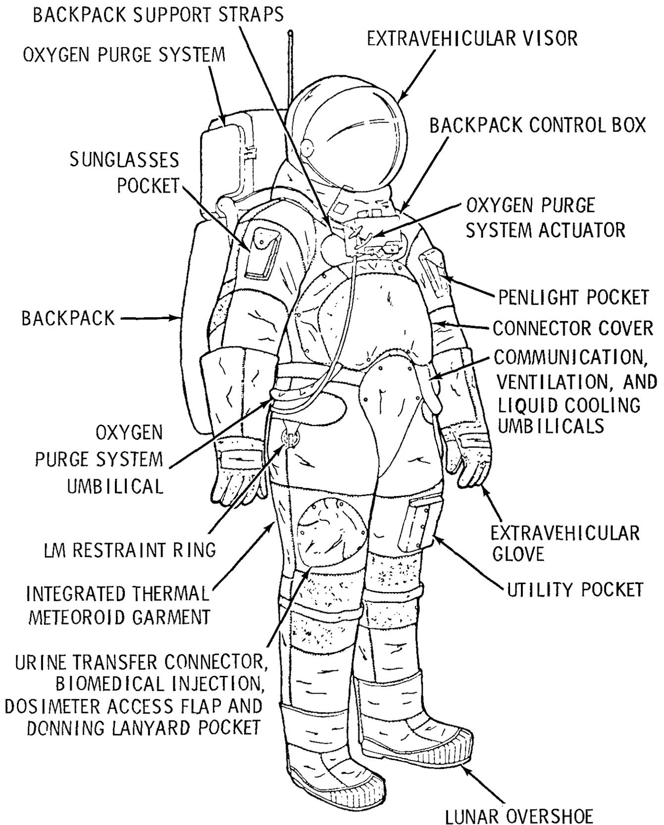
Extravehicular visor assembly--A polycarbonate shell and two visors with thermal control and optical coatings on them. The EVA visor is attached over the pressure helmet to provide impact, micrometeoroid, thermal and light protection to the EVA crewman.
