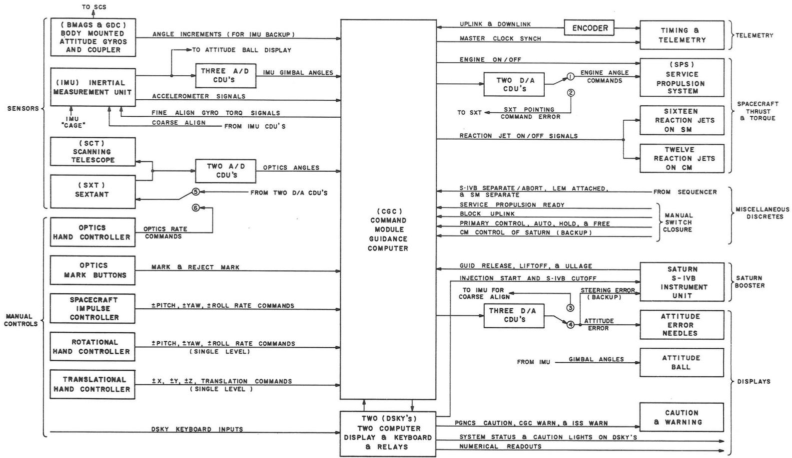
Fig. 3.1 Block II G&N and Block II CSM Functional Interface Diagram
