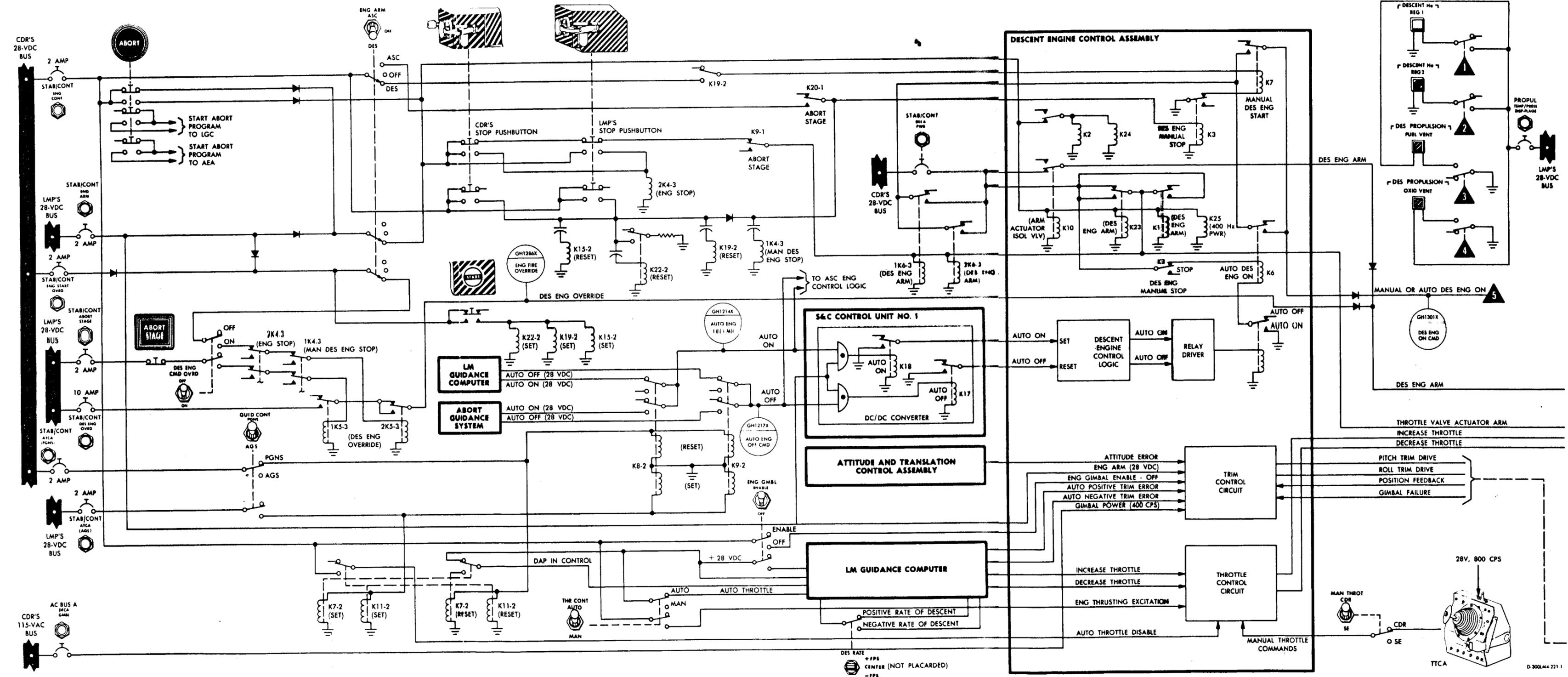
Figure 2.1-18. Descent Engine Control Schematic (Sheet 1 of 2)
