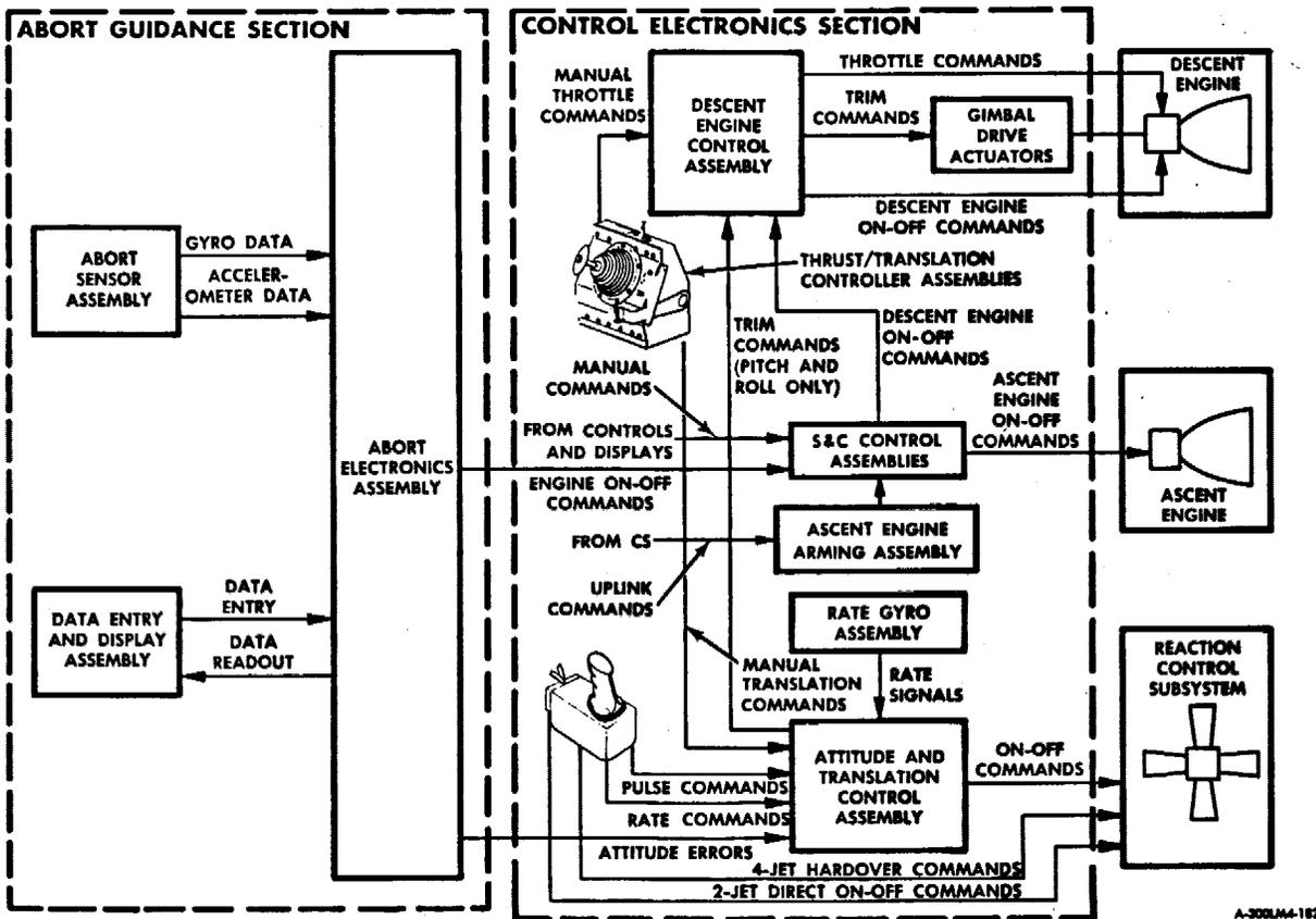
Figure 2.1-14. Abort Guidance Path - Simplified Block Diagram
