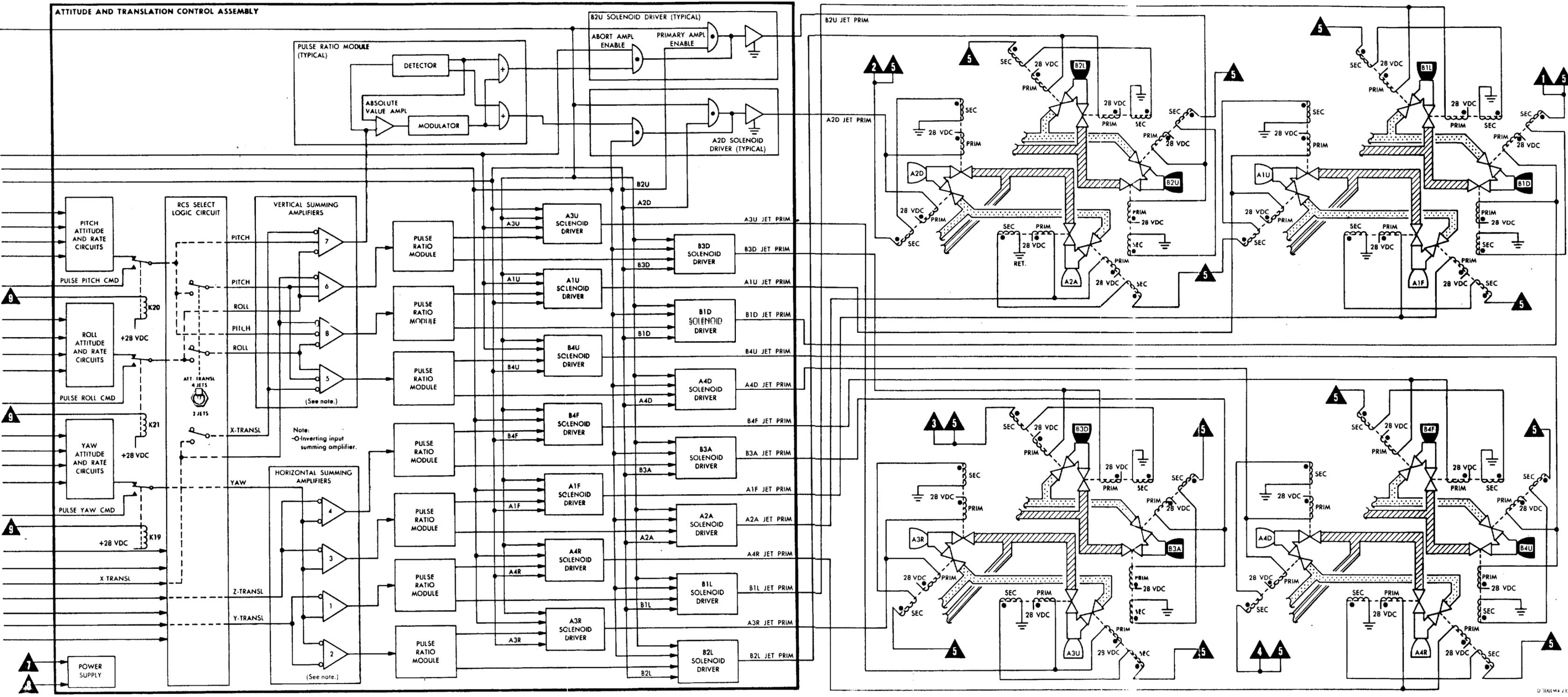
Figure 2.1-17. Attitude and Translation Control Schematic (Sheet 2 of 2)
