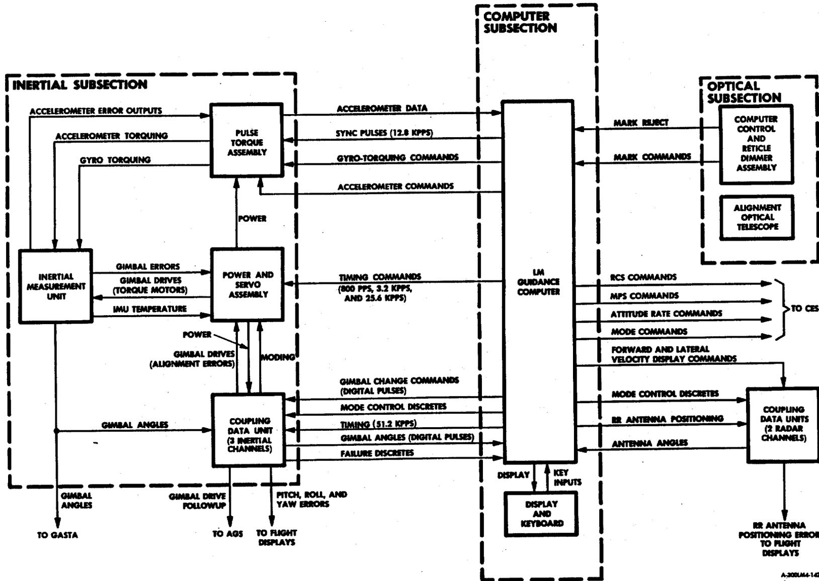
Figure 2.1-3. Primary Guidance and Navigation Section - Block Diagram
