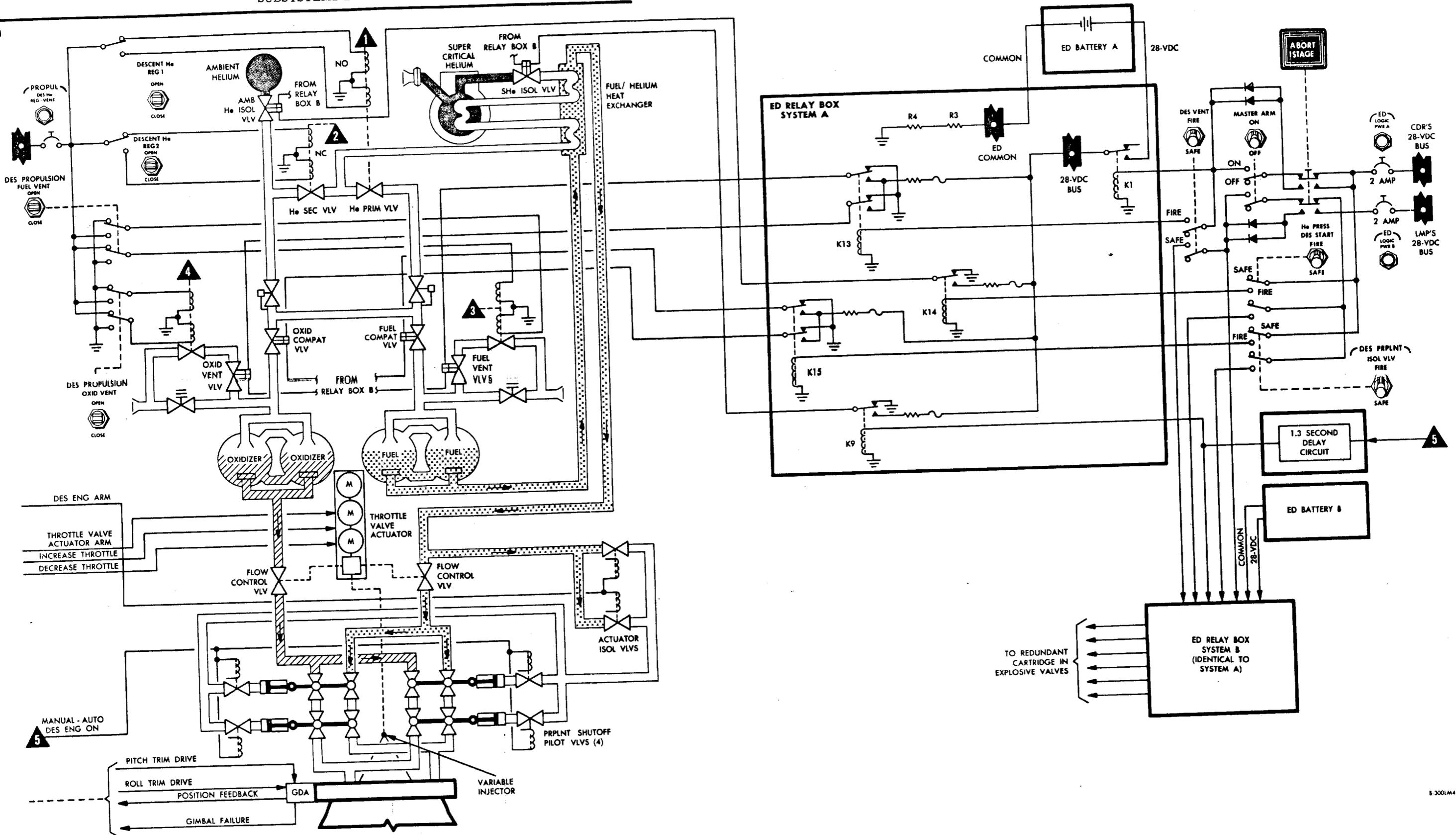
Figure 2.1-18. Descent Engine Control Schematic (Sheet 2 of 2)
