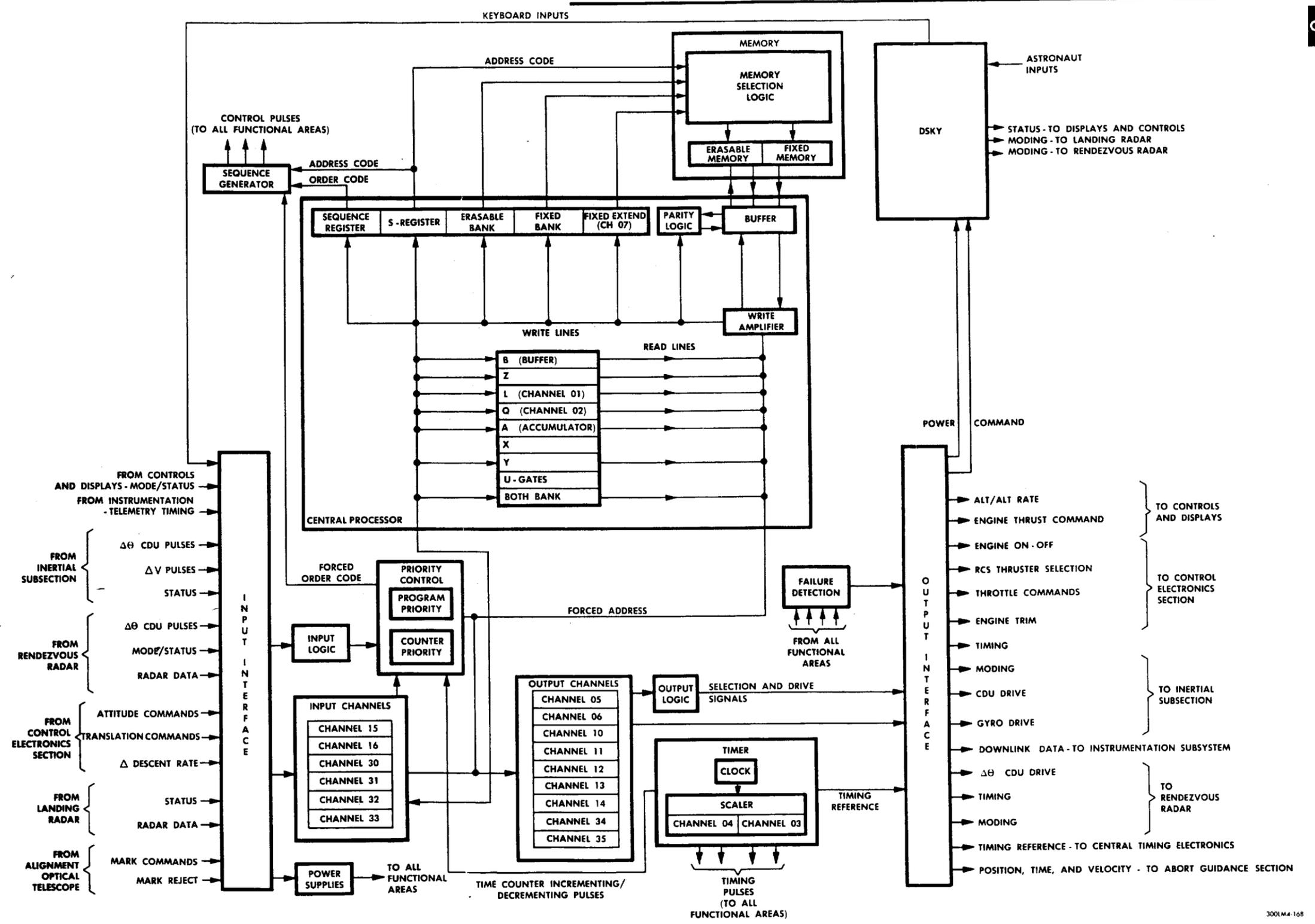
Figure 2.2-51. LM Guidance Computer - Functional Flow Diagram
