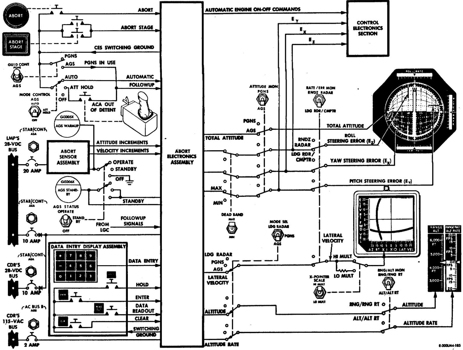
Figure 2.1-16. Abort Guidance Section - Functional Flow Diagram
