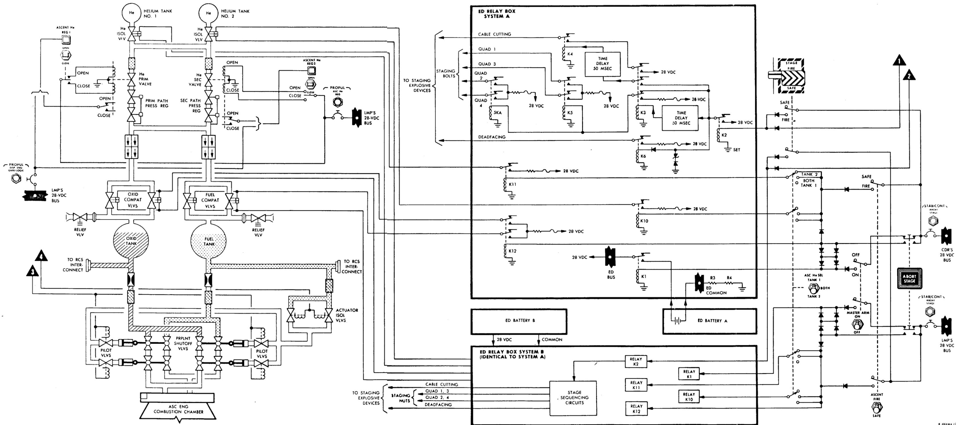
Figure 2.1-19. Ascent Engine Control Schematic (Sheet 2 of 2)
