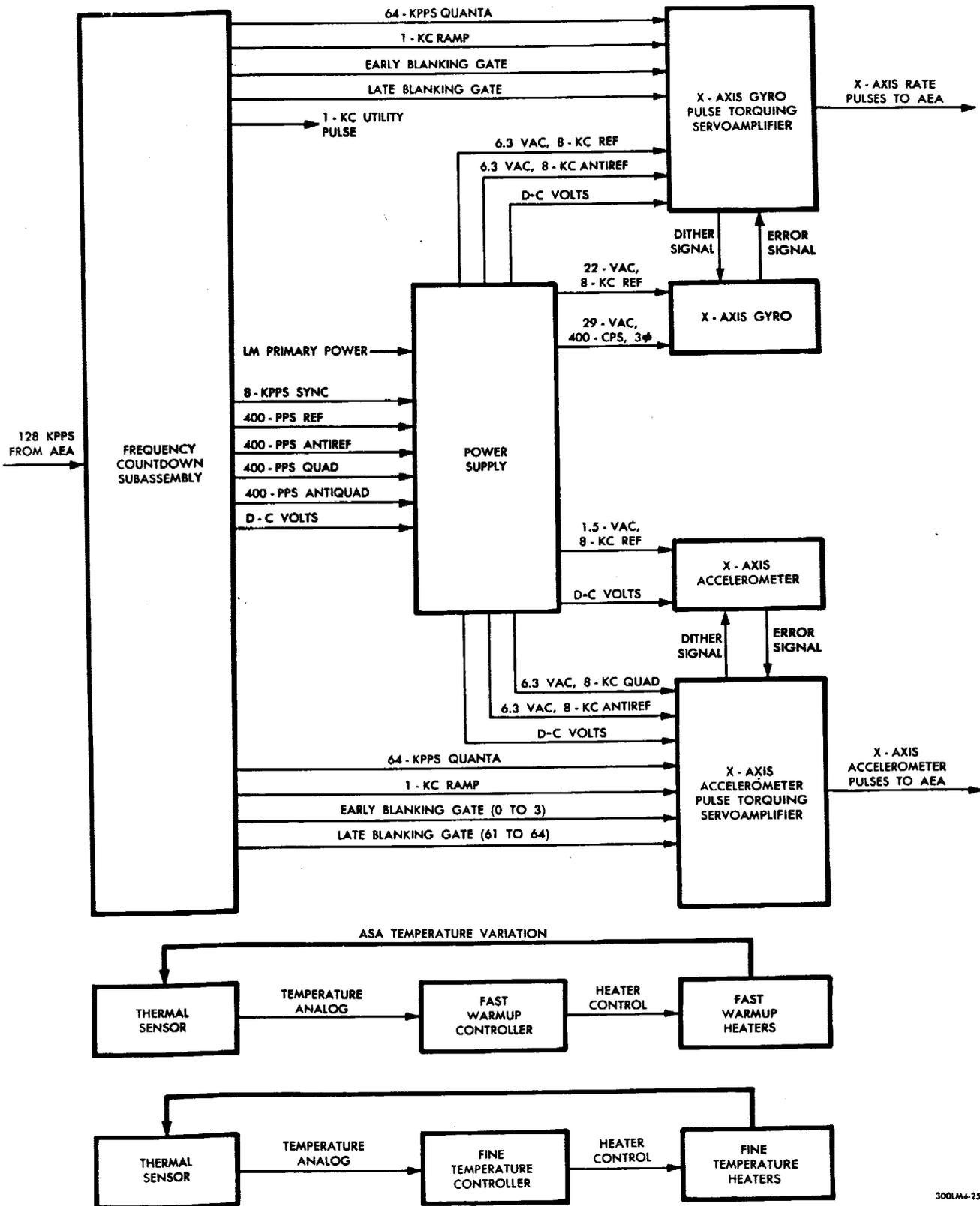
Figure 2.1-34. Abort Sensor Assembly - Block Diagram
