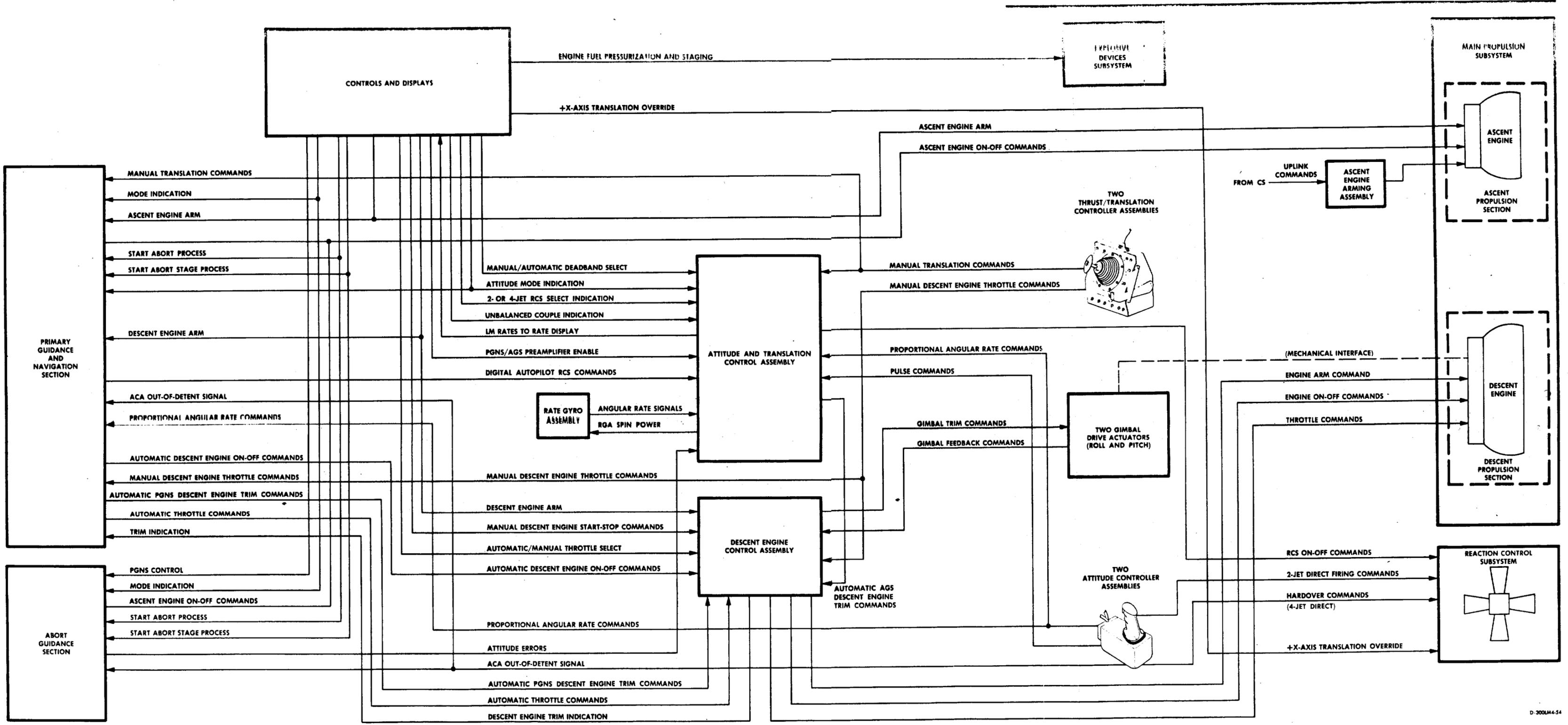
Figure 2.1-8. Control Electronics Section - Block Diagram
