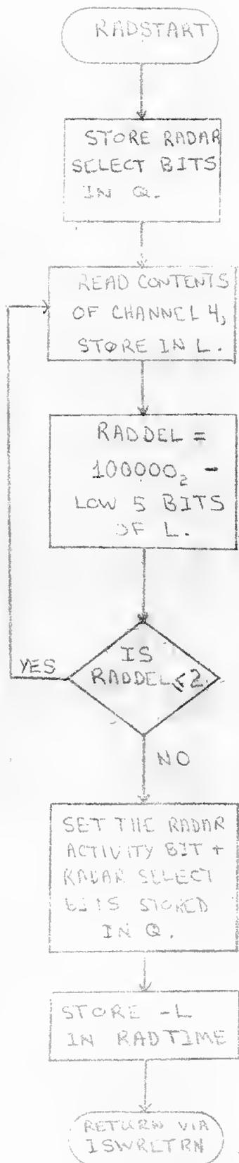
Inputs are the radar select bits in A and bits 1-4 of channel 13 zeroed.
