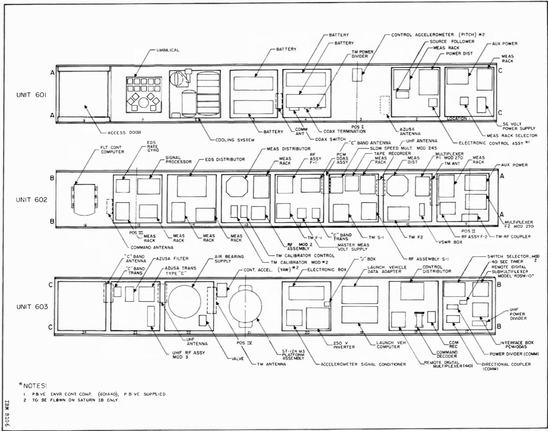
Figure 12.1-2 Saturn IB Instrument Unit Equipment Layout, R & D
