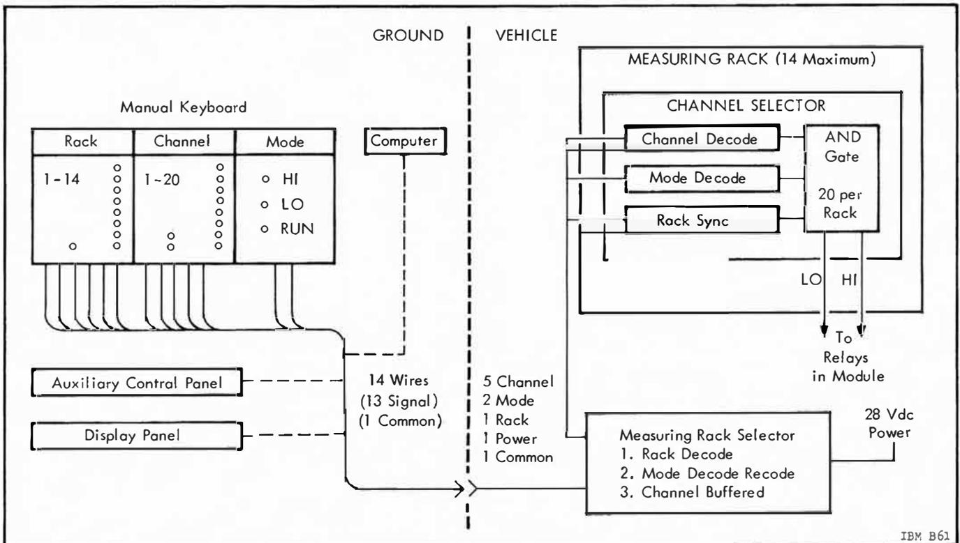
Figure 5.3-1 Block Diagram of RACS for the IU
