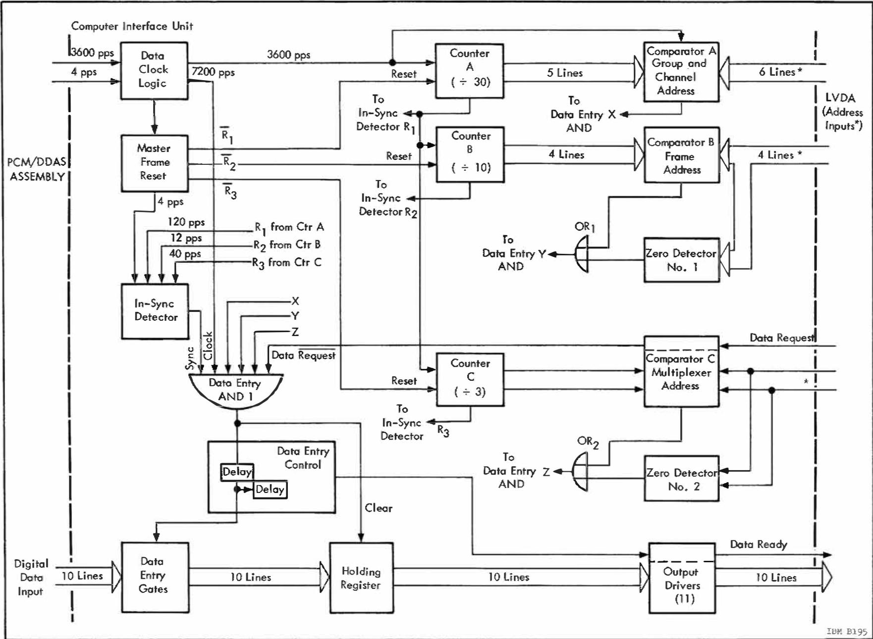
Figure 5.7-2 Computer Interface Unit Block Diagram
