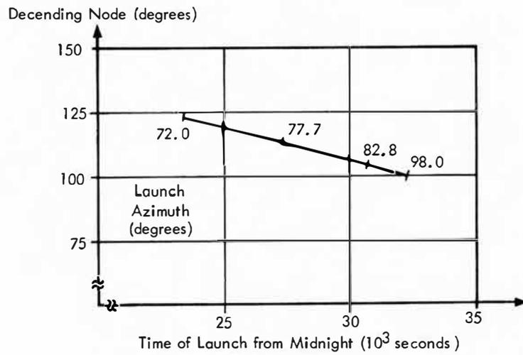
Time of Launch Versus Launch Azimuth
