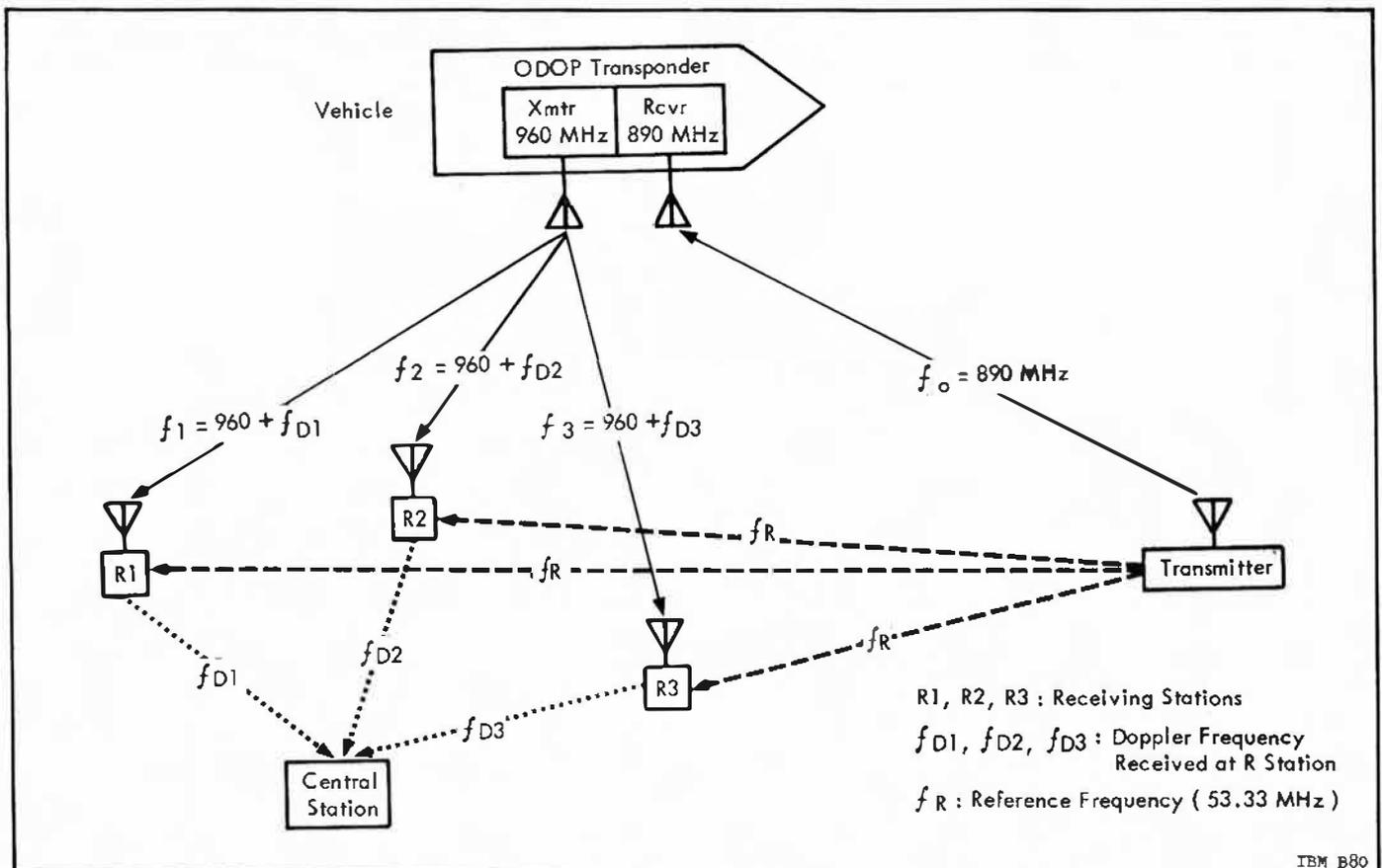
Figure 7.4-1 ODOP System Configuration
