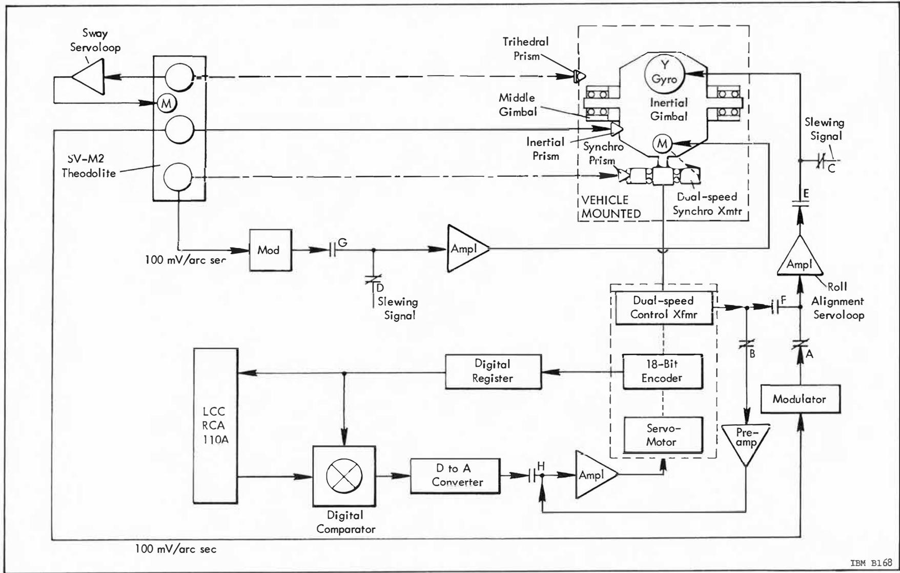
Figure 14.7-6 Azimuth Alignment Scheme
