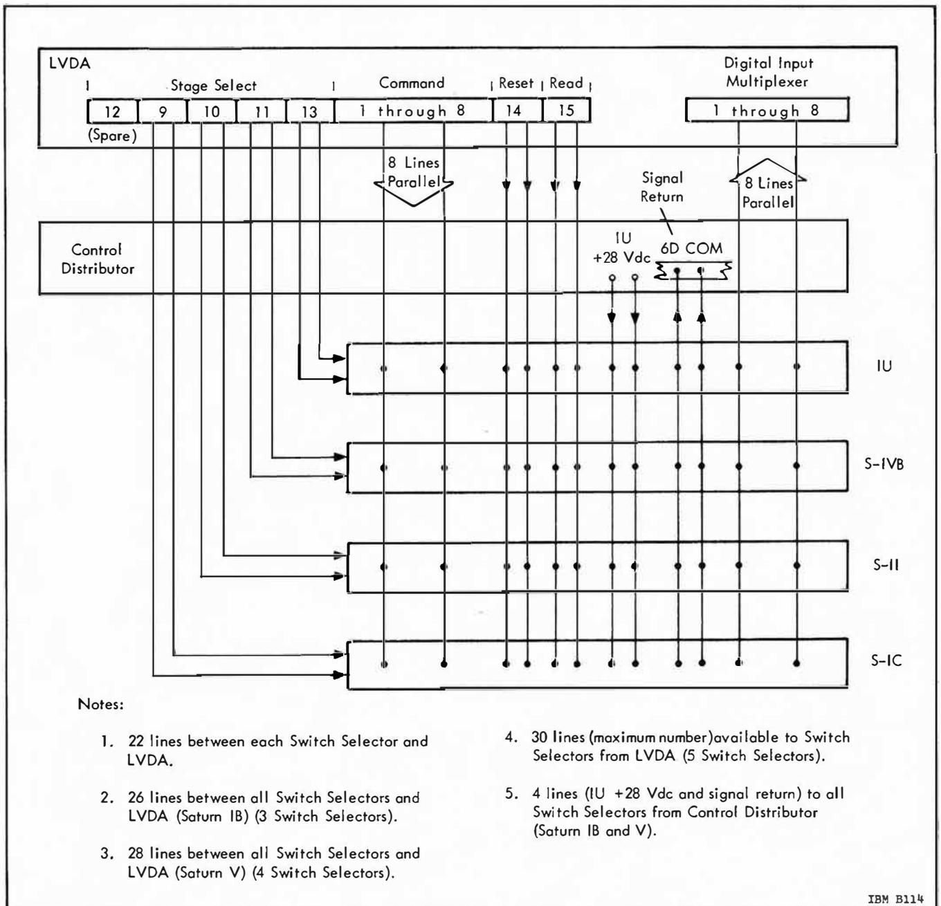
Figure 4.2-3 LVDC - Switch Selector Interconnection Diagram
