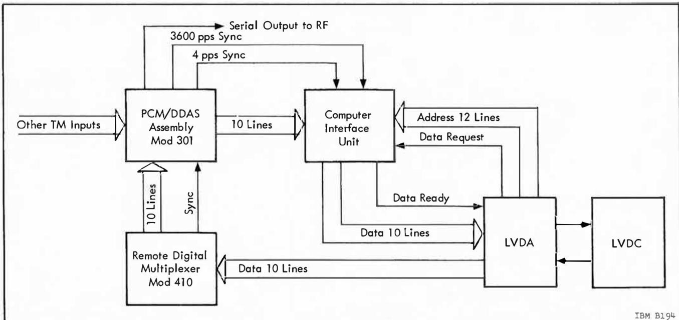
Figure 5.7-1 Computer Interface Unit - System Interconnection Diagram
