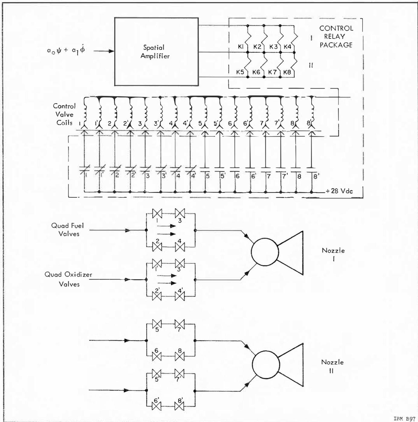
Figure 3.2-8 Relay Control Unit and Quad Redundant Valves
