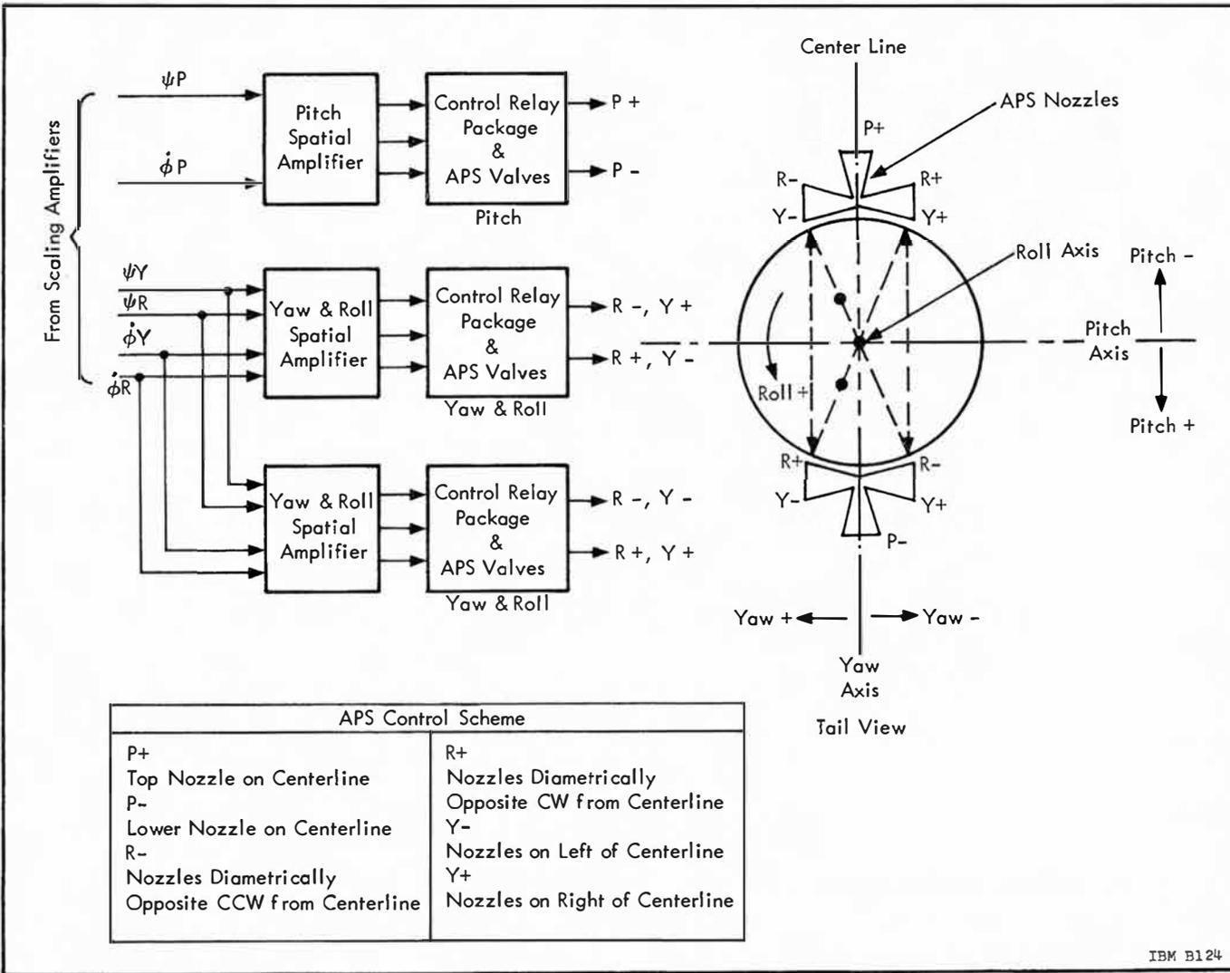
Figure 3.4-7 Connection of Control Signals to Spatial Amplifiers
