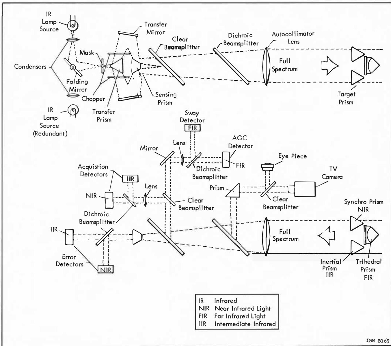
Figure 14.7-3 Optical Schematic Diagram of SV-M2 Theodolite
