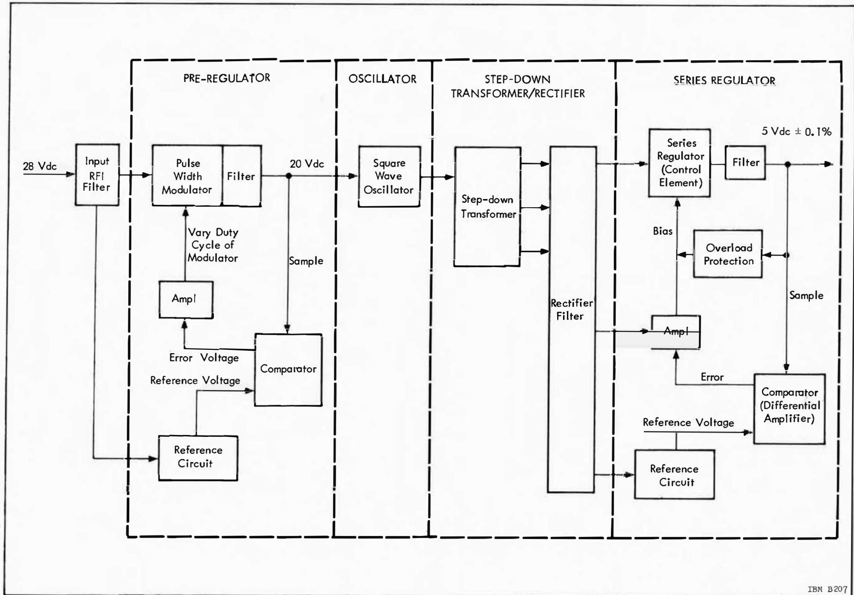
Figure 8.5-1 5 Volt Measuring Voltage Supply Block Diagram
