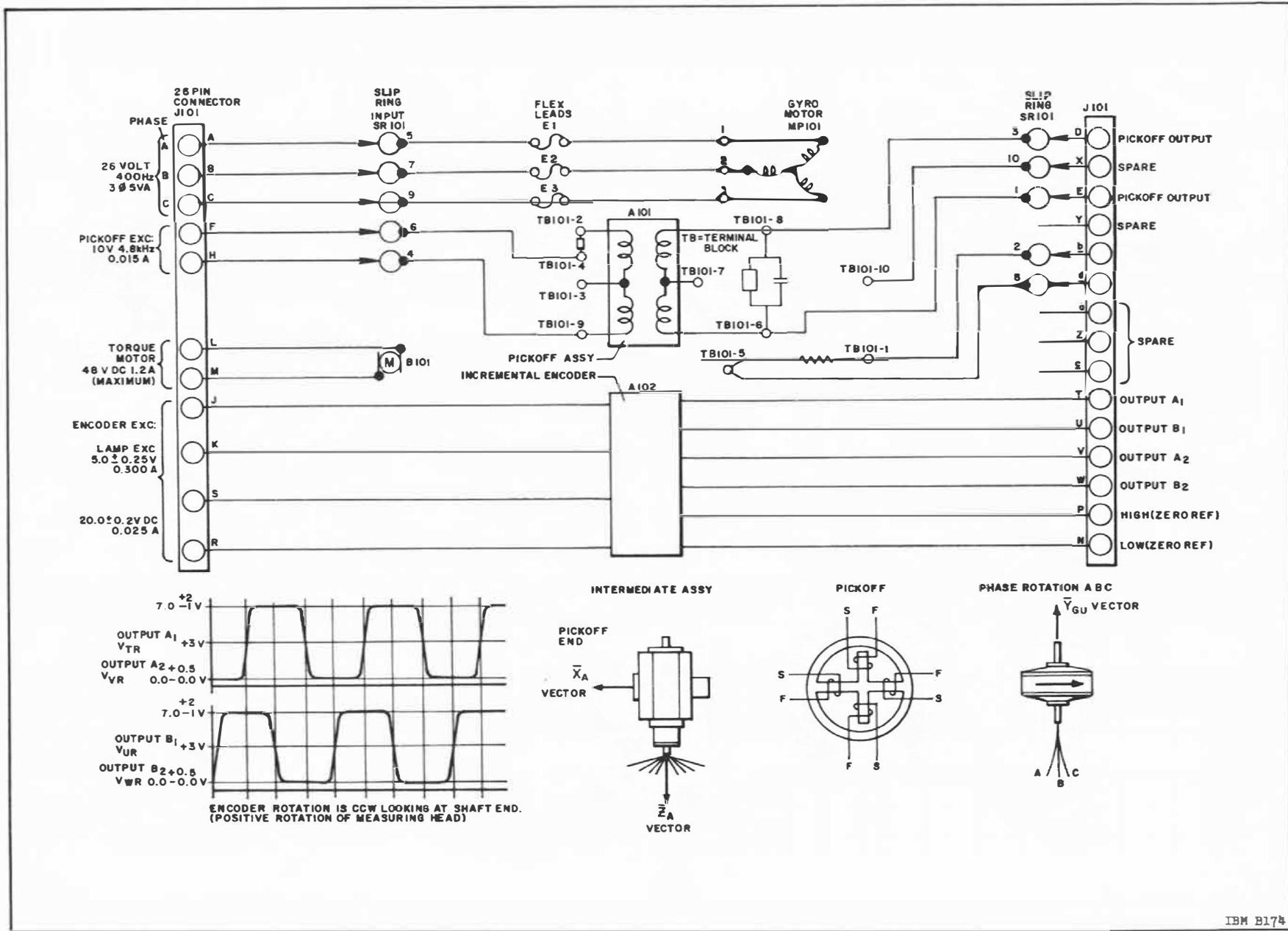
Figure 14.9-3 Electrical Schematic of an AB3-K8 Accelerometer
