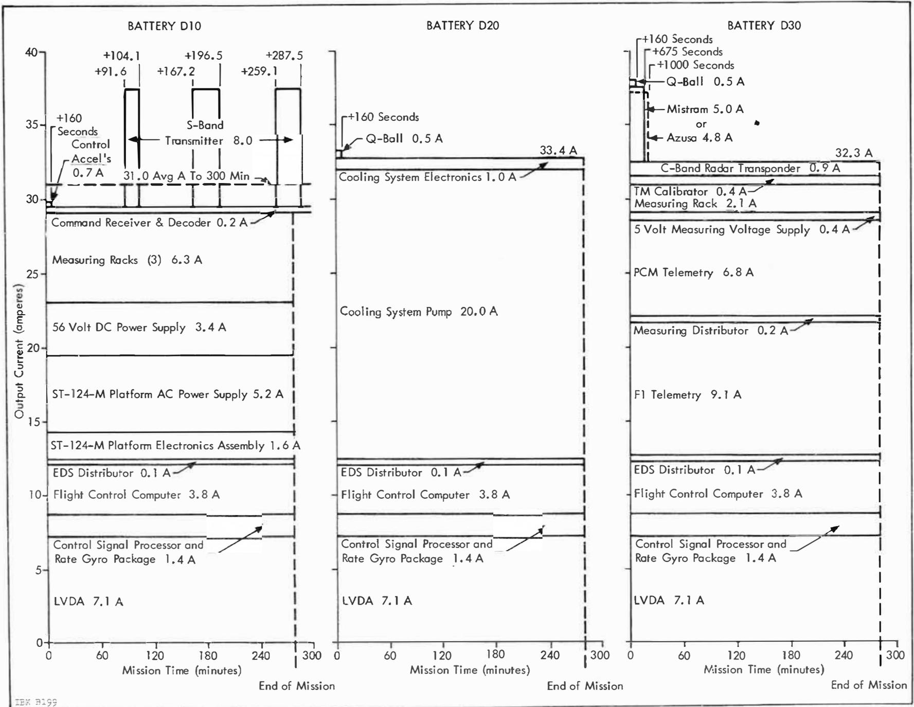
Figure 8.2-2 Battery Load Profiles for SA-IU-205 and Subsequent Vehicles
