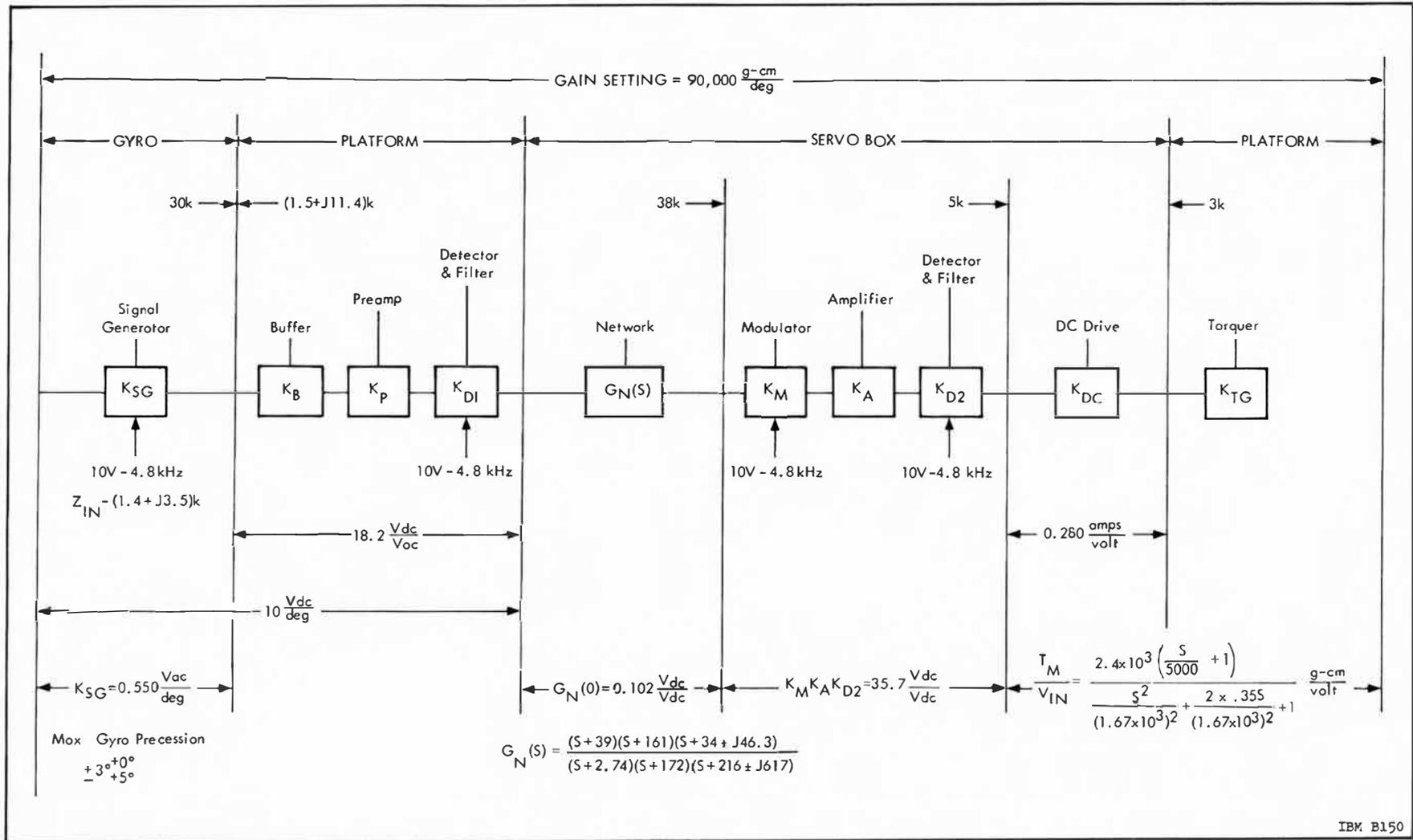
Figure 14.3-4 Gimbal Electronics Block Diagram
