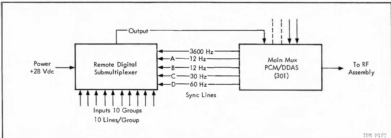
Figure 5. 5-3 Block Diagram of RDSM Inputs and Outputs
