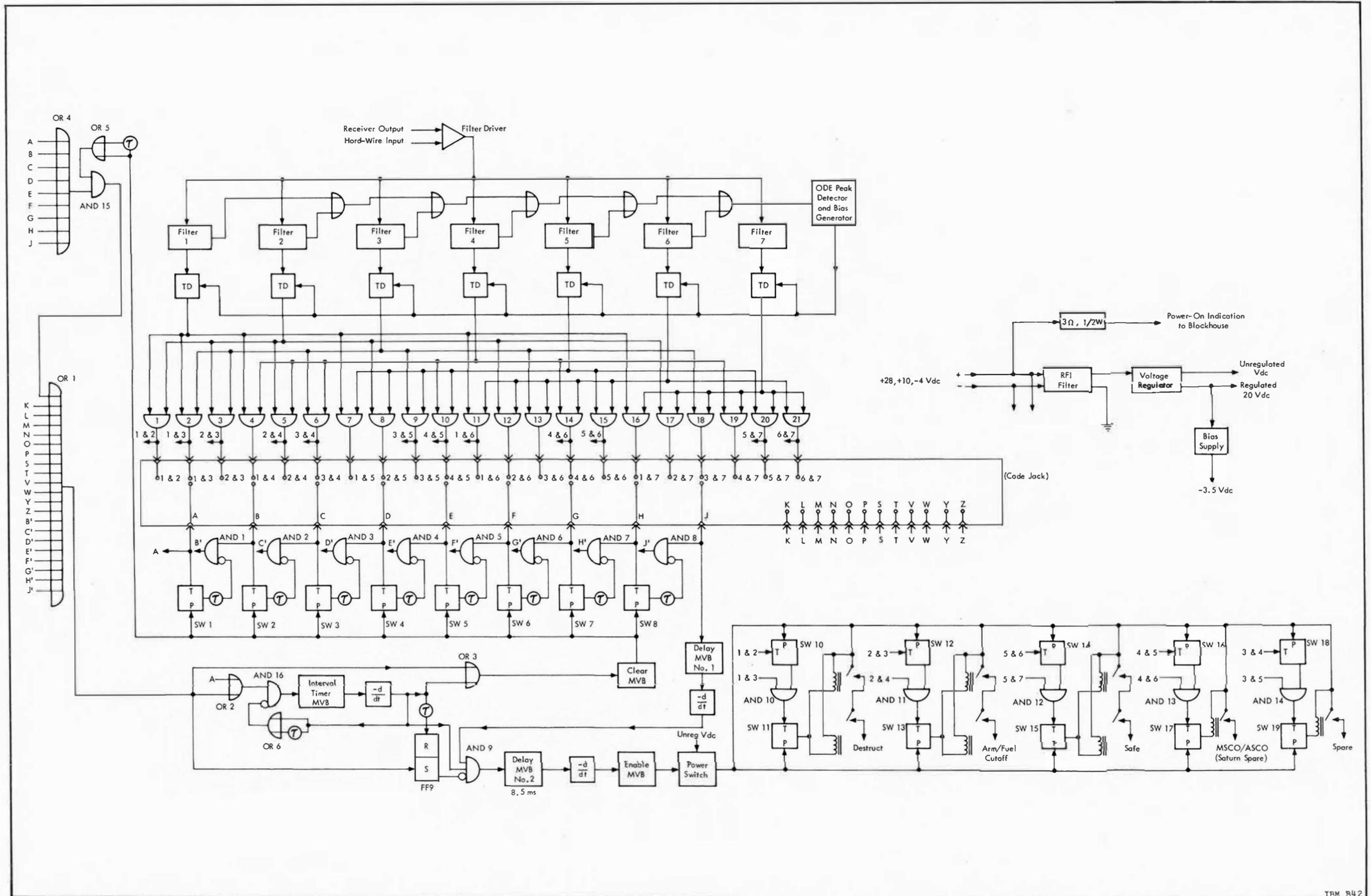
Figure 6.3-5 Secure Range Safety Decoder Simplified Logic Diagram
