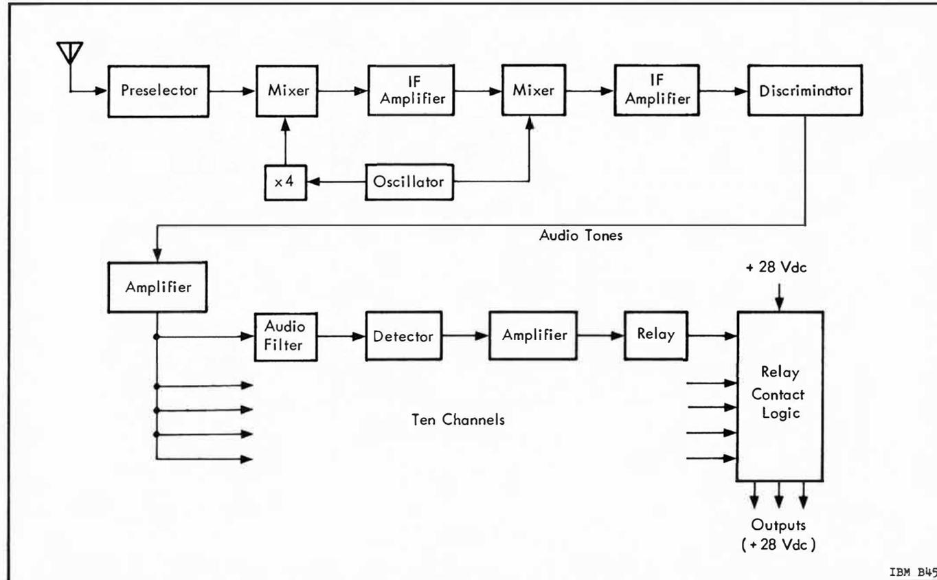
Figure 6. 5-3 AN/DRW-13 Receiver/Decoder
