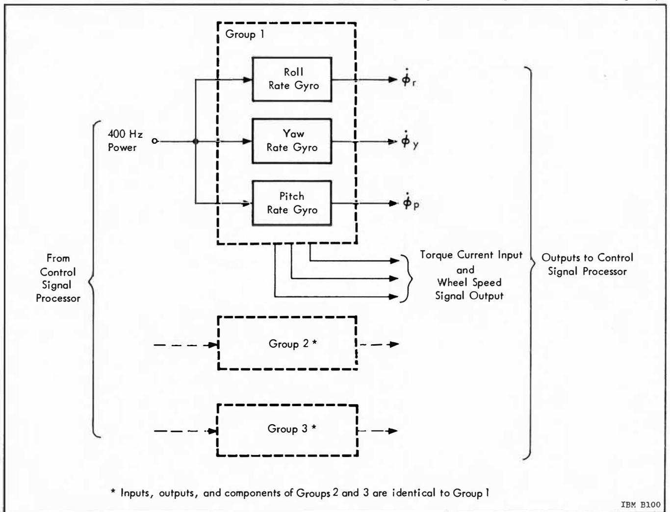
Figure 3.3-3 Control - EDS Rate Gyro Block Diagram
