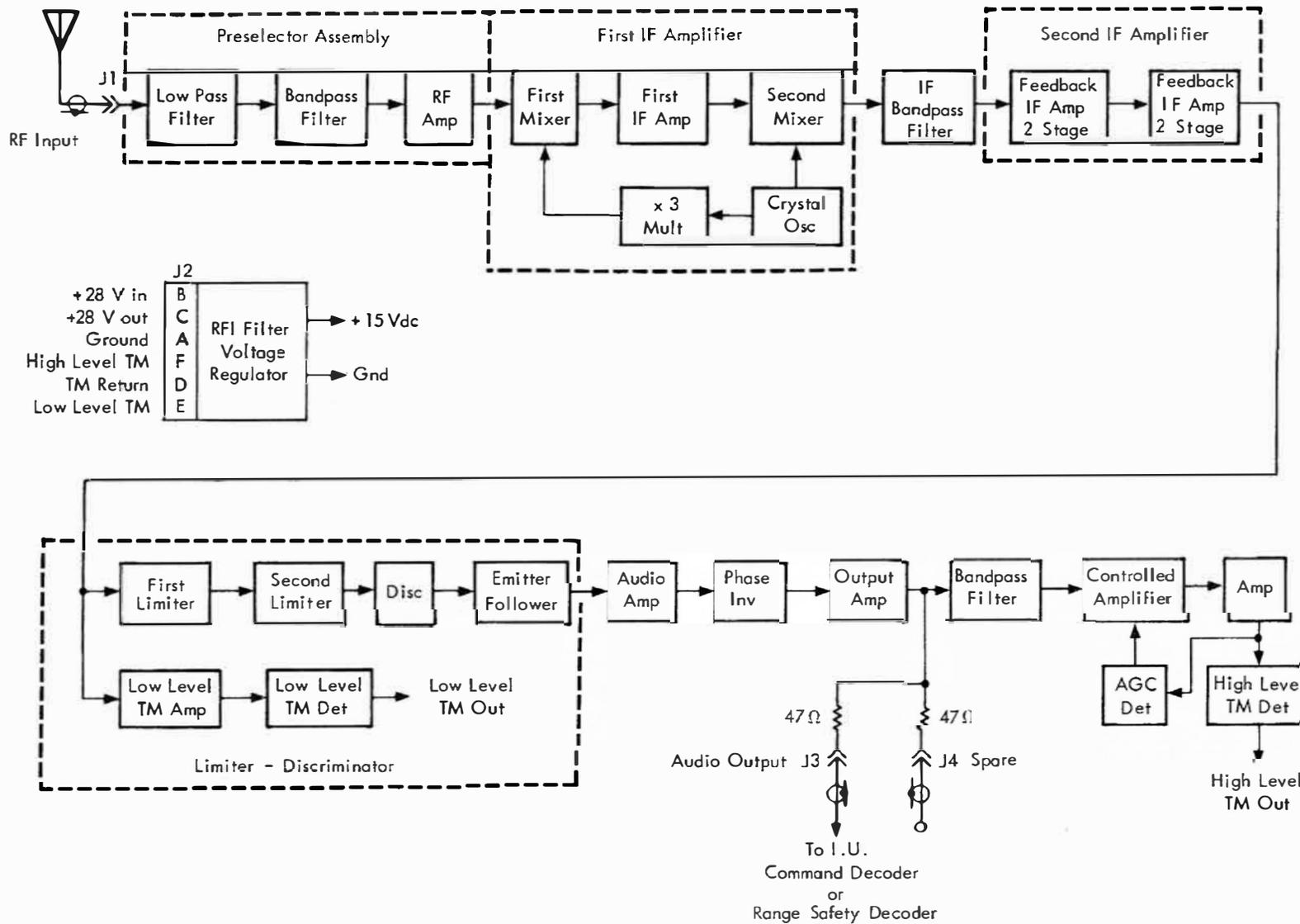
Figure 6.2-8 MCR-503 Command Receiver
