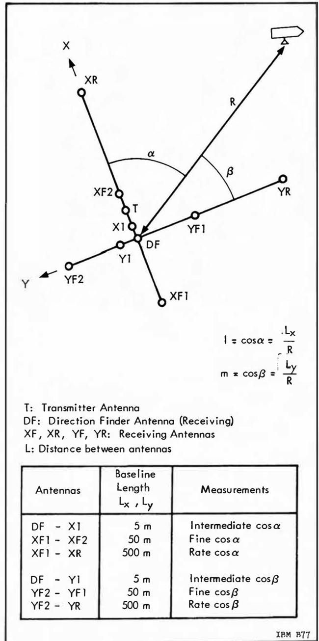
Figure 7.3-1 AZUSA (MK II) Ground Station Layout
