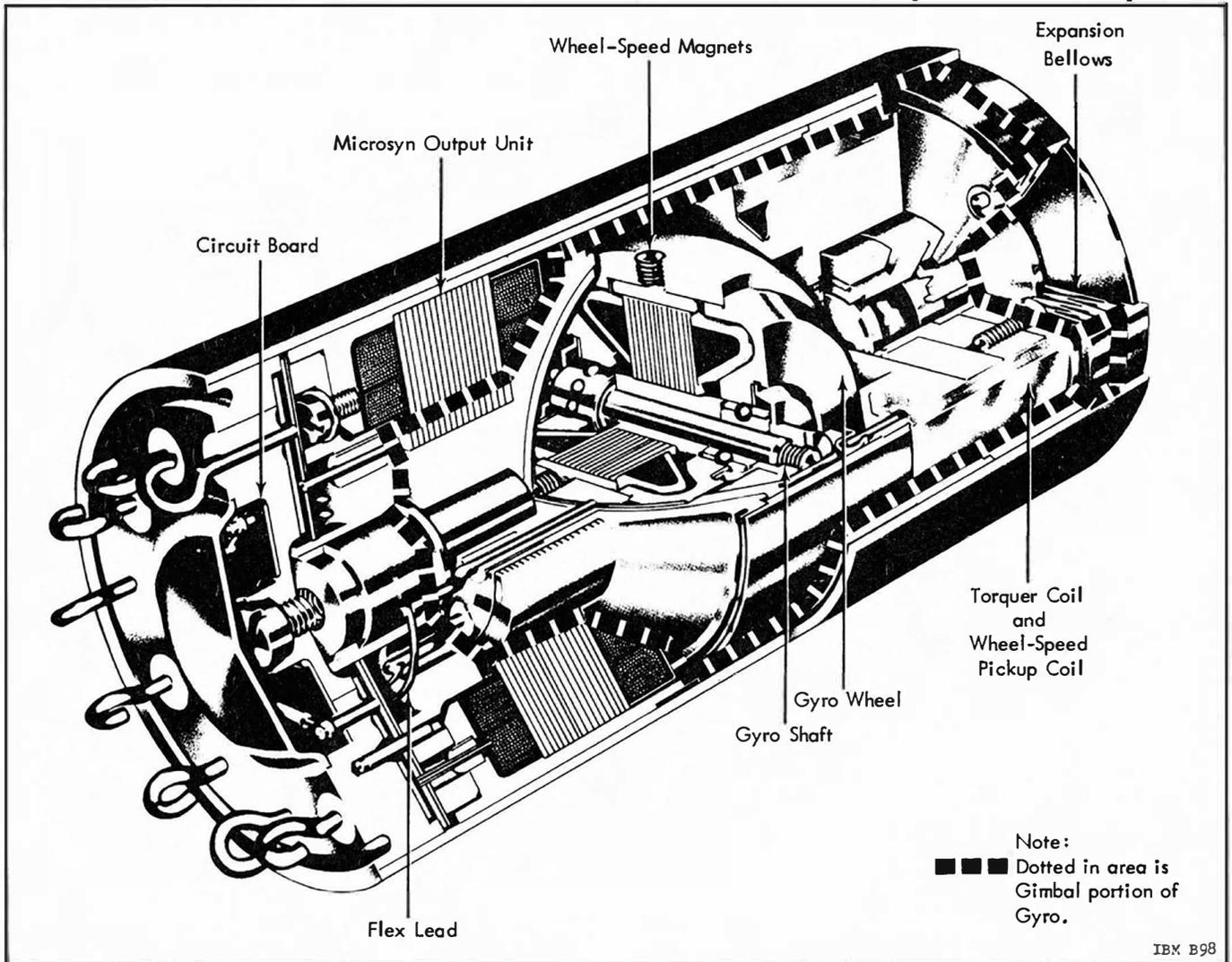
Figure 3.3-1 Cutaway View of a Self-Test Rate Gyro
