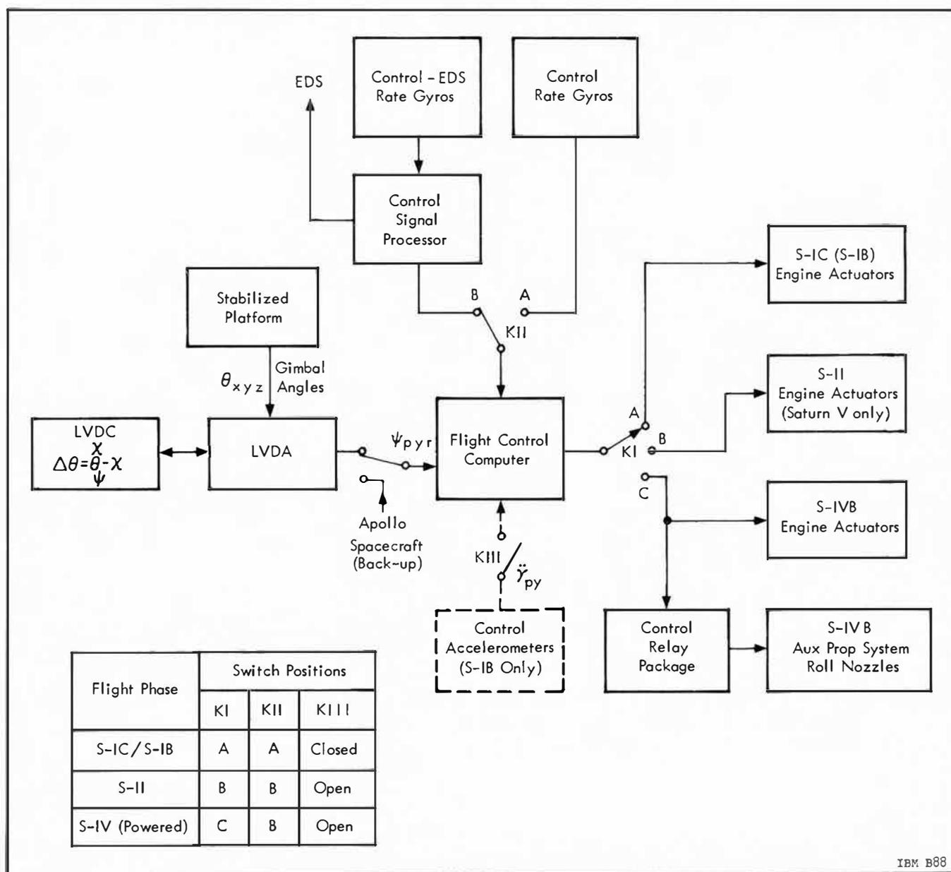
Figure 3.1-7 Saturn Control System Block Diagram (Powered Flight)
