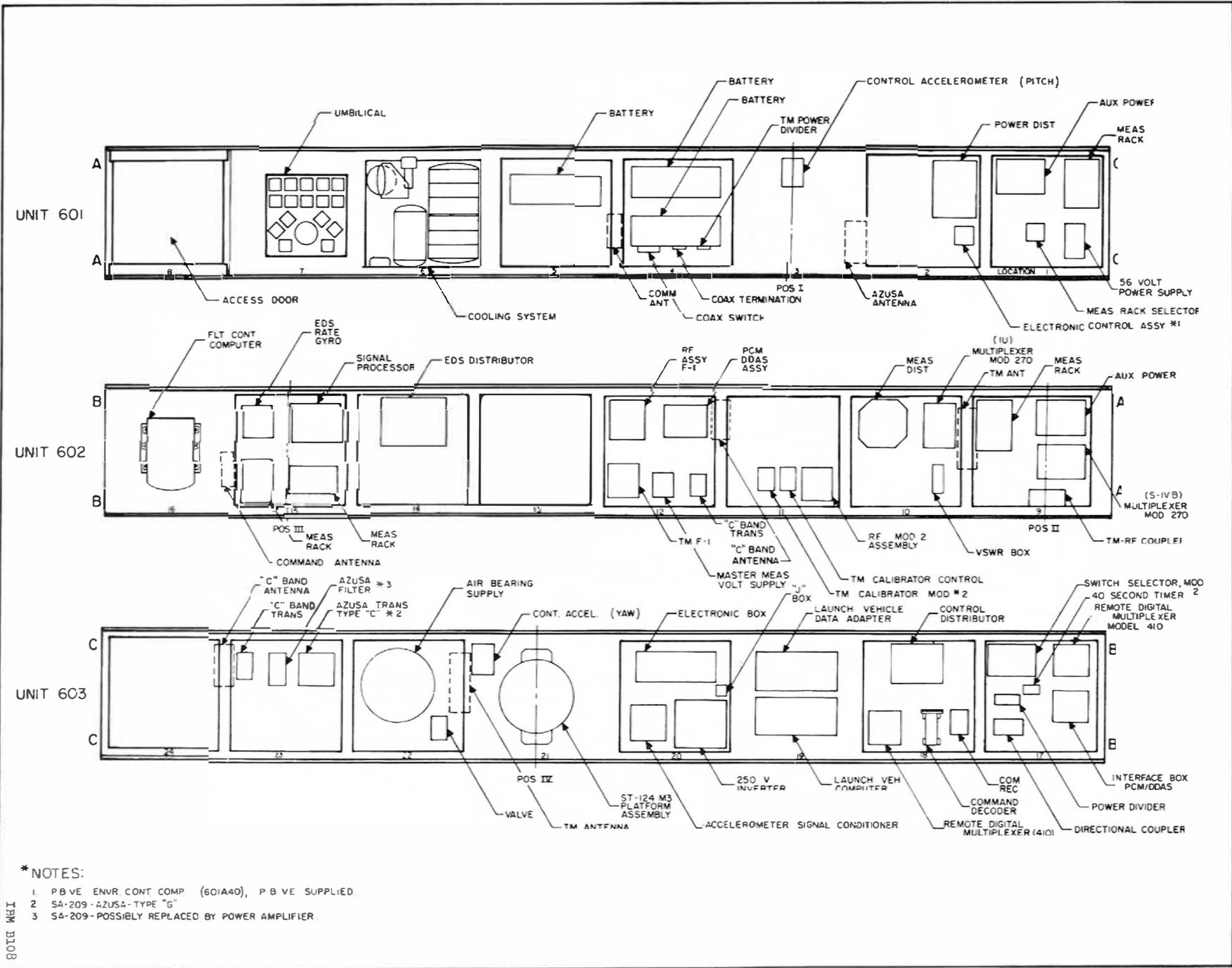
Figure 12. 1-4 Saturn IB Instrument Unit Equipment Layout, Operational
