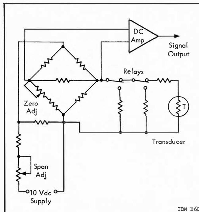
Figure 5.2-14 Typical Signal Conditioning Card for Temperature Measurements
