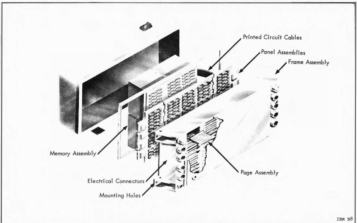
Figure 15.2-4 Exploded View of the Launch Vehicle Digital Computer
