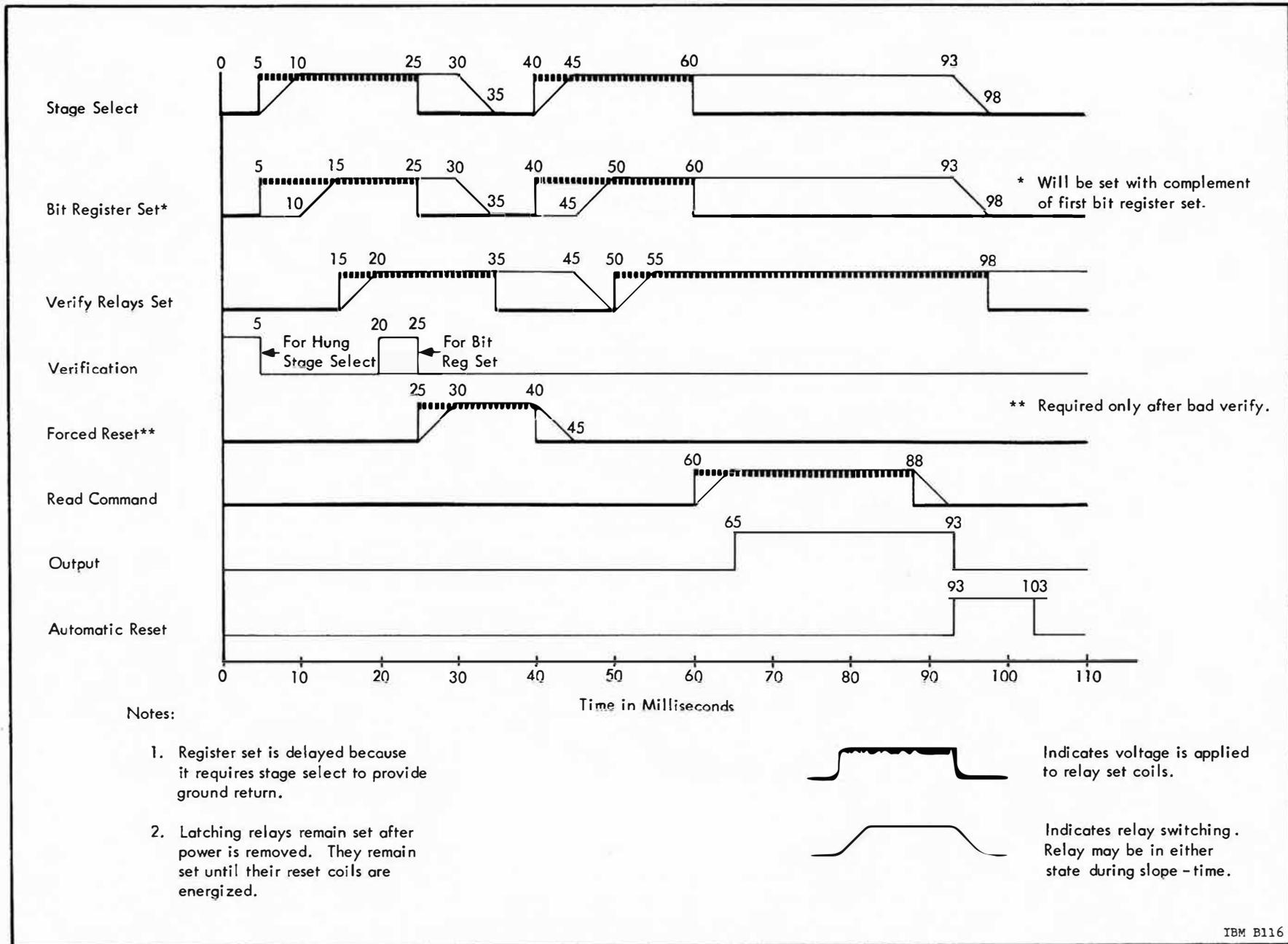
Figure 4.2-5 Switch Selector Timing Diagram
