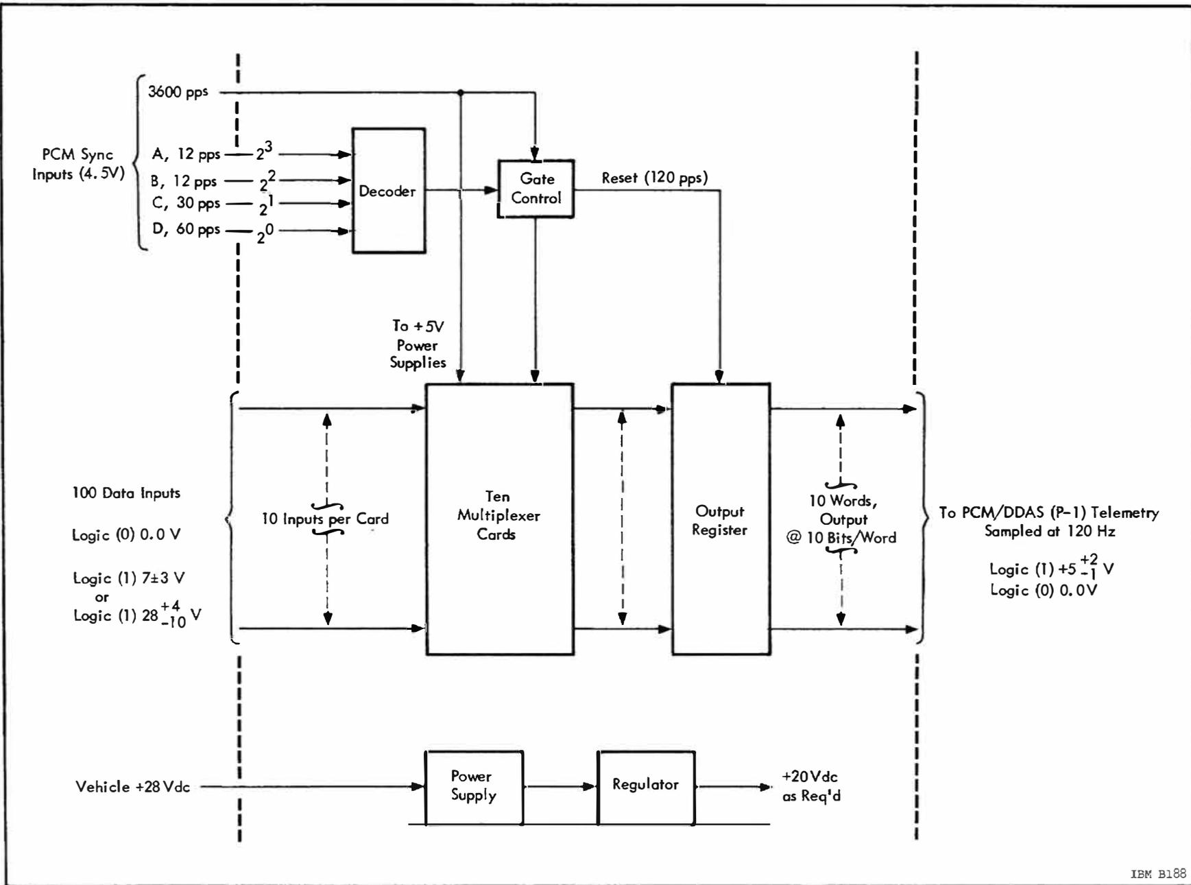
Figure 5.5-4 Remote Digital Submultiplexer Simplified Block Diagram
