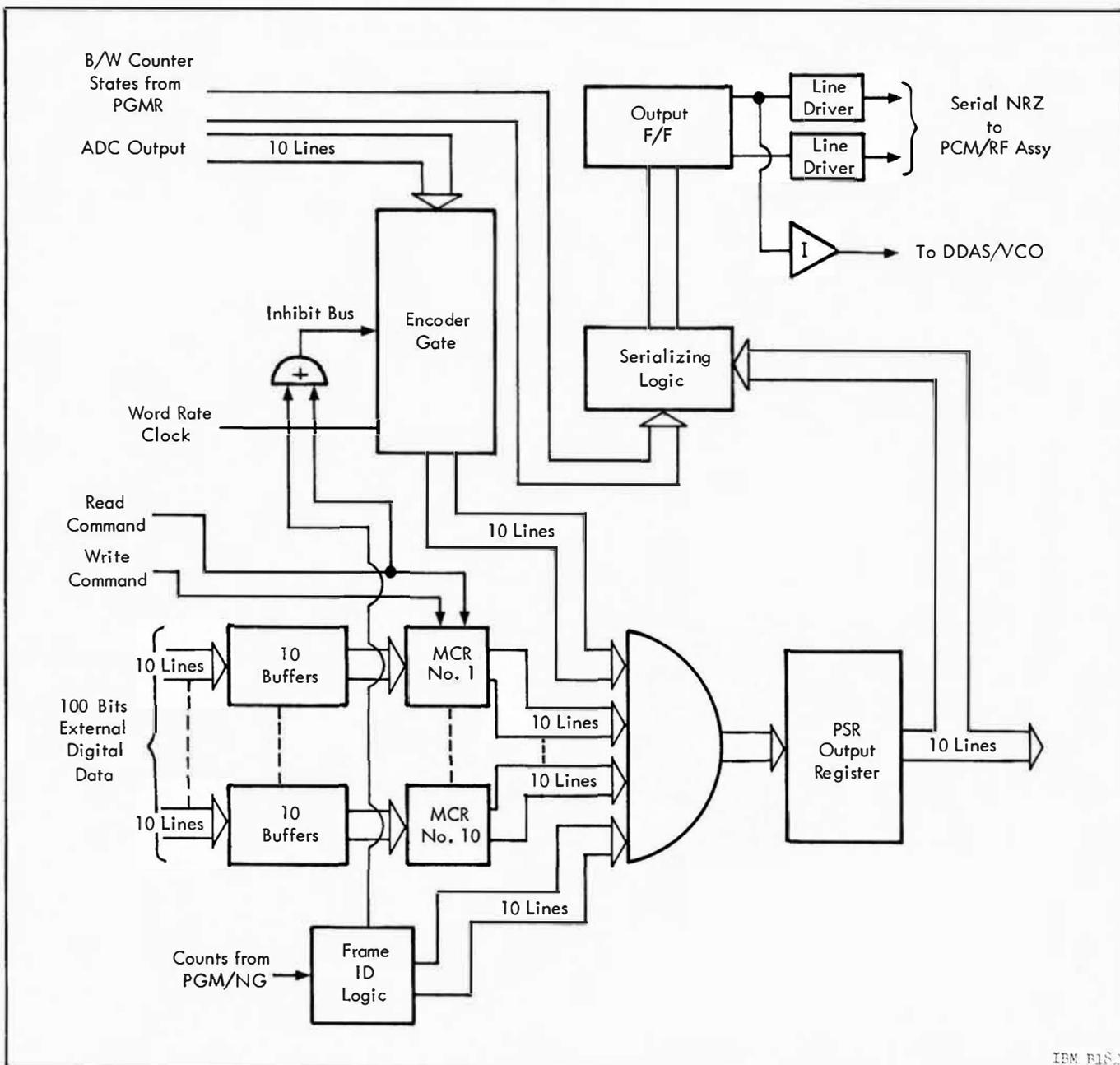
Figure 5.4-7 Digital Multiplexing and Formatting Logic
