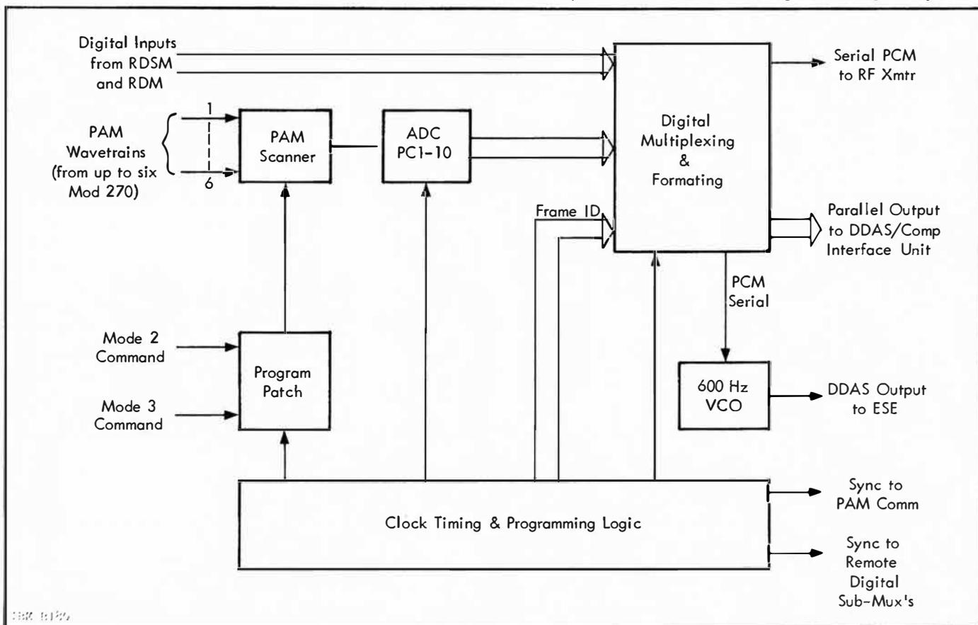
Figure 5.4-5 General Block Diagram - PCM/DDAS Assembly
