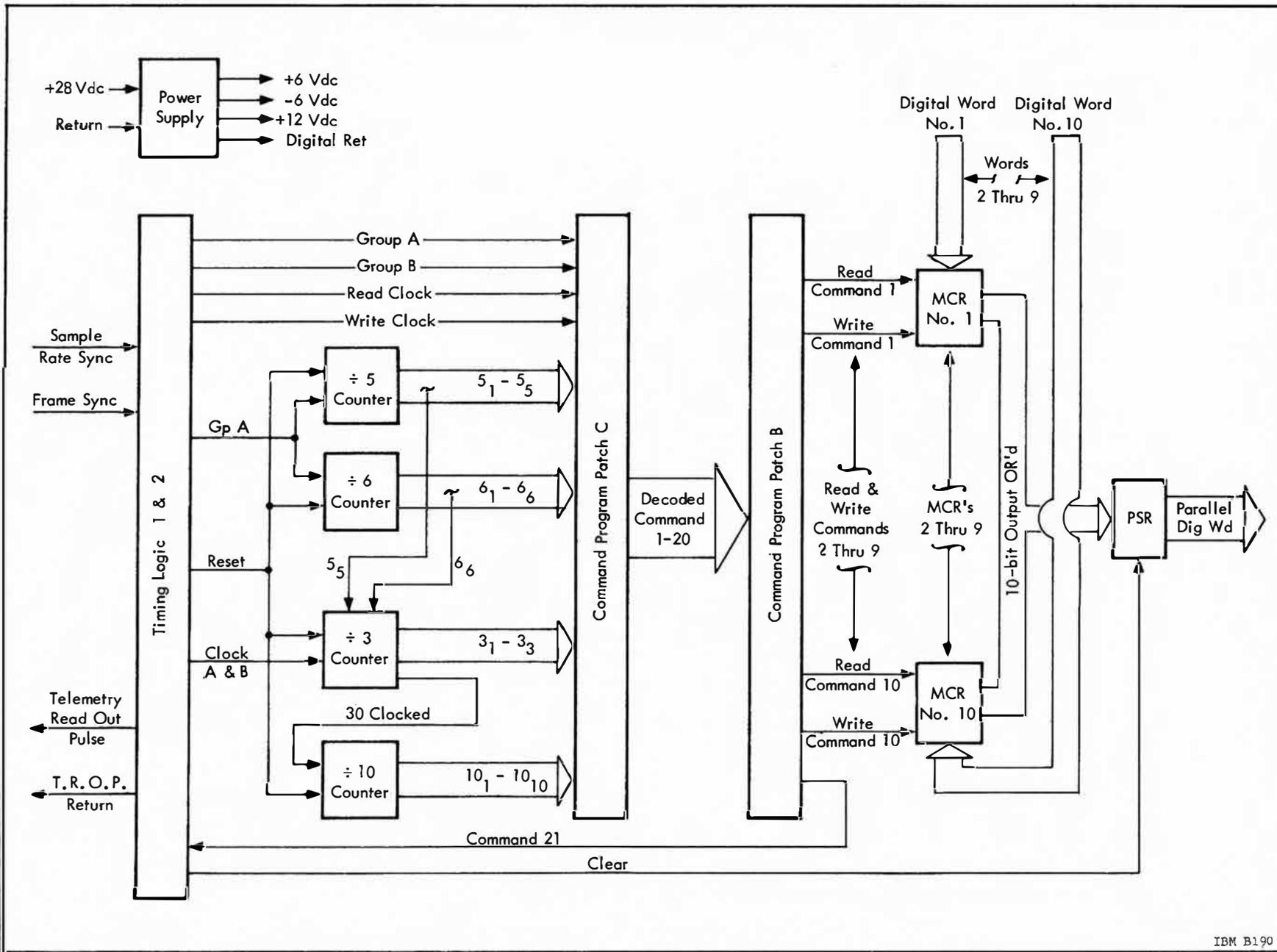
Figure 5. 5-6 Block Diagram of Mod 410 Multiplexer
