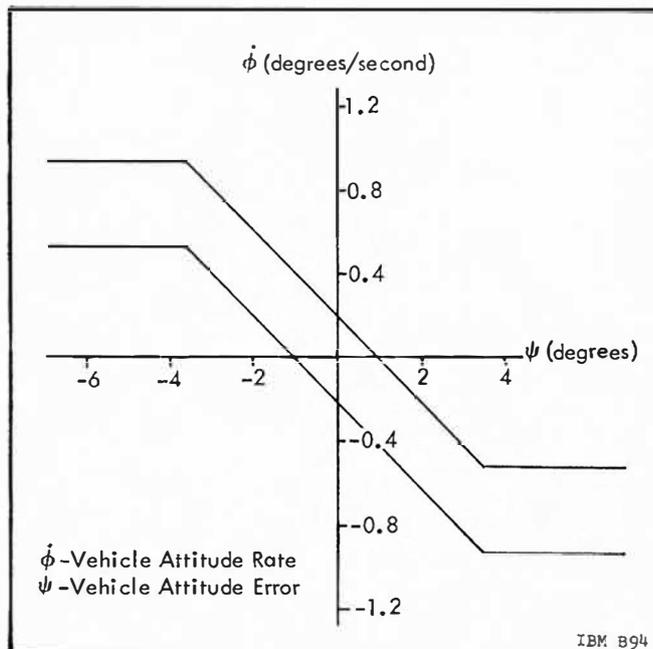
Figure 3.2-5 Roll Deadband for S-IVB Auxiliary Propulsion System
