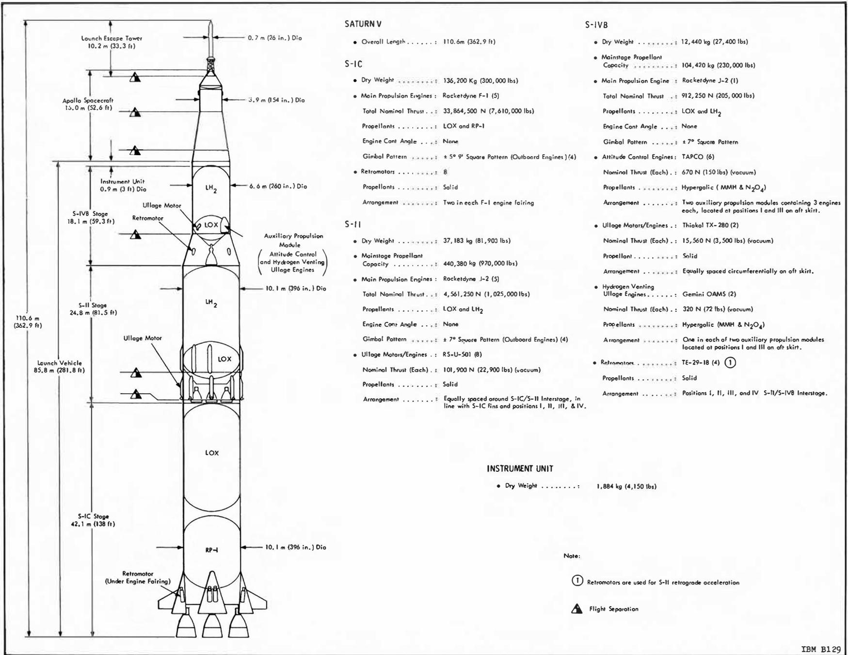
Figure 1.2-2 Saturn V Launch Vehicle Characteristic Data
