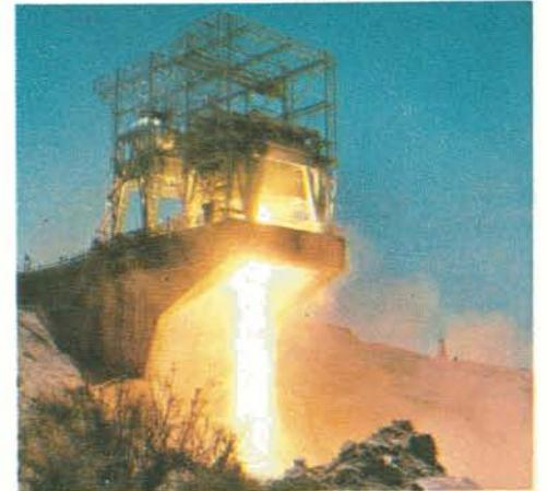
The photo shows a single F-1 engine firing during a captive test.
