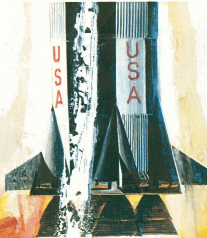
**Apollo/Saturn V is the vehicle that America will use to send man to the moon. Apollo is the spacecraft; Saturn V is the launch vehicle. In a short time the complete "stack" will be launched—for the first time. The first stage alone will develop 7,500,000 lbs. of thrust. We have already taken many big steps toward putting man on the moon; the first Apollo/Saturn V test flight, called the Apollo 4 mission, will be a Giant Step. That's why it's the Big Shot.**
