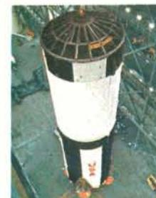
*First Flight of the Saturn S-IC.* The Saturn S-IC first stage, with five F-1 engines, will be launched for the first time—after years of exacting ground tests. Its 7.5 million lbs. of
