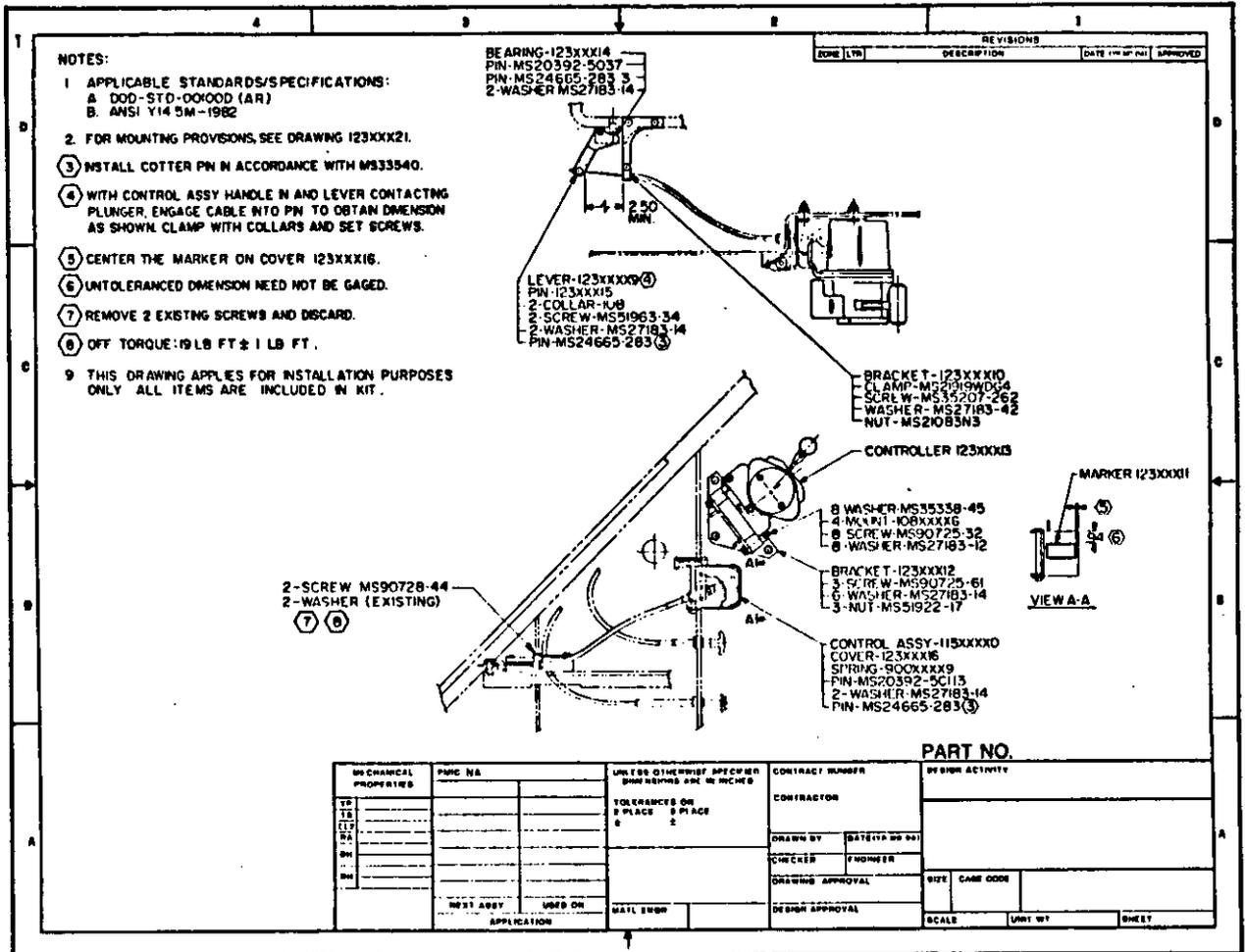
FIGURE 200-36. Installation instruction drawing
