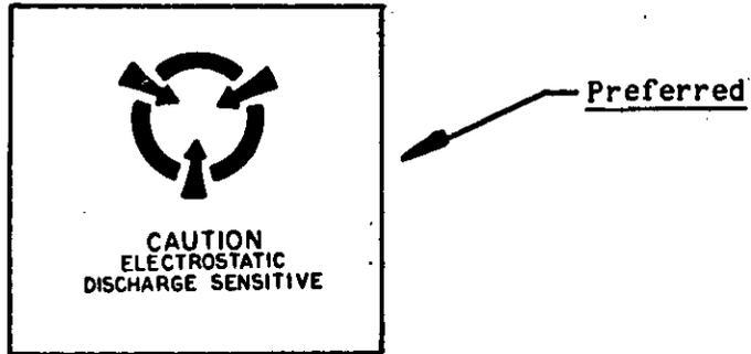
FIGURE 400-6. Sensitive electronic devices (SED) symbol
