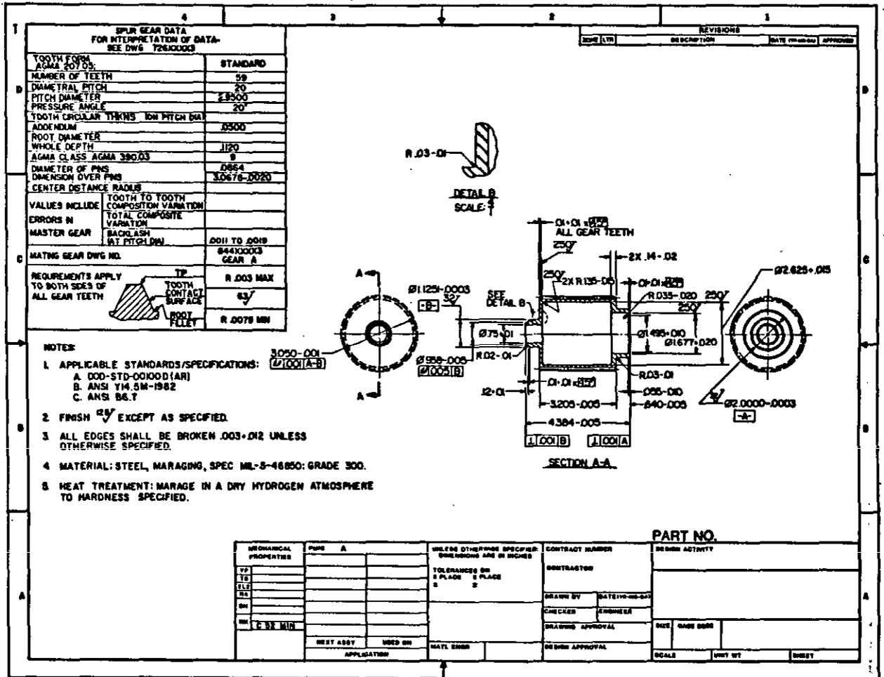
FIGURE D-16. Spur Gear Data Drawing
