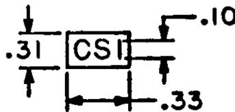
402.16.7.2 Critical Safety Item Assembly. If on an assembly drawing the process or method of assembly is critical, the same rules apply as for a drawing of a critical safety item.
