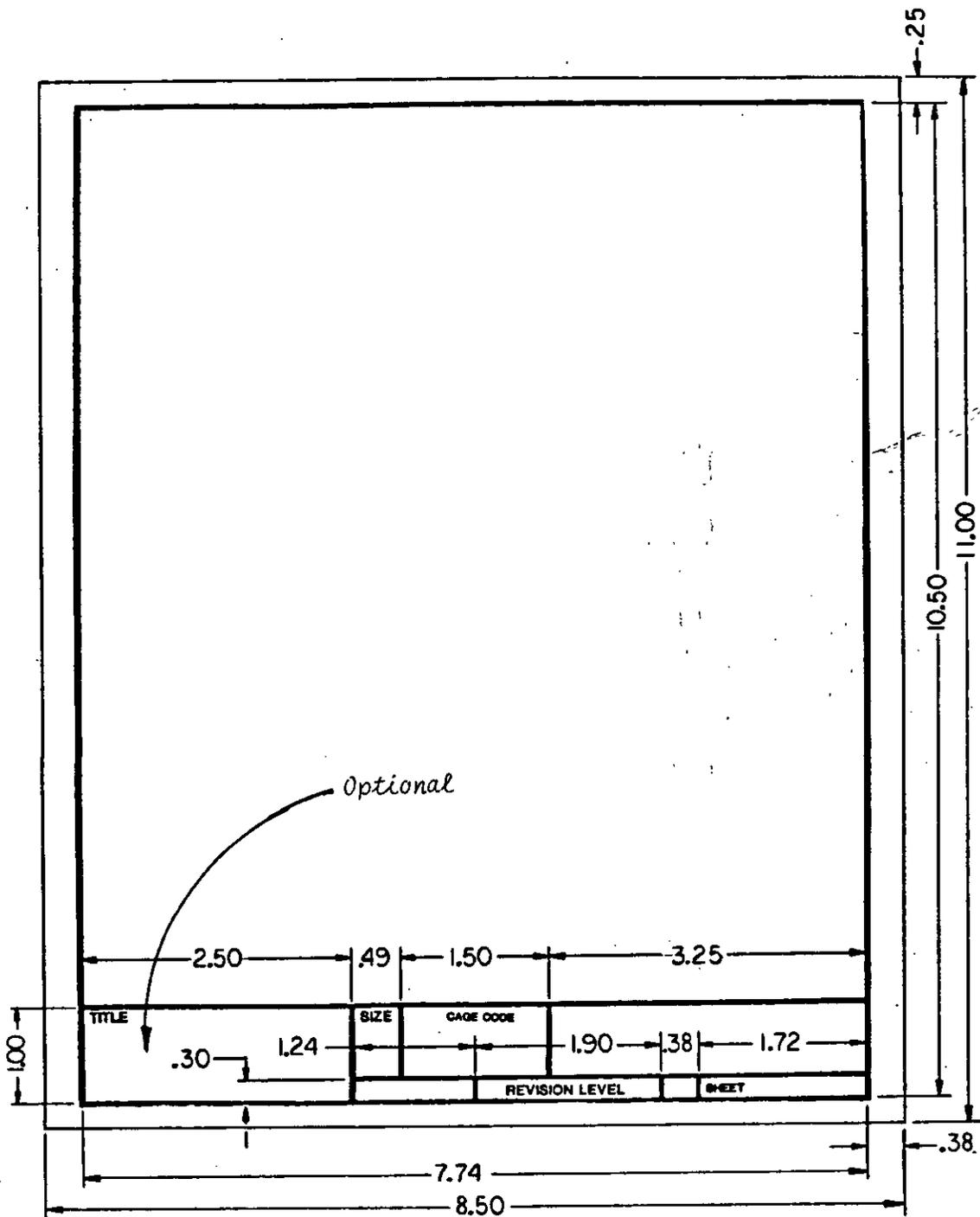
FIGURE A-6. Drawing format for A size continuation sheet
