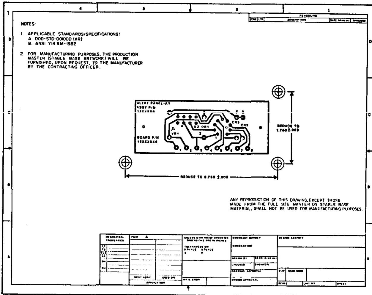
FIGURE 200-34. Printed wiring master pattern drawing
