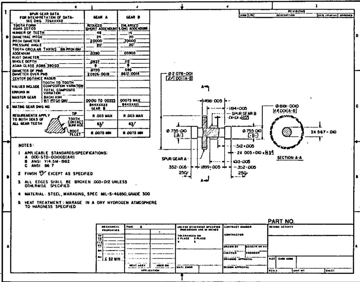
FIGURE D-17. Spur Gear Data Drawing
