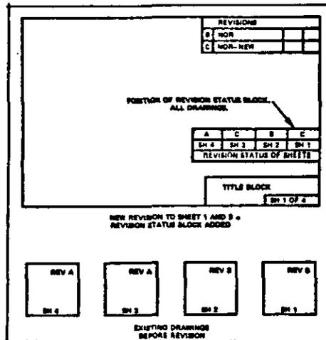
FIGURE 500-4. Revision status to existing drawings
