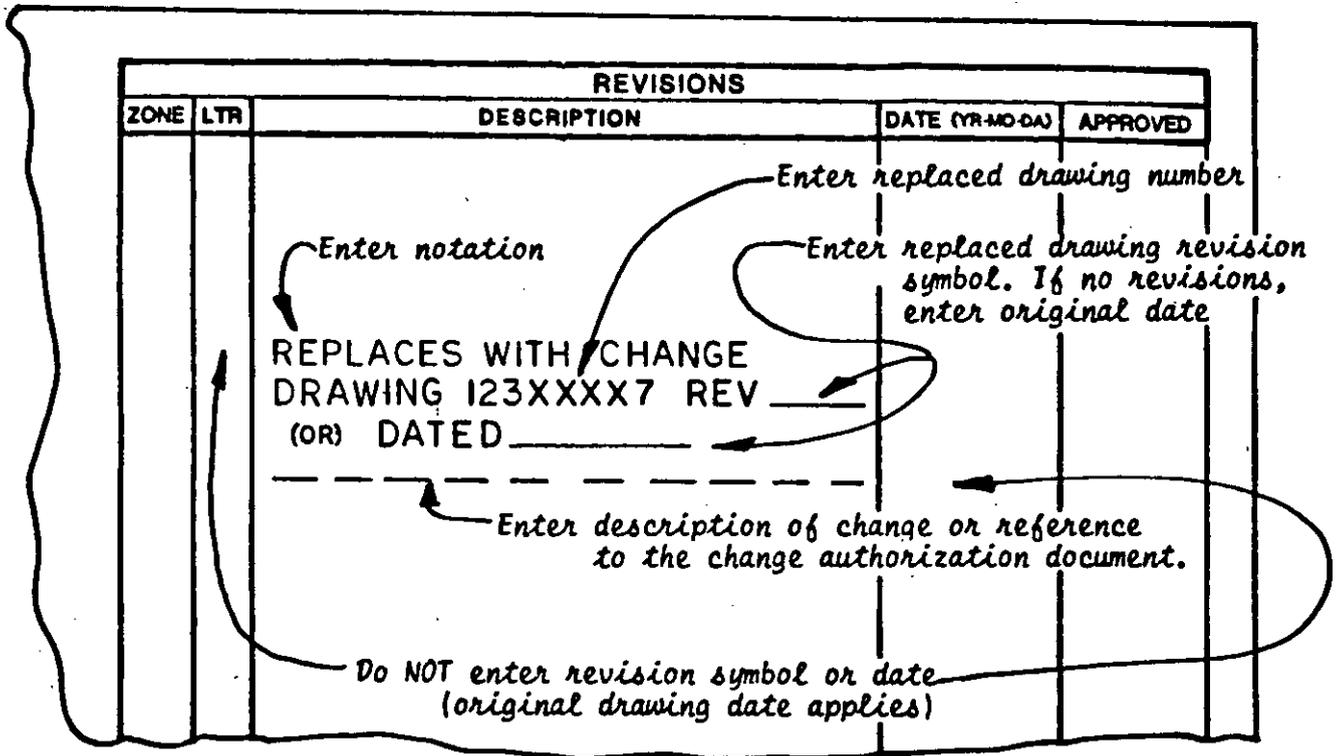
FIGURE 500-7. Superseding (new) Drawing Notations Replacing Drawing with Different Number
