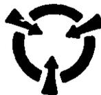
(2) For assemblies, equipment and equipment enclosures, the symbol and accompanying note shall be as shown below.
