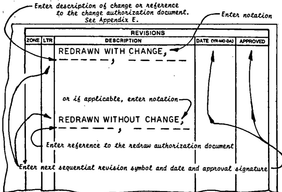
FIGURE 500-5. Superseding (new) Drawing Notations Redrawn with Same Number
