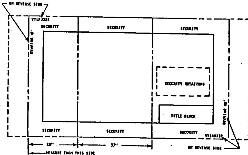
FIGURE B-2. Location of Security Markings on Roll Size Drawings
