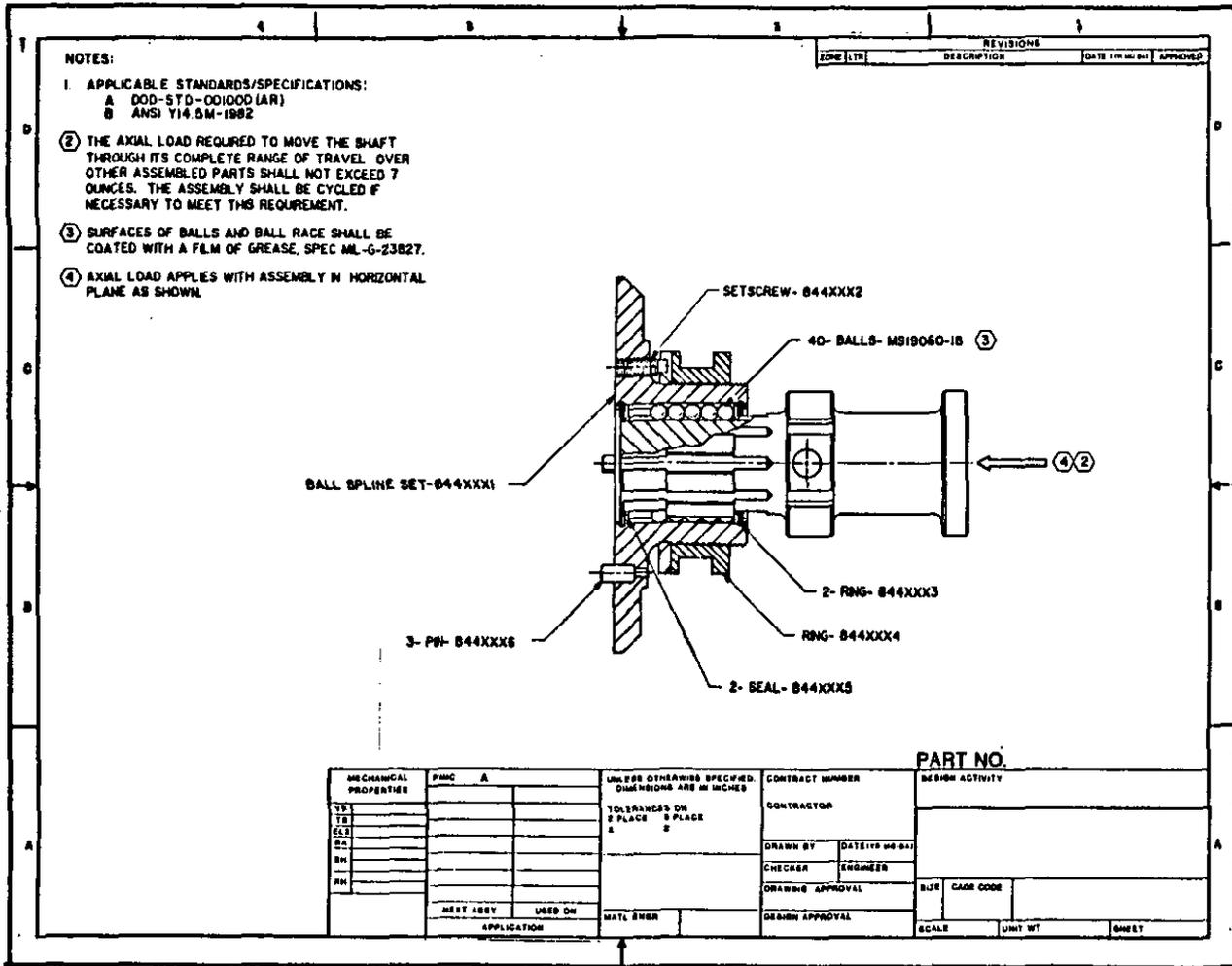
FIGURE 200-6. Assembly drawing
