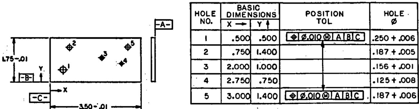
FIGURE 100-6. Tabular Dimensioning Method
