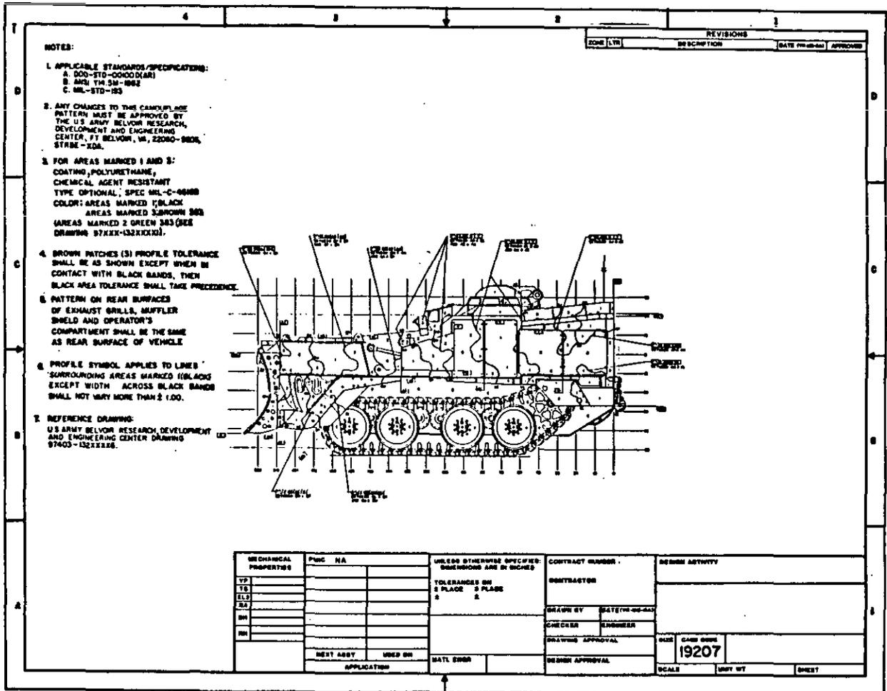
FIGURE 200-45. Vehicle camouflage pattern drawing
