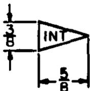
402.19.1 Location of symbol. The symbol shall be placed adjacent to the requirement if in note form and under the dimension for the feature as shown in the following example:
