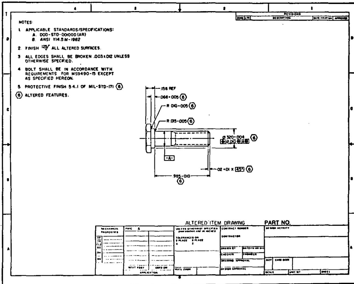
FIGURE 200-15. Altered item drawing (part controlled by Military Standard)
