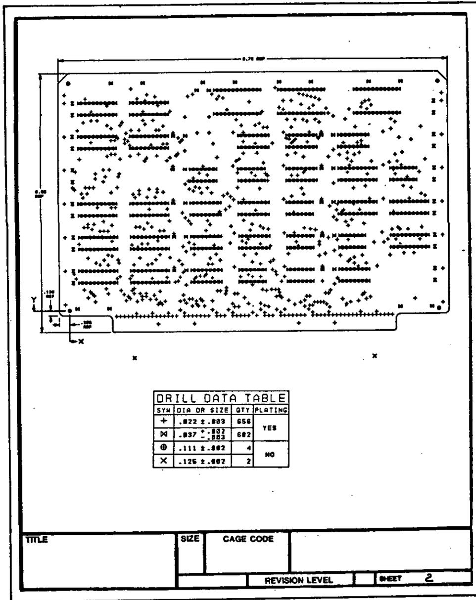
FIGURE D-11. Printed wiring hole location drawing (Cont'd)
