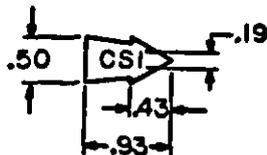
b. Method of Identifying Critical Safety Items on drawings when a leader line is used shall be as shown:
