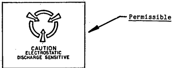
FIGURE 400-6a. Alternative Sensitive electronic devices (SED) symbol
