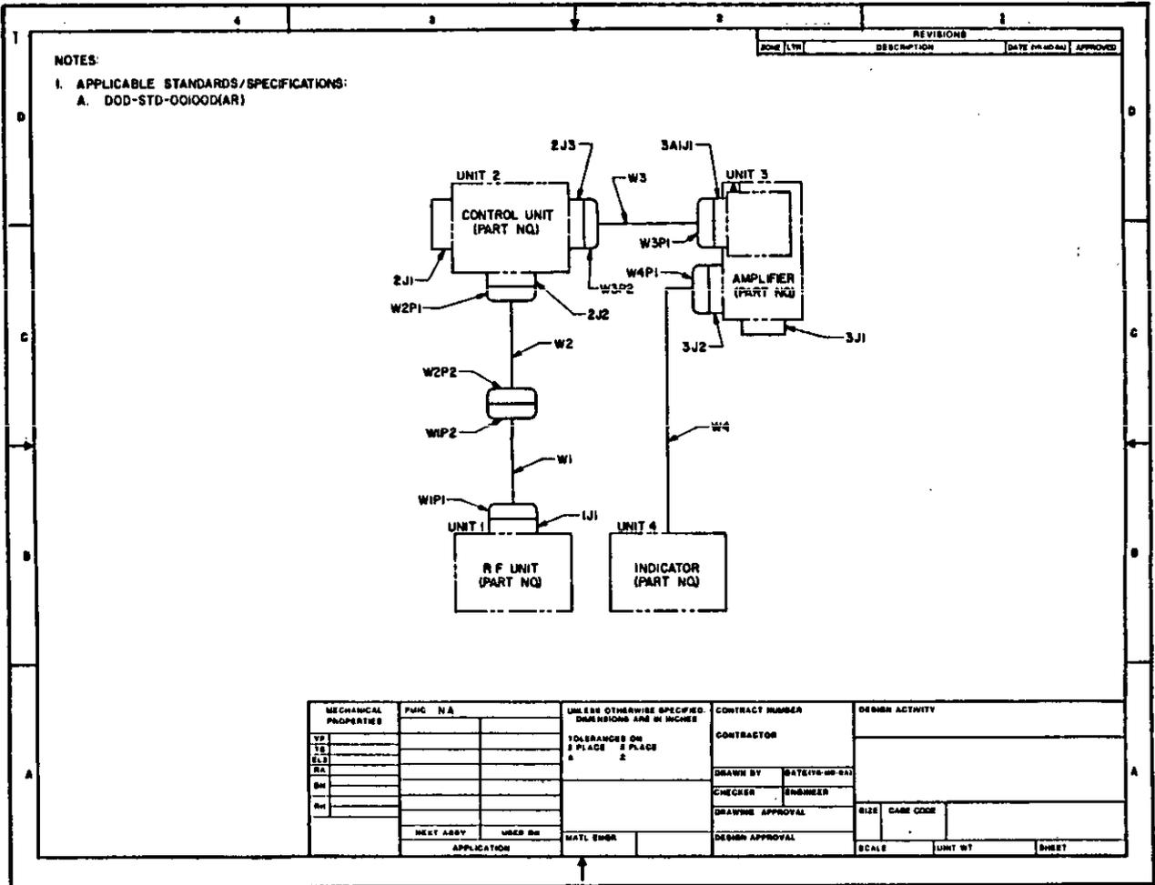
FIGURE 200-23a. Interconnection diagram drawing (cabling type)
