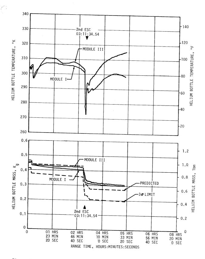
Figure 7-34. S-IVB APS Pressurization System Performance, Sheet 1 of 2
