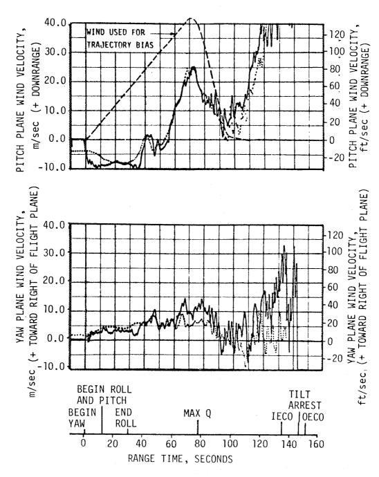
Figure 11-12. Wind Velocity During S-IC Powered Flight
