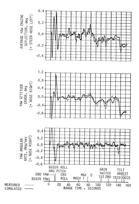
Figure 11-10. Yaw Plane Dynamics During S-IC Burn
