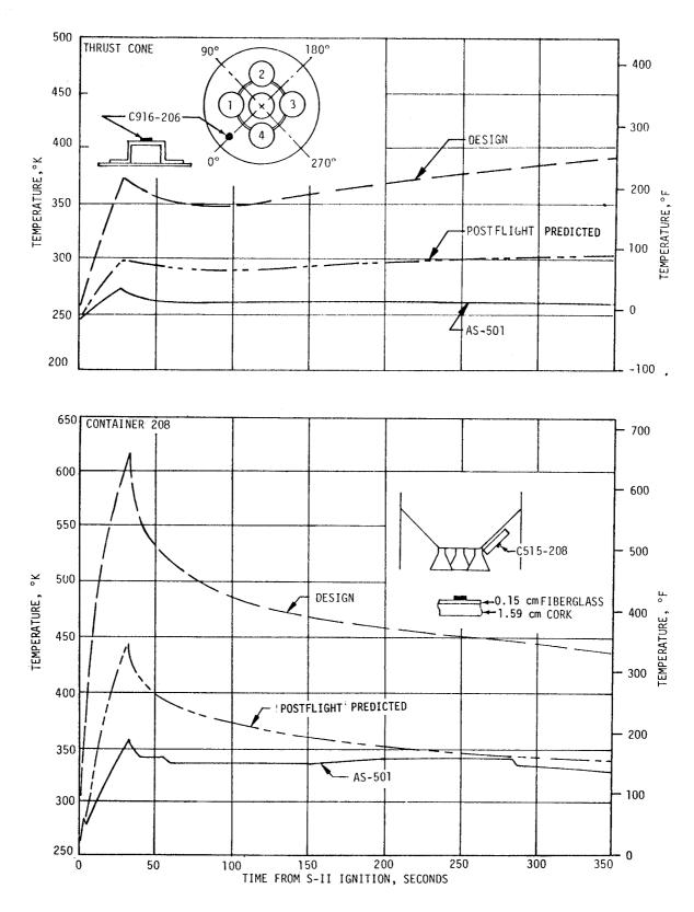
Figure 17-8. Thrust Cone Area Temperatures
