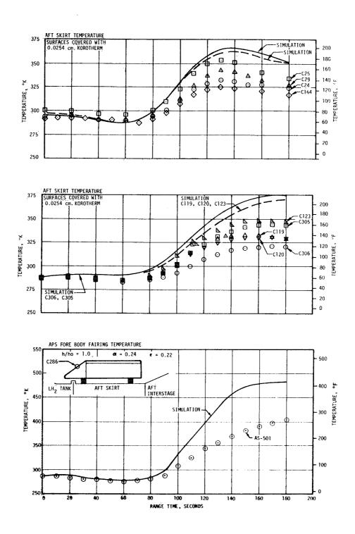
Figure 17-15. S-IVB Protuberance Aeroheating Environment
