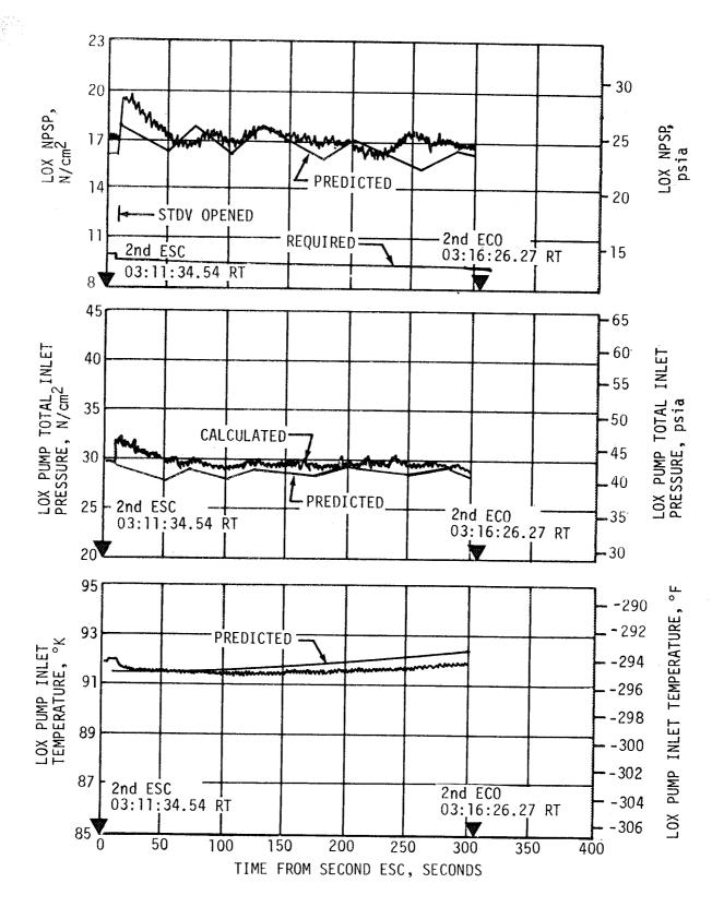
Figure 7-29. S-IVB LOX Pump Inlet Conditions - Second Burn
