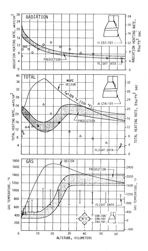
Figure 17-2. F-1 Engine Thermal Environment
