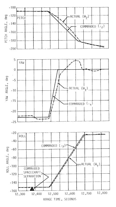
Figure 11-39 Vehicle Attitude Following Spacecraft Separation
