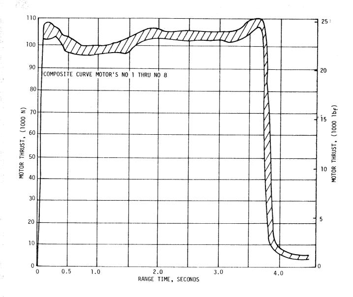
Figure 12-2. S-II Ullage Motor Thrust
