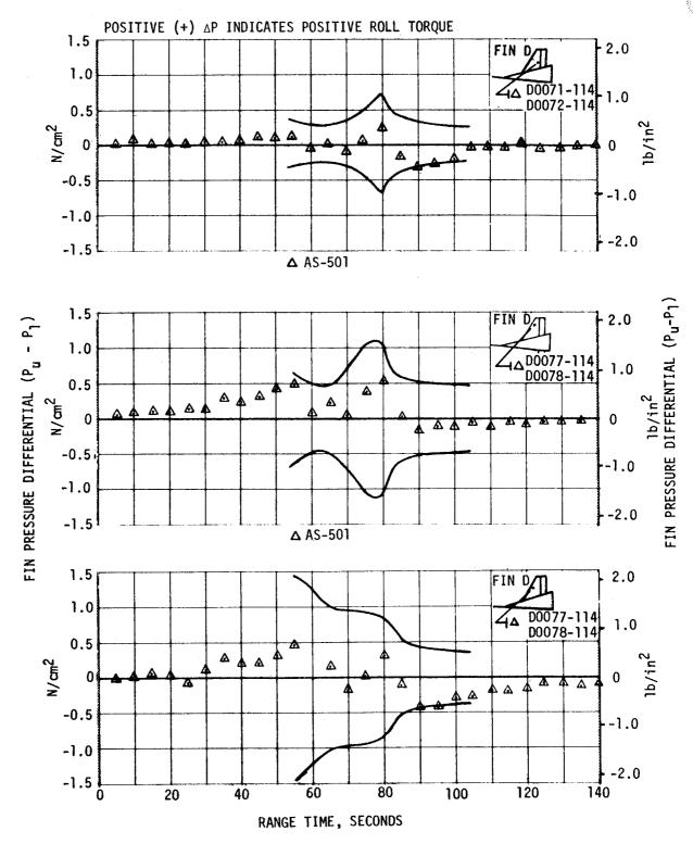
Figure 20-3. S-IC Fin Pressure Differential, Sheet 2 of 2
