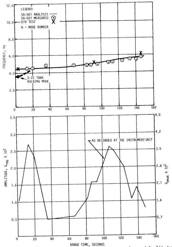
Figure 9-6. First Longitudinal Modal Frequencies and Amplitudes
