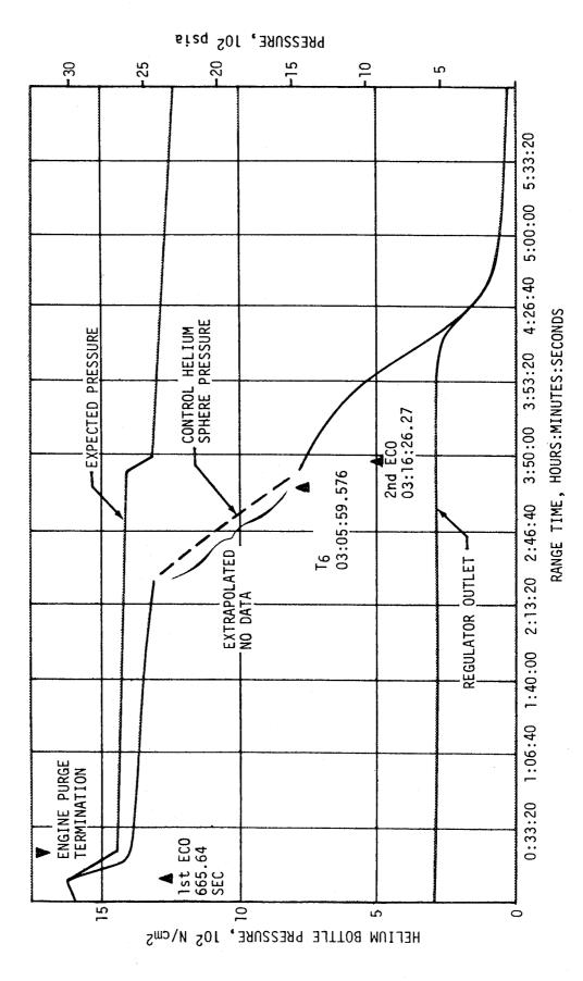
Figure 7-30. S-IVB Pneumatic Control Helium Bottle Pressure
