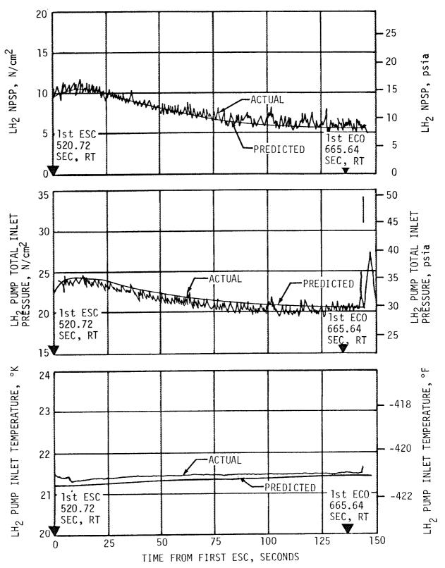
Figure 7-23. S-IVB Fuel Pump Inlet Conditions - First Burn
