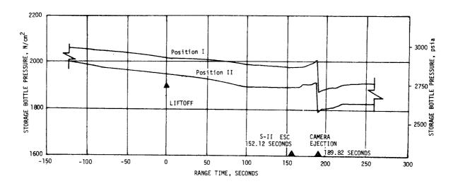
Figure 6-20 S-II Camera Ejection System Pressures
