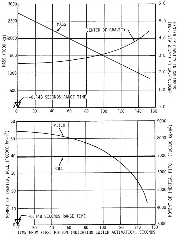
Figure 21-1. Vehicle Mass, Center of Gravity, and Mass Moment of Inertia During S-IC Stage Powered Flight
