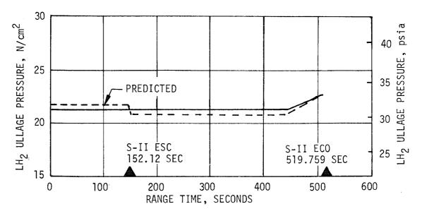
Figure 6-13. S-II LH<sub>2</sub> Ullage Pressure During S-II Burn
