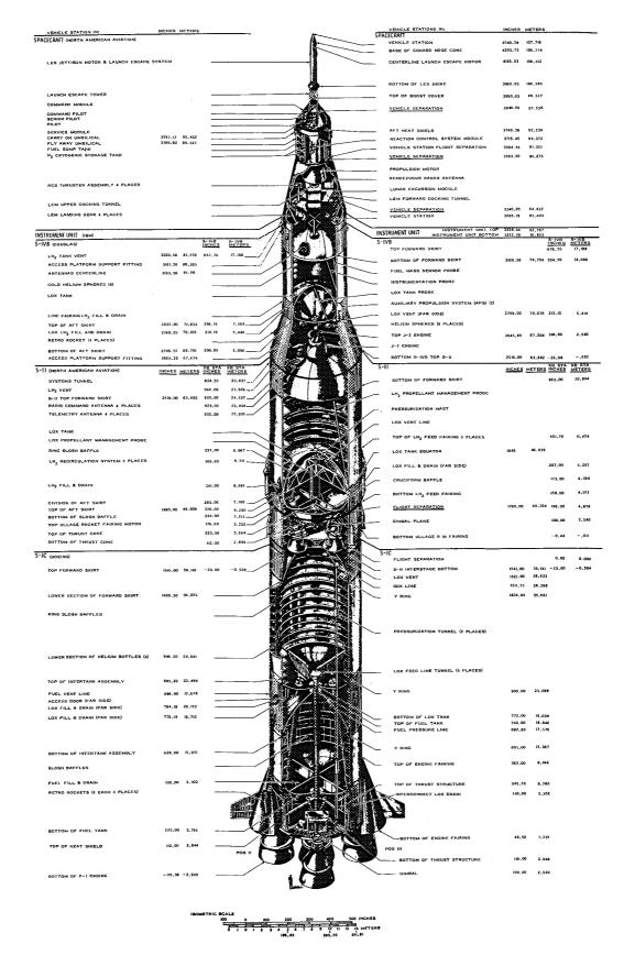
Figure B-1. Saturn V Apollo Flight Configuration
