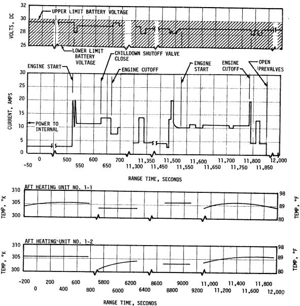
NOTE: PREDICTED CURRENT WAS BASED ON MAXIMUM LOADS. VALUES ARE BEYOND THE SCALE OF THESE PLOTS AND THEREFORE NOT SHOWN. ACTUAL CURRENT FELL WELL BELOW PREDICTED.
