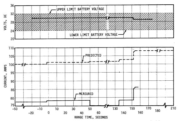
Figure 13-2. S-IC Stage Voltage and Current, Bus 1D20
