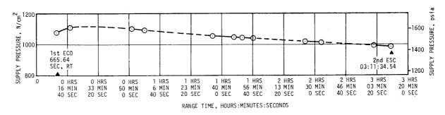
Figure 7-27. S-IVB Cold Helium Sphere Condition - Coast Phase
