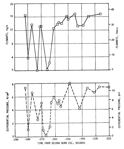
Figure 7-12. S-IVB LOX Pump Chilldown Performance - Second Burn
