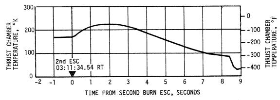
Figure 7-11. S-IVB Thrust Chamber Temperature - Second Burn
