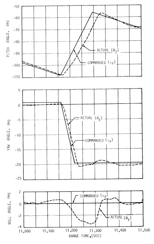
Figure 11-32. Vehicle Attitude During Restart Orientation Maneuver
