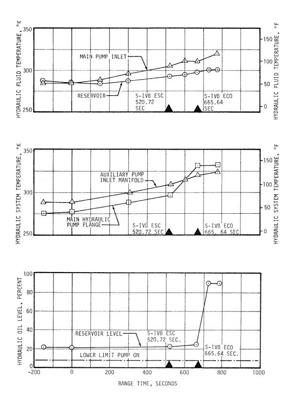
Figure 8-3. S-IVB Hydraulic System Performance - First Burn
