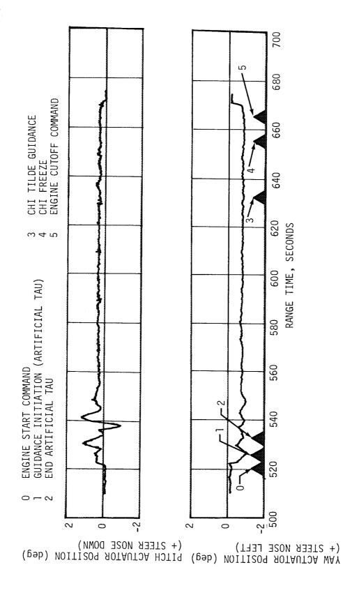
S-IVB Pitch and Yaw Actuator Positions During First Burn Figure 11-28.
