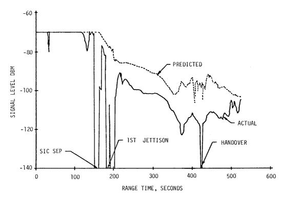
Figure 19-6. Merritt Island CCS Down Link Carrier Signal Strength, AS-501
