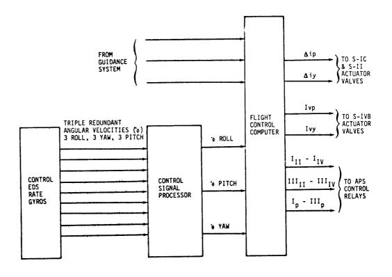
Figure 11-1. Control Components Block Diagram
