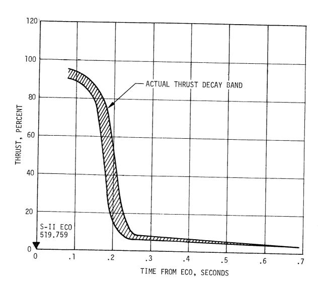
Figure 6-8. S-II Engine Shutdown Transient
