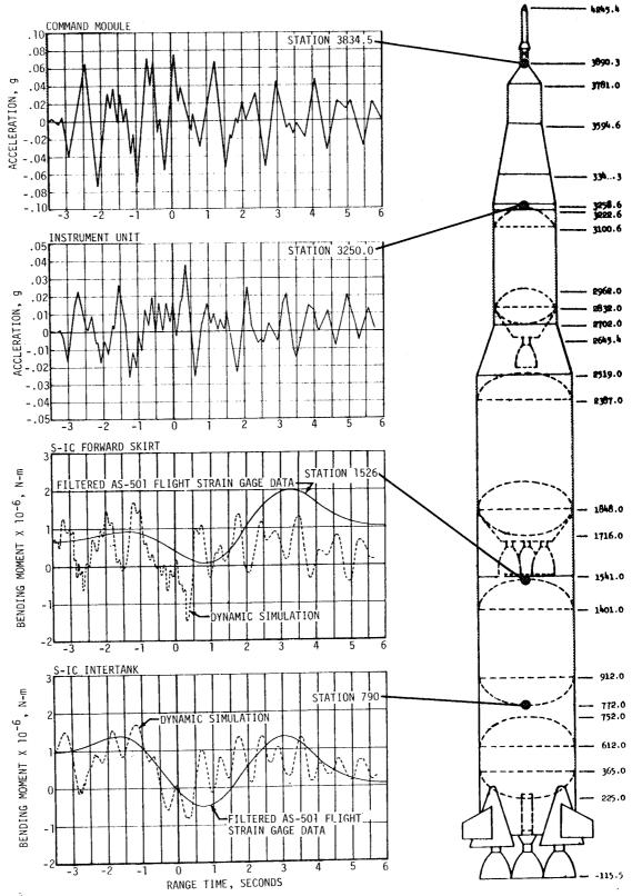
Figure 9-4. Lateral (Pitch) Structural Dynamic Response During
