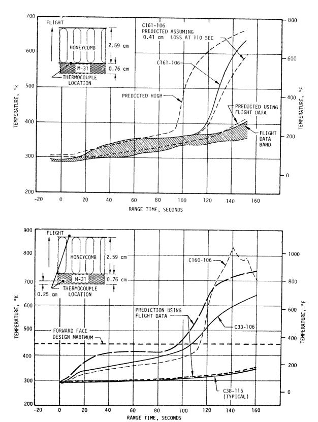
Figure 17-5. S-IC Base Heat Shield Structural Temperatures
