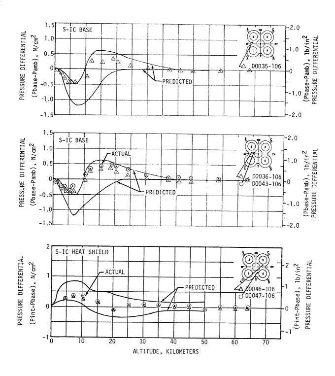
Figure 16-8. S-IC Base Heat Shield Pressure Environment
