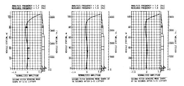
Figure 9-9. Pitch Mode Shapes During S-IC Powered Flight
