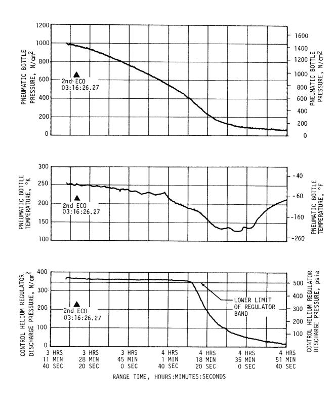
Figure 7-32. S-IVB Pneumatic Control Performance - Second Burn
