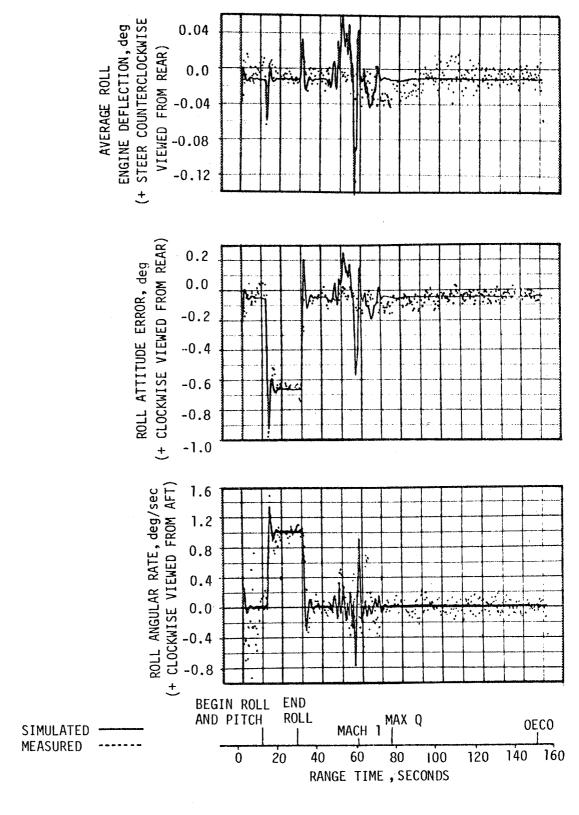
Figure 11-11. Roll Plane Dynamics During S-IC Burn
