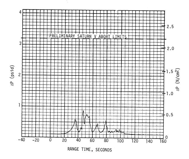
Figure 15-2. Q-Ball  $\Delta P$  Versus Flight Time 15-5
