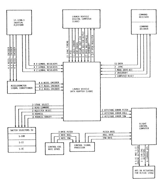
Figure 10-1. Navigation, Guidance, and Control System Block Diagram
