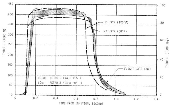
Figure 12-1. S-IC Retro Motors Thrust
