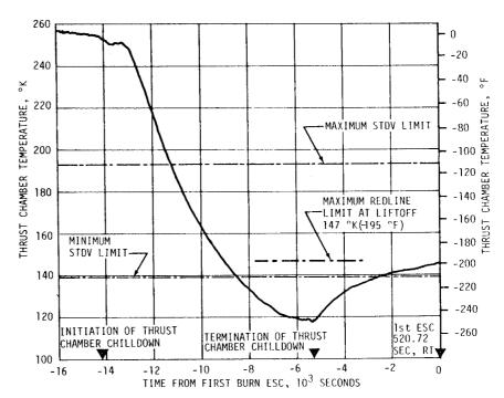
Figure 7-2. S-IVB Thrust Chamber Temperature - First Burn
