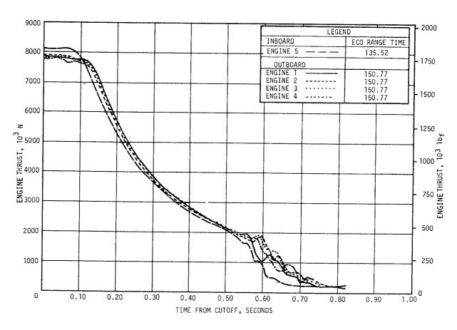
Figure 5-4. S-IC Engine Shutdown Transient Performance
