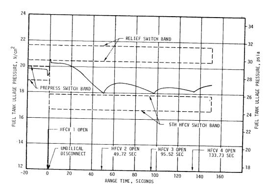
Figure 5-7. S-IC Fuel Ullage Pressure During Boost
