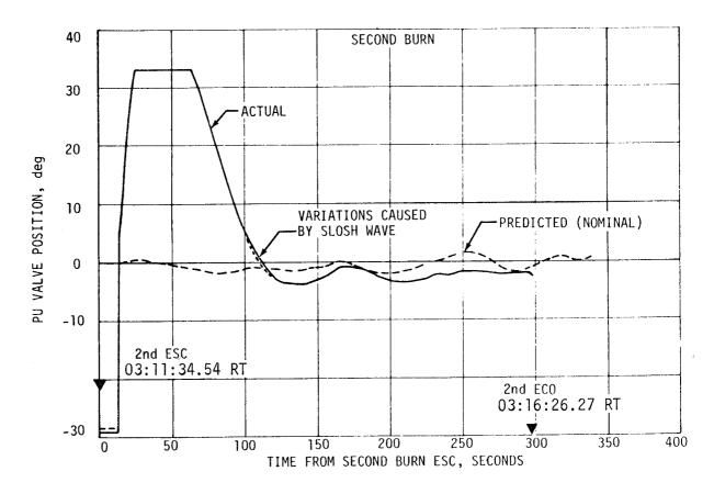
Figure 7-17. S-IVB PU Valve Positions
