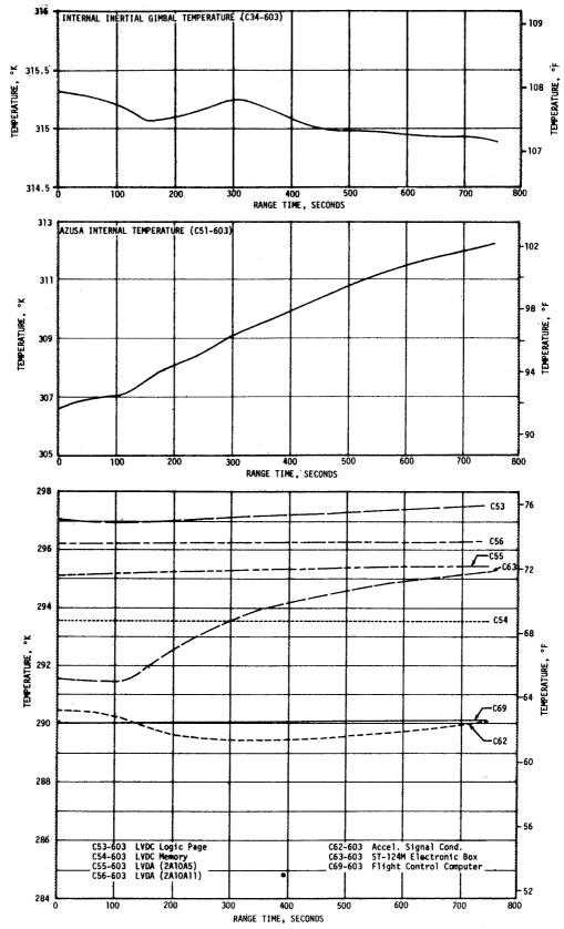
Figure 18-5. Selected Component Temperatures
