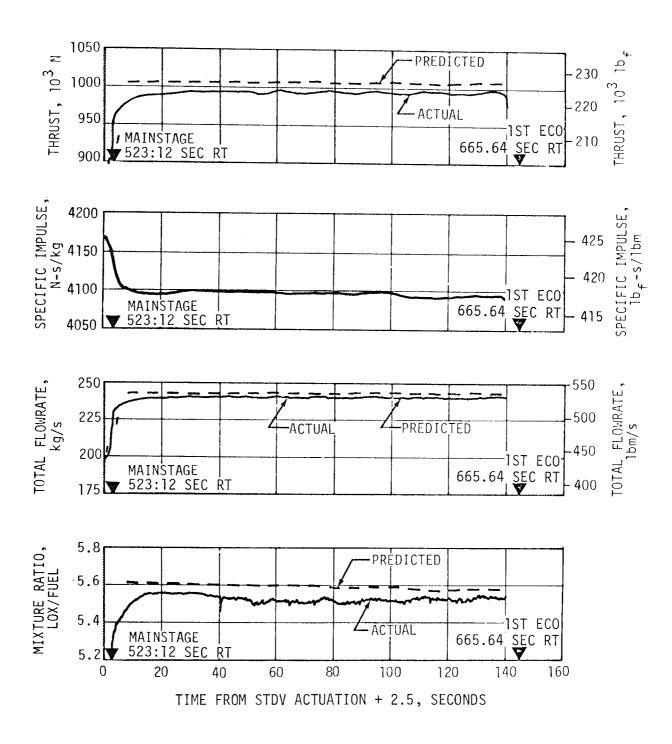
Figure 7-5. S-IVB Steady State Operation - First Burn
