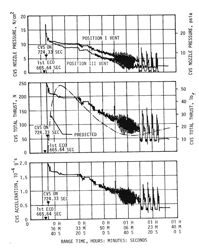
Figure 7-8. S-IVB CVS Performance - Coast Phase, Sheet 1 of 2
