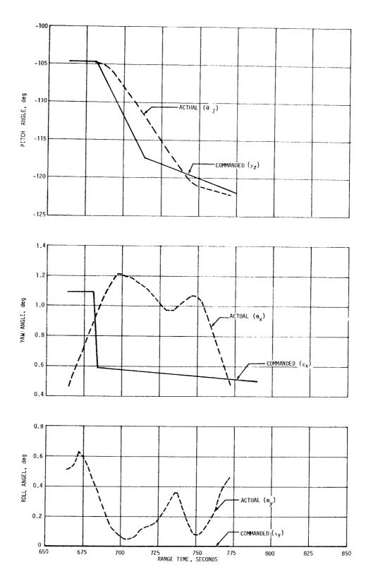
Figure 11-31. Vehicle Attitude Following S-IVB First Burn Cutoff
