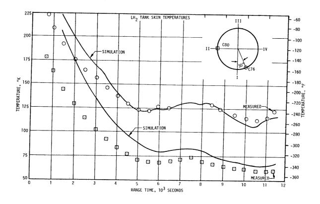
Figure 17-18.  $LH_2$  Heating During Orbit and Tank Skin Temperatures
