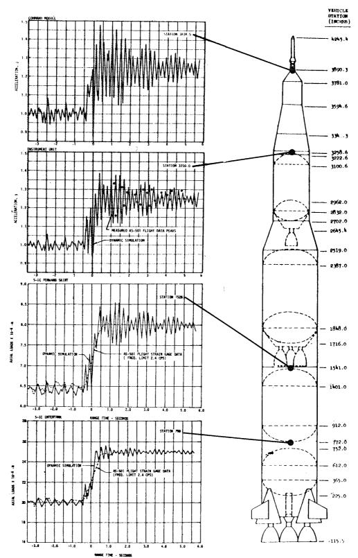
Figure 9-1. Longitudinal Structural Dynamic Response Due to Thrust Buildup and Release
