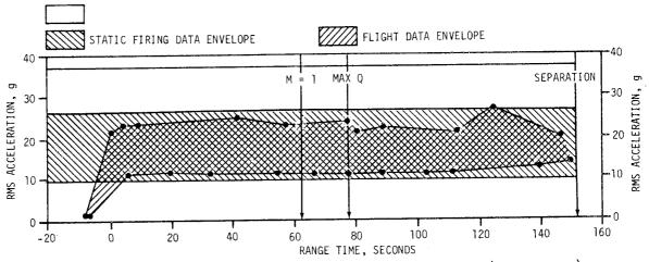
Figure 9-12. S-IC Stage Engine Vibration Envelopes (Turbopump)
