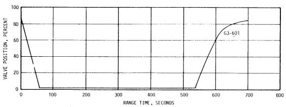
Figure 18-4. Modulating Flow Control Valve Performance
