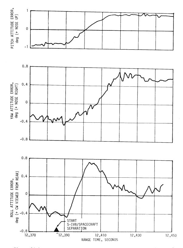
Figure 12-16. S-IVB-IU Attitude Errors During Spacecraft Separation
