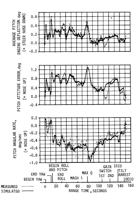
Figure 11-9. Pitch Plane Dynamics During S-IC Burn
