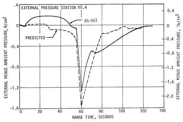
Figure 16-5. Sidewall Insulation Differential Pressures
