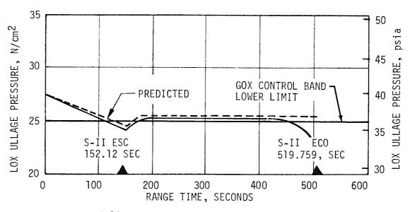
Figure 6-16. S-II LOX Ullage Pressure During Burn
