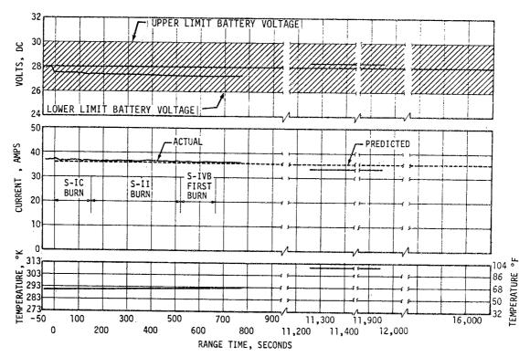
Figure 13-13. IU Battery 6D30 Voltage, Current, and Temperature
