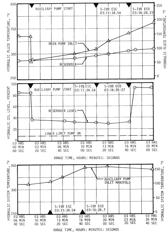
Figure 8-5 S-IVB Hydraulic System Performance - Second Burn
