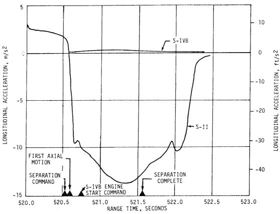
Figure 12-12. S-II/S-IVB Longitudinal Acceleration
