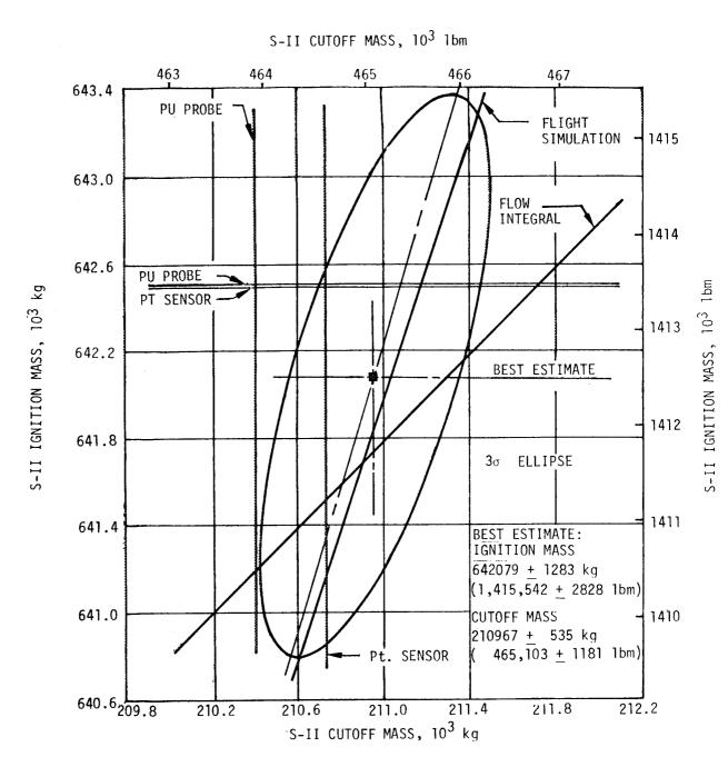
Figure 6-11. Stage Mass at S-II Ignition and Cutoff
