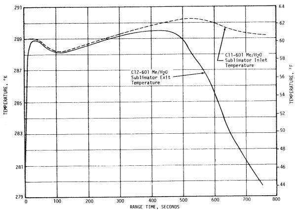
Figure 18-2. Sublimator Inlet and Exit Temperatures
