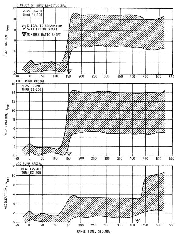
Figure 9-15. S-II Stage Engine Vibration Envelopes
