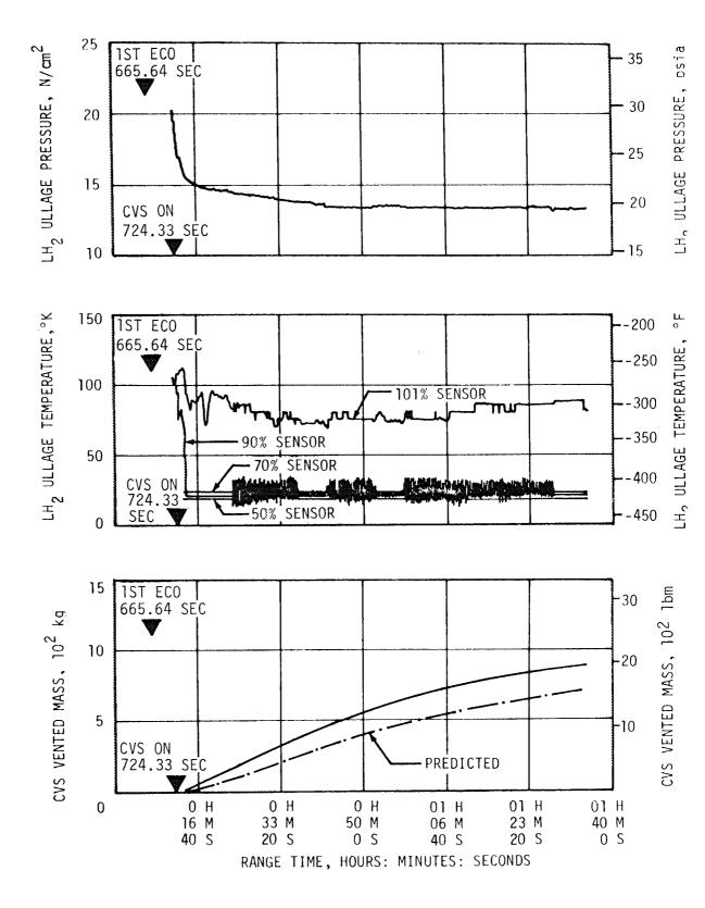
Figure 7-9. S-IVB  $LH_2$  Ullage Conditions - Coast Phase, Sheet 1 of 2
