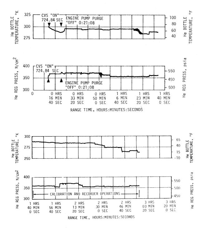
Figure 7-31. S-IVB Pneumatic Control Performance
