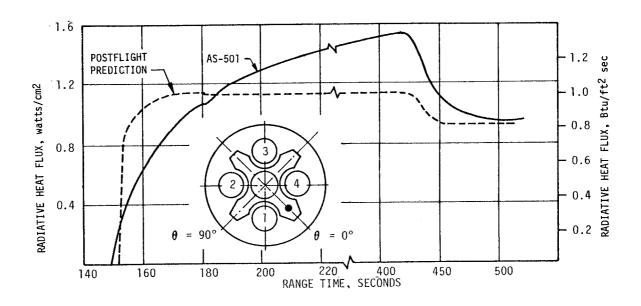
Figure 17-6. S-II Heat Shield Heating Rates
