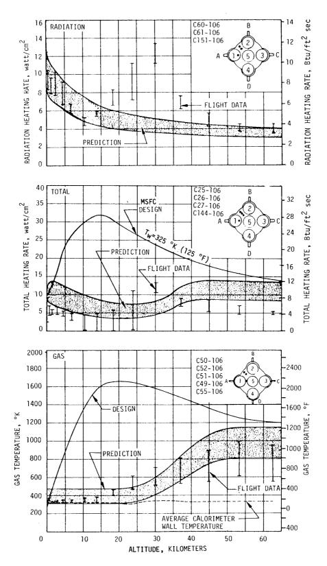
Figure 17-1. S-IC Base Heat Shield Thermal Environment
