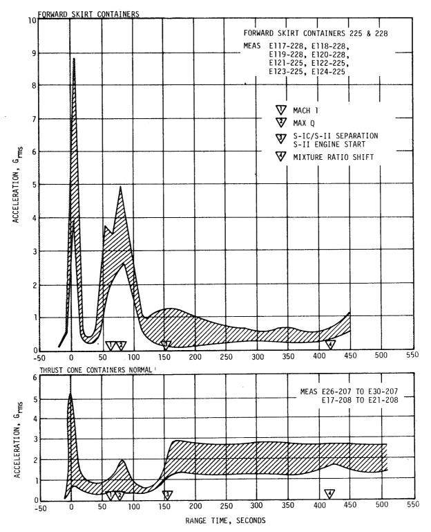
Figure 9-16. S-II Stage Component Vibration Envelopes
