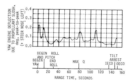
Figure 11-18. S-IC Engine Deflection Response to Propellant Slosh
