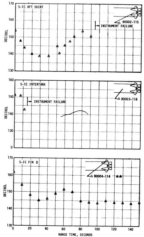
Figure 16-11. Vehicle Overall Fluctuating Pressure Level, Sheet 2 of 2
