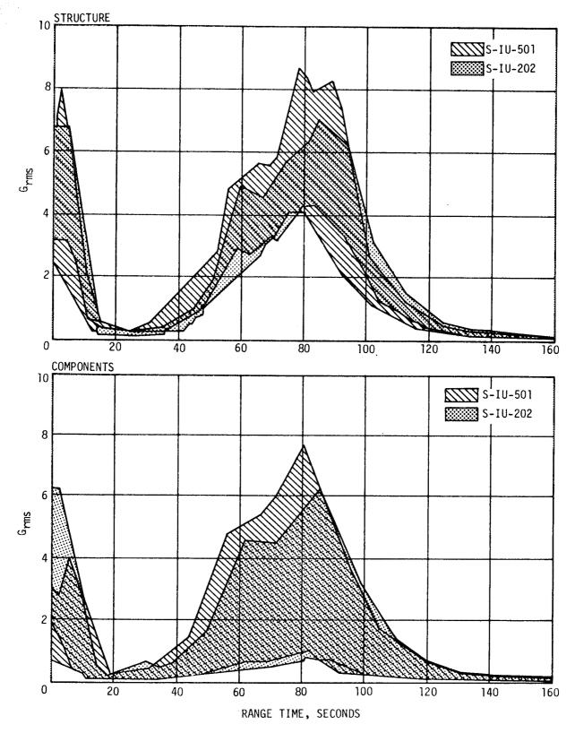
Figure 9-19. Instrument Unit Vibration Envelopes
