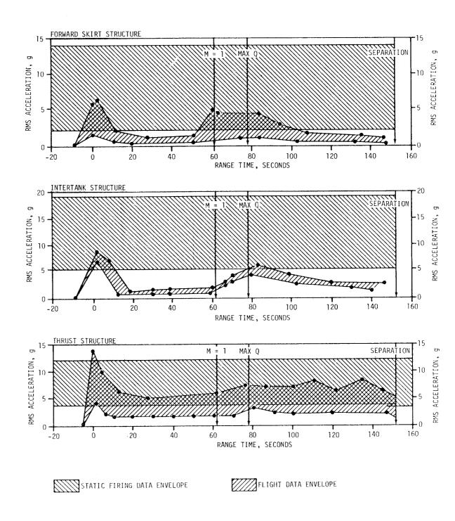
Figure 9-11. S-IC Stage Structure Vibration Envelopes
