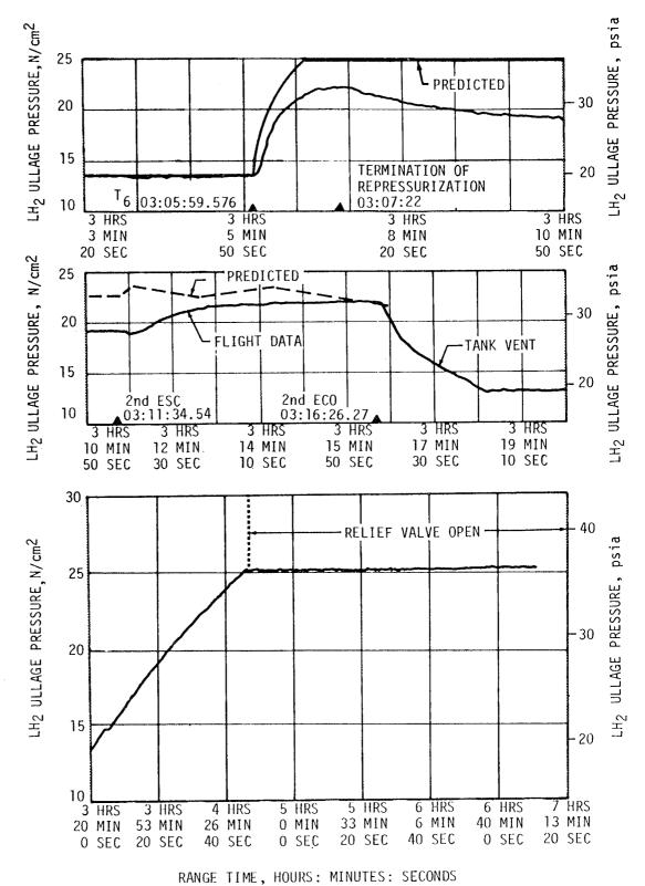
Figure 7-22. S-IVB LH<sub>2</sub> Ullage Pressure - Second Burn
