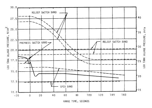
Figure 5-9. S-IC LOX Ullage Pressure
