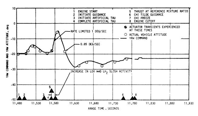
Figure 11-36. Vehicle Attitude During S-IVB Second Burn
