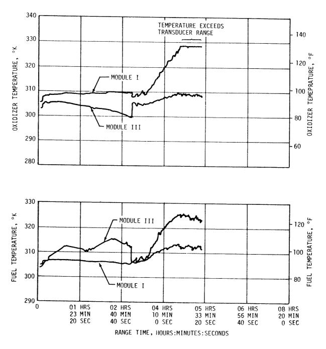
Figure 7-36. S-IVB APS Propellant Conditions
