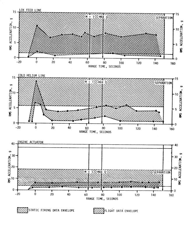
Figure 9-13. S-IC Stage Components Vibration Envelopes
