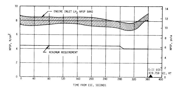
Figure 6-14. S-II Fuel Pump Inlet Conditions
