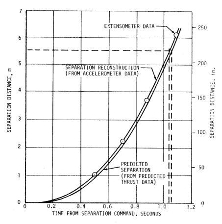
Figure 12-11. S-II/S-IVB Separation Distance
