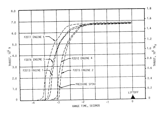
Figure 5-2. S-IC Engine Buildup Transient
