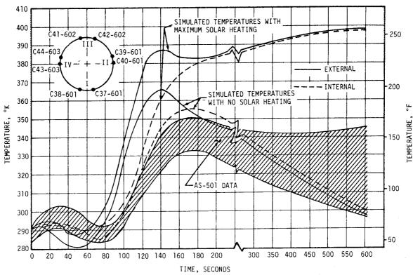
Figure 17-16. Instrument Unit Skin Temperature
