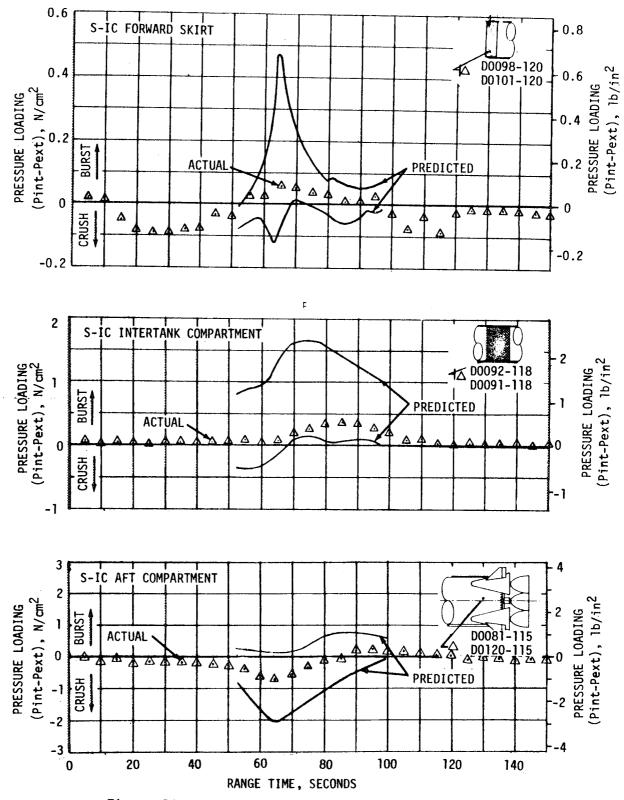
Figure 16-3. S-IC Compartment Pressure Loads
