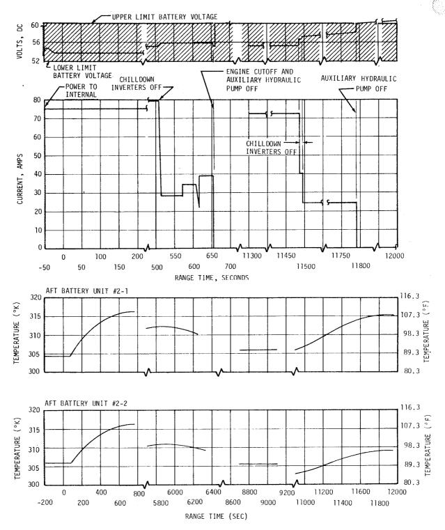
NOTE: PREDICTED CURRENT WAS BASED ON MAXIMUM LOADS. VALUES ARE BEYOND THE SCALE OF THESE PLOTS AND THEREFORE NOT SHOWN. ACTUAL CURRENT FELL WELL BELOW PREDICTED.
