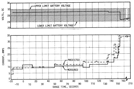
Figure 13-1. S-IC Stage Voltage and Current, Bus 1D10
