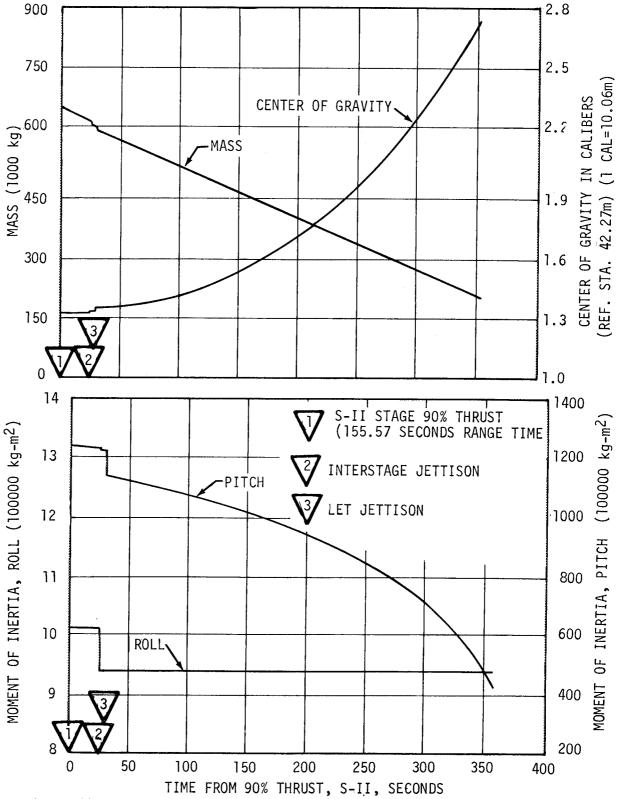
Figure 21-2. Total Vehicle Mass, Center of Gravity, and Mass Moment of Inertia During S-II Stage Powered Flight
