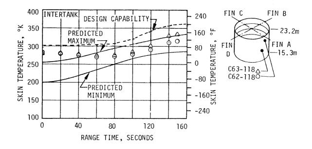
Figure 17-9. S-IC Body Aerodynamic Heating
