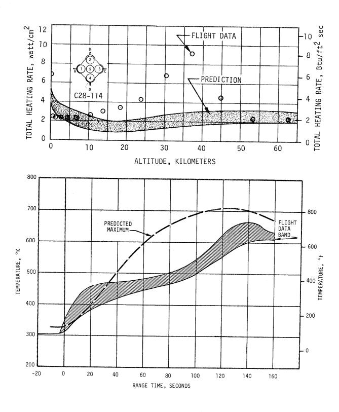
Figure 17-3. S-IC Fin Aft Face Thermal Environment
