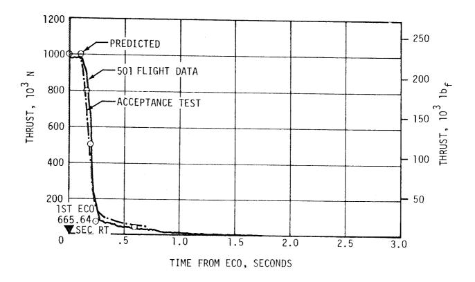
Figure 7-6. S-IVB Shutdown Transient Performance - First Burn
