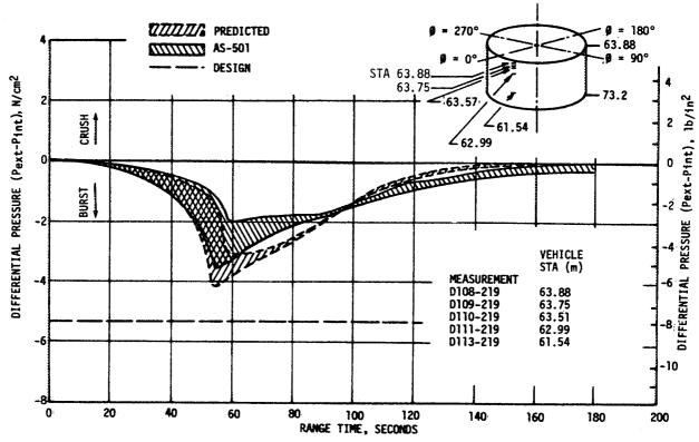
Figure 16-4. Forward Skirt Differential Pressures
