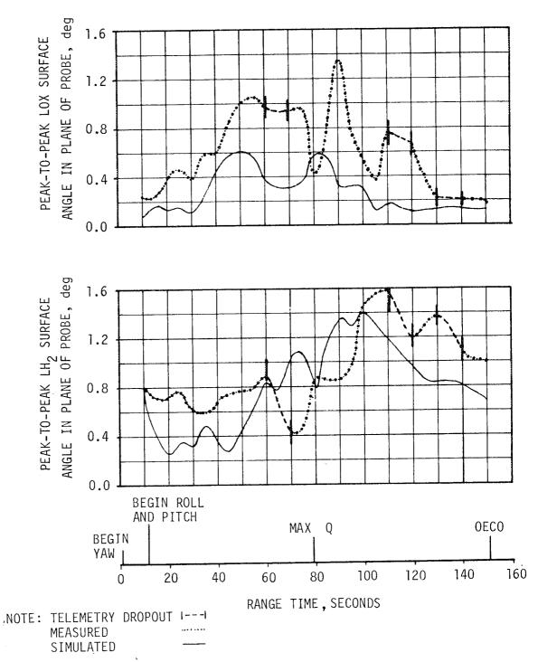
Figure 11-17. S-II Propellant Slosh Amplitudes During S-IC Burn
