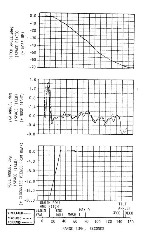
Figure 11-8. Vehicle Attitude During S-IC Burn
