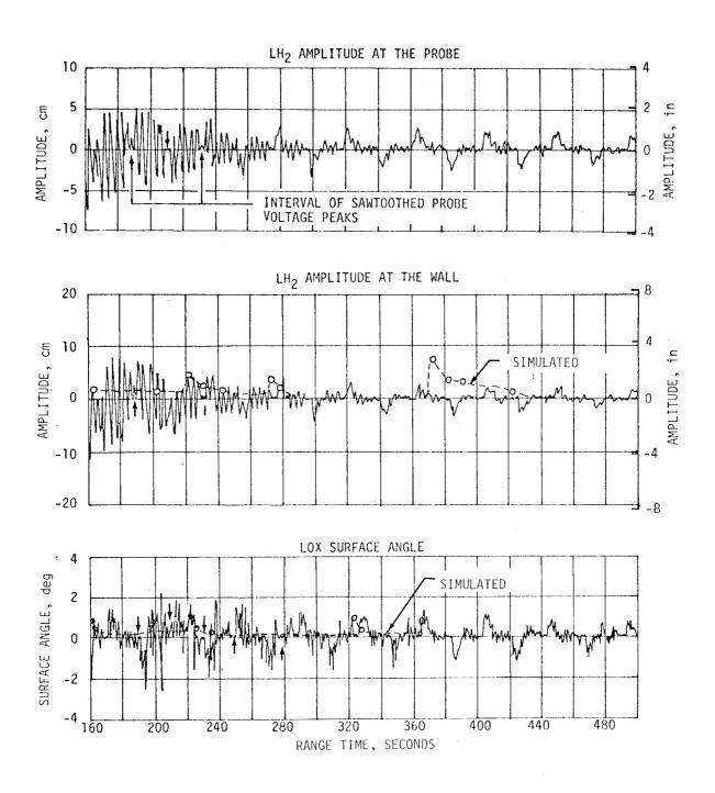
Figure 11-23. LH<sub>2</sub> and LOX Slosh Amplitudes During S-II Flight
