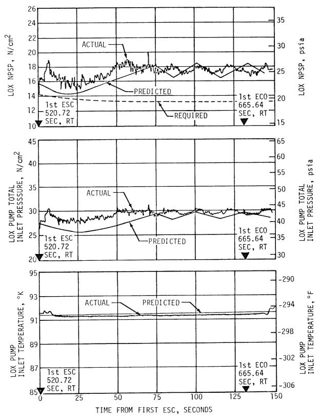
Figure 7-28. S-IVB LOX Pump Inlet Conditions - First Burn
