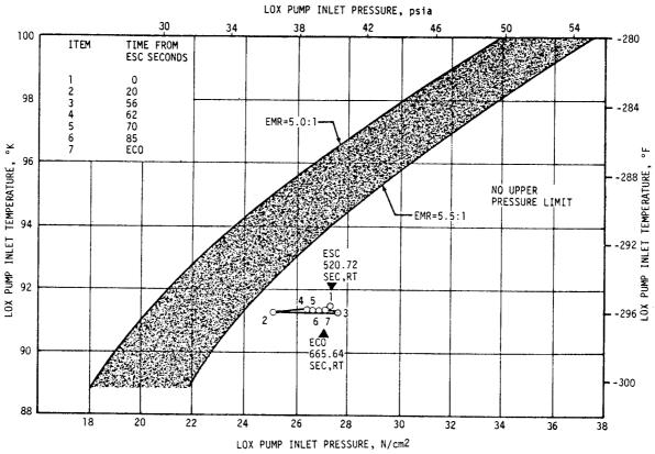
Figure 7-1. S-IVB Start Box and Run Requirements - First Burn
