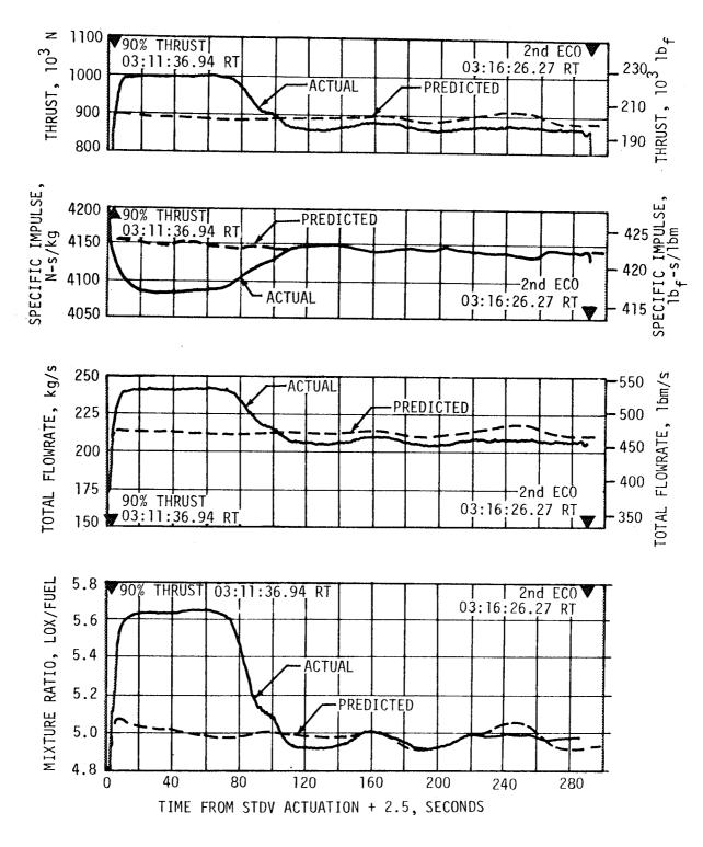
Figure 7-14. S-IVB Steady State Operation - Second Burn
