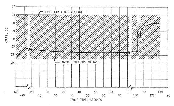
Figure 13-6. S-II Stage Ignition DC Voltage
