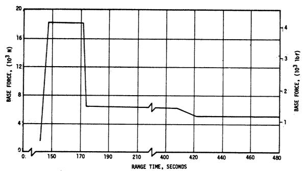
Figure 20-2. Base Pressure Thrust Increment During S-II Boost
