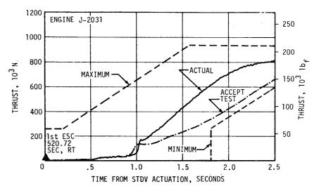
Figure 7-4. S-IVB Buildup Transient - First Burn
