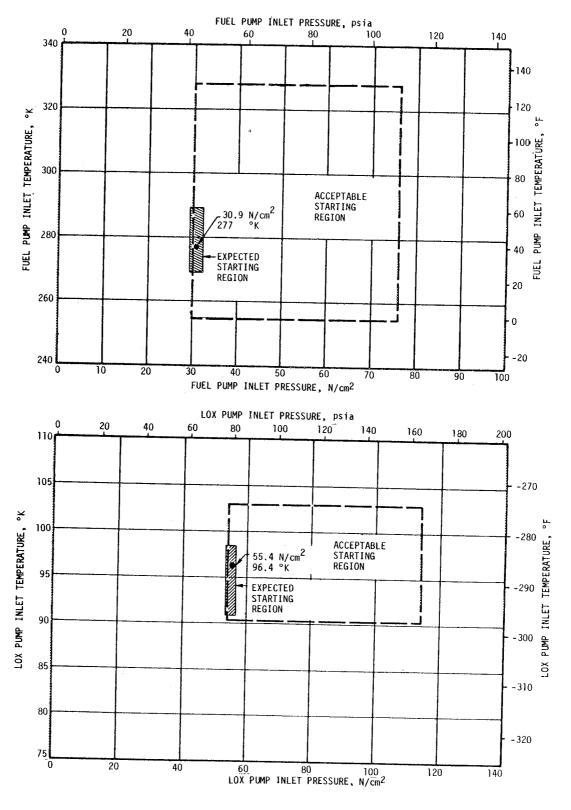
Figure 5-1. S-IC Start Box Requirements
