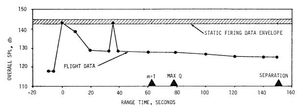
Figure 16-13. S-IC Acoustic Environment, Acoustic Measurement Summary
