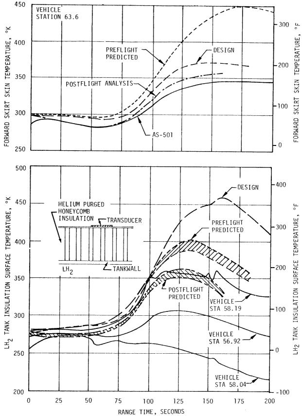
Figure 17-12. Forward Skirt Skin and Insulation Temperatures
