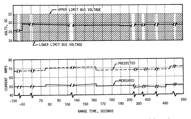
Figure 13-4. S-II Stage Instrumentation Bus Voltage and Current
