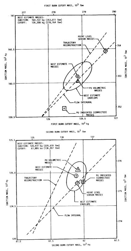
Figure 7-16. S-IVB Ignition and Cutoff Best Estimate Masses
