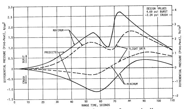
Figure 16-7. S-II/S-IVB Interstage Pressure Loading
