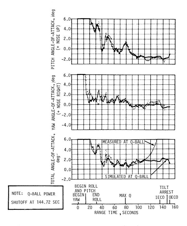
Figure 11-13. Free Stream Angle-of-Attack During S-IC Burn
