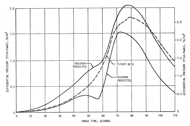
Figure 16-6. S-II/S-IVB Interstage Pressure Differential
