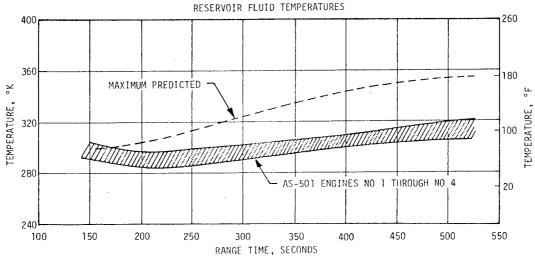
Figure 8-2. S-II Hydraulic System Performance
