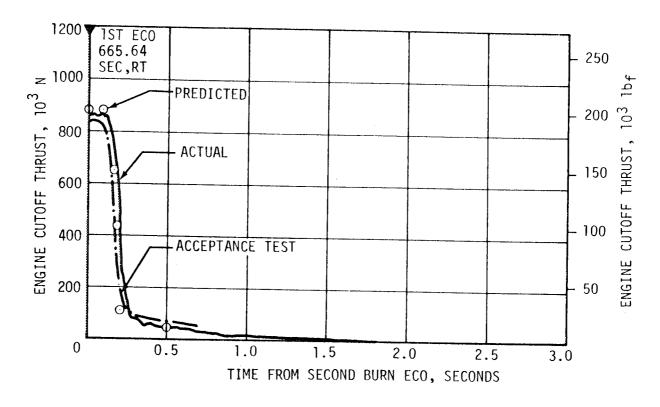
Figure 7-15. S-IVB Shutdown Transient - Second Burn
