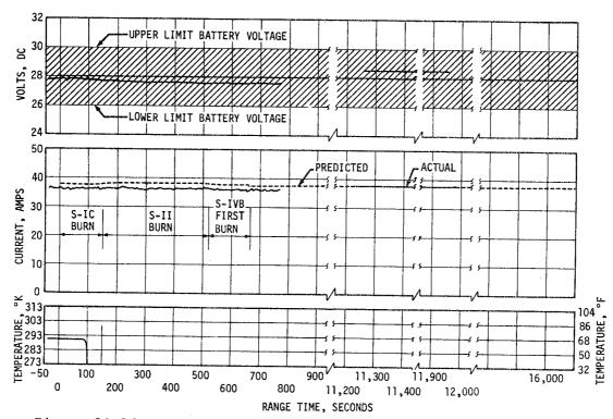
Figure 13-14. IU Battery 6D40 Voltage, Current, and Temperature
