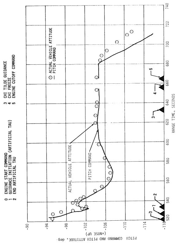
Figure 11-29. Vehicle Attitude During S-IVB First Burn
