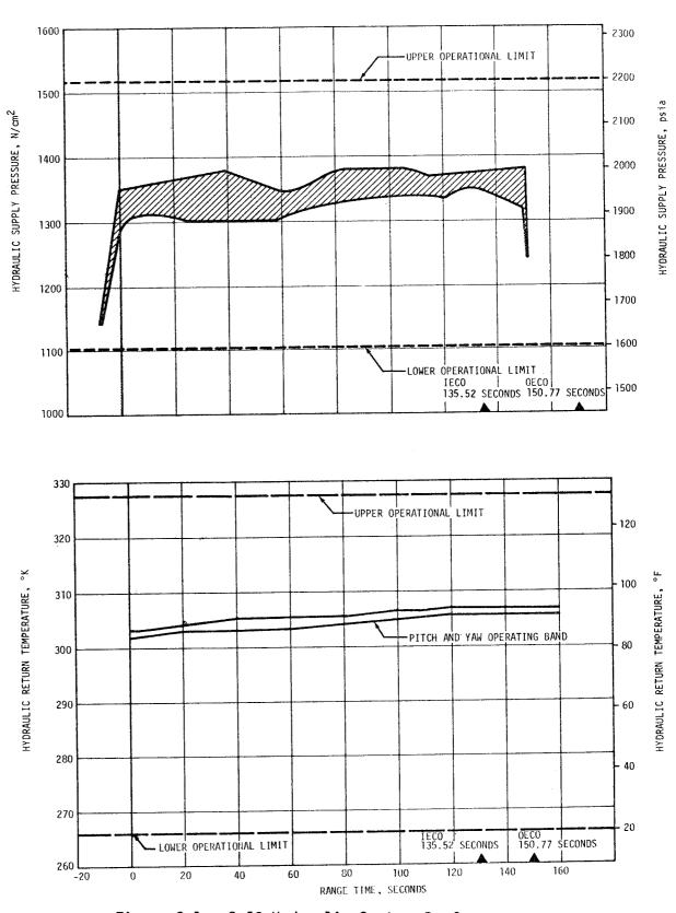
Figure 8-1. S-IC Hydraulic System Performance
