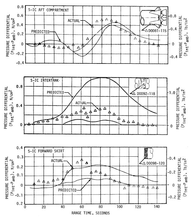
Figure 16-2. S-IC Compartment Pressure Differentials
