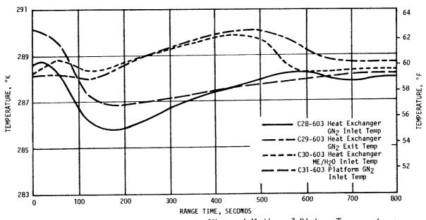
Figure 18-8. Heat Exchanger GN<sub>2</sub> and Methanol/Water Temperatures
