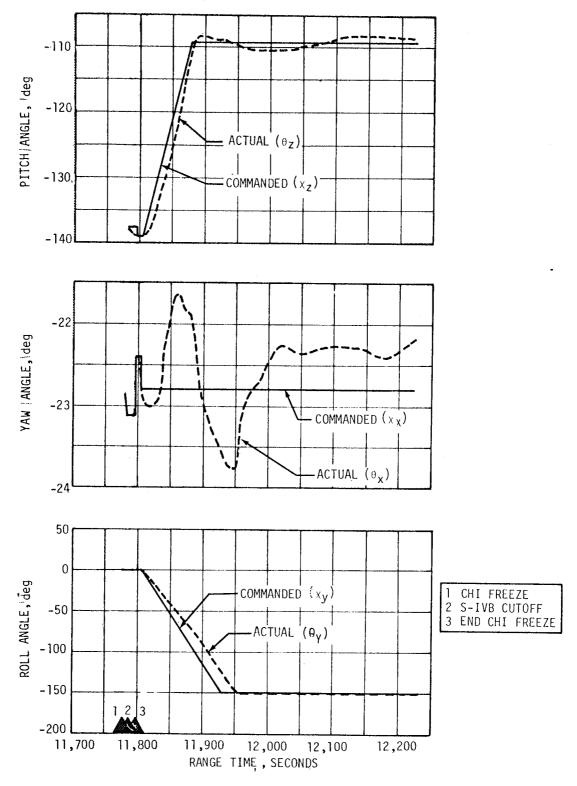
Figure / 11-38 Vehicle Attitude Prior to Spacecraft Separation
