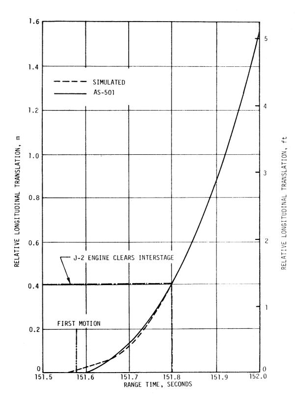
Figure 12-4. S-IC/S-II Separation Distance
