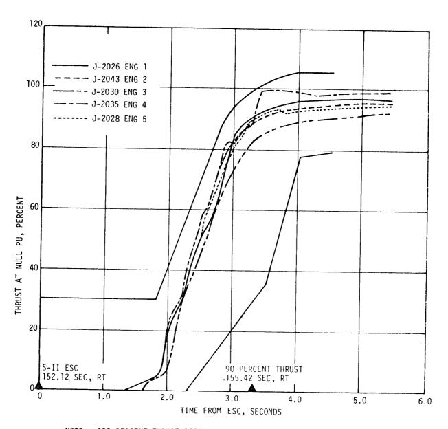
NOTE: 100 PERCENT THRUST BASED ON ENGINE THRUST AT 60 SECOND TIME SLICE.
