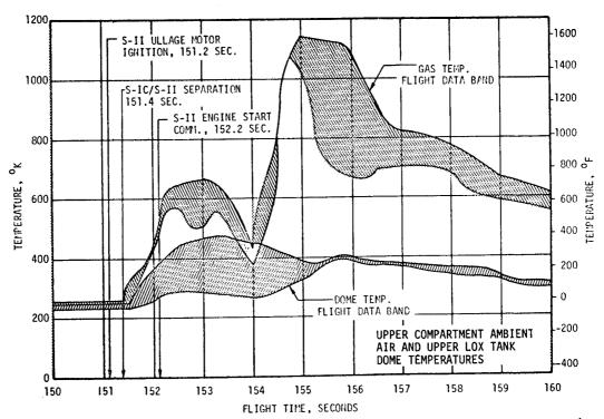
Figure 17-4. S-IC Interstage Thermal Environment During Separation
