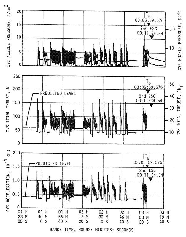
Figure 7-8. S-IVB CVS Performance - Coast Phase, Sheet 2 of 2
