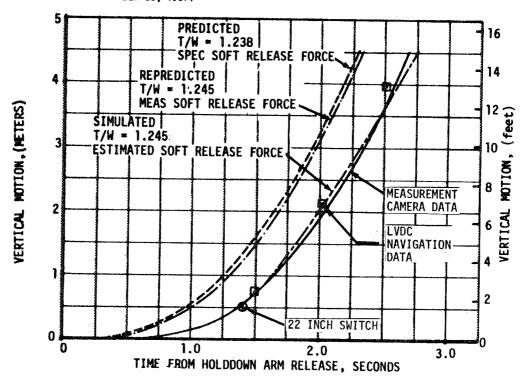
Figure 11-2. Liftoff Vertical Motion
