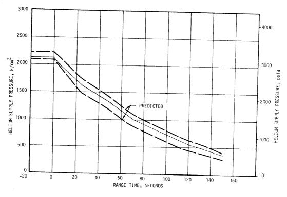
Figure 5-8. S-IC Helium Bottle Pressure for Fuel Pressurization
