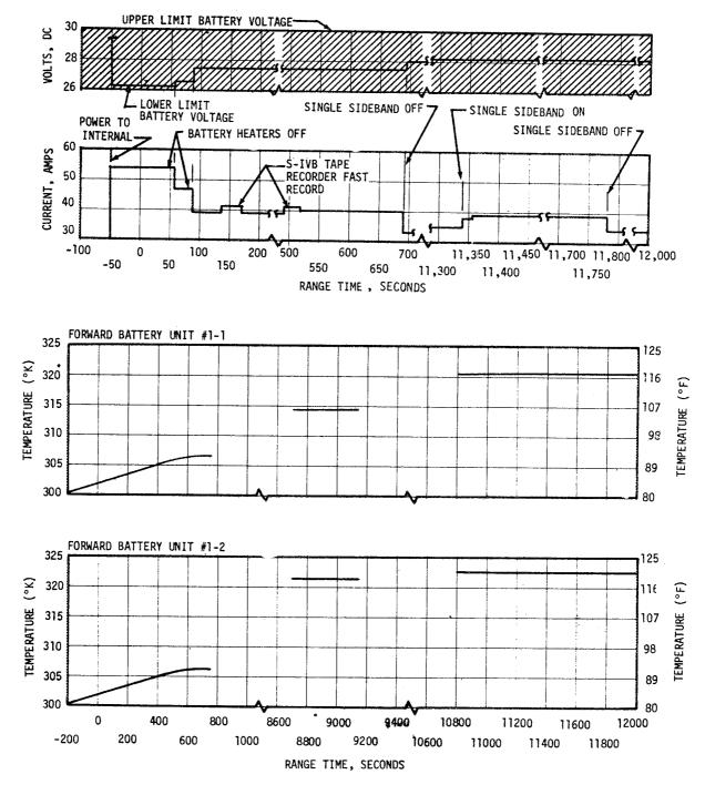
NOTE: PREDICTED CURRENT WAS BASED ON MAXIMUM LOADS. VALUES ARE BEYOND THE SCALE OF THESE PLOTS AND THEREFORE NOT SHOWN. ACTUAL CURRENT FELL WELL BELOW PREDICTED.
