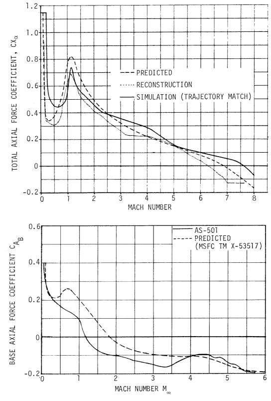
Figure 20-1. Vehicle Axial Force Characteristics
