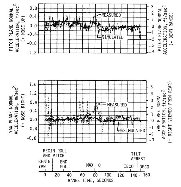
Figure 11-14. Normal Acceleration During S-IC Powered Flight
