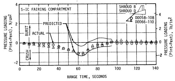
Figure 16-1. S-IC Engine Fairing Compartment Pressure Differential and Aerodynamic Loads
