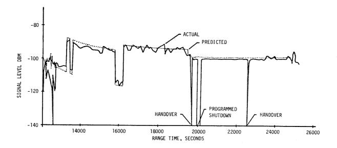
Figure 19-8. Ascension CCS Down Link Carrier Signal Strength, AS-501
