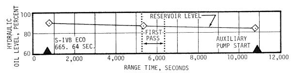
Figure 8-4. S-IVB Hydraulic System Performance - Coast Phase
