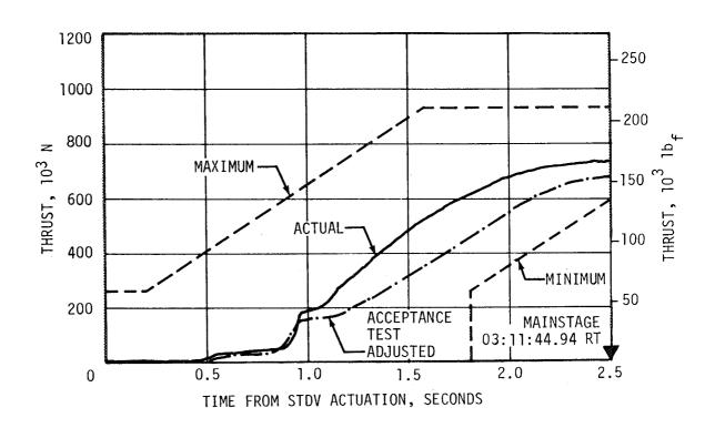
Figure 7-13. S-IVB Buildup Transient - Second Burn
