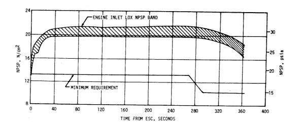
Figure 6-18. S-II LOX Pump Inlet Conditions
