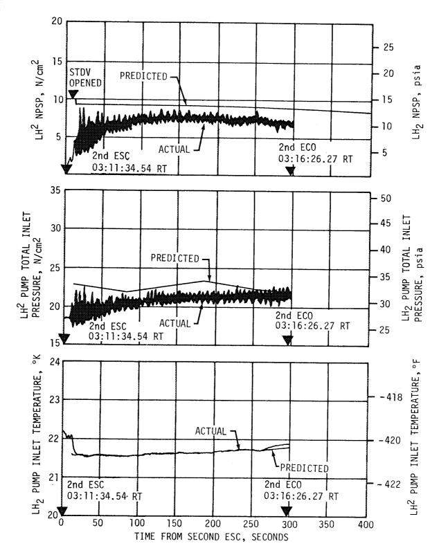
Figure 7-24. S-IVB Fuel Pump Inlet Conditions - Second Burn
