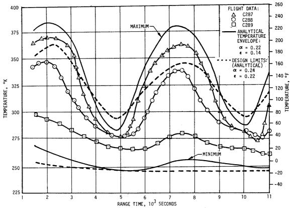
Figure 17-17. APS Fairing Orbital Temperature
