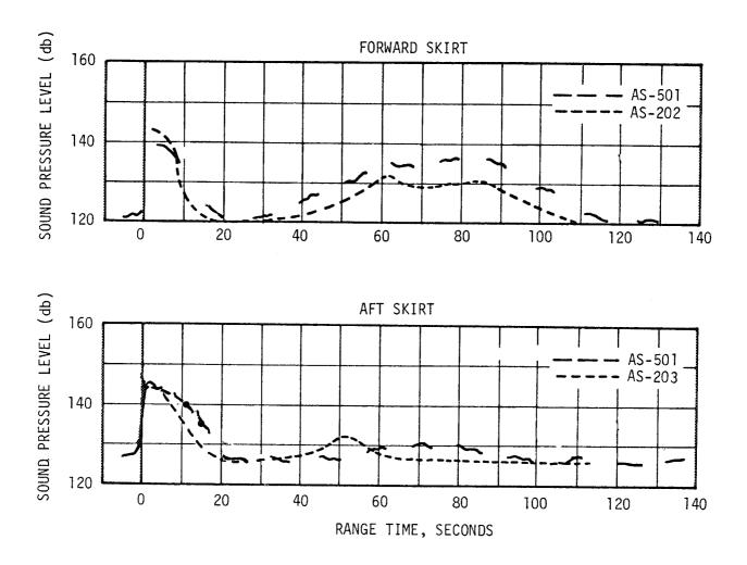
Figure 16-14. S-IVB Internal Sound Pressure Levels
