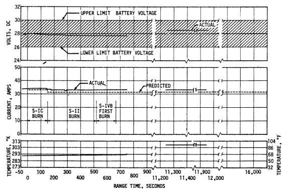
Figure 13-12. IU Battery 6D20 Voltage, Current, and Temperature
