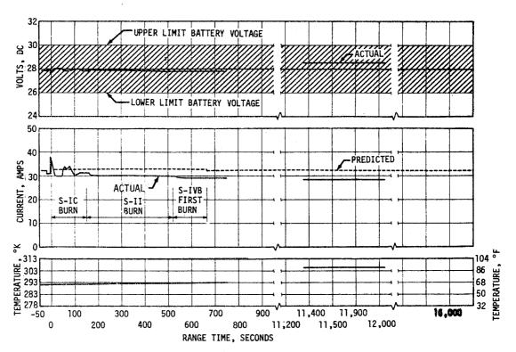
Figure 13-11. IU Battery 6D10 VoTtage, Current, and Temperature
