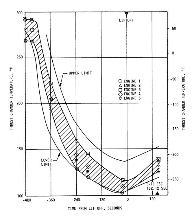
Figure 6-1. S-II Thrust Chamber Temperatures
