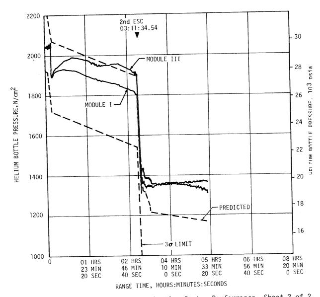
Figure 7-34. S-IVB APS Pressurization System Performance, Sheet 2 of 2 to  $38 \text{ N/cm}^2$  (55 psia). A possible cause of this anomaly was a restriction of propellant flow to the engine.
