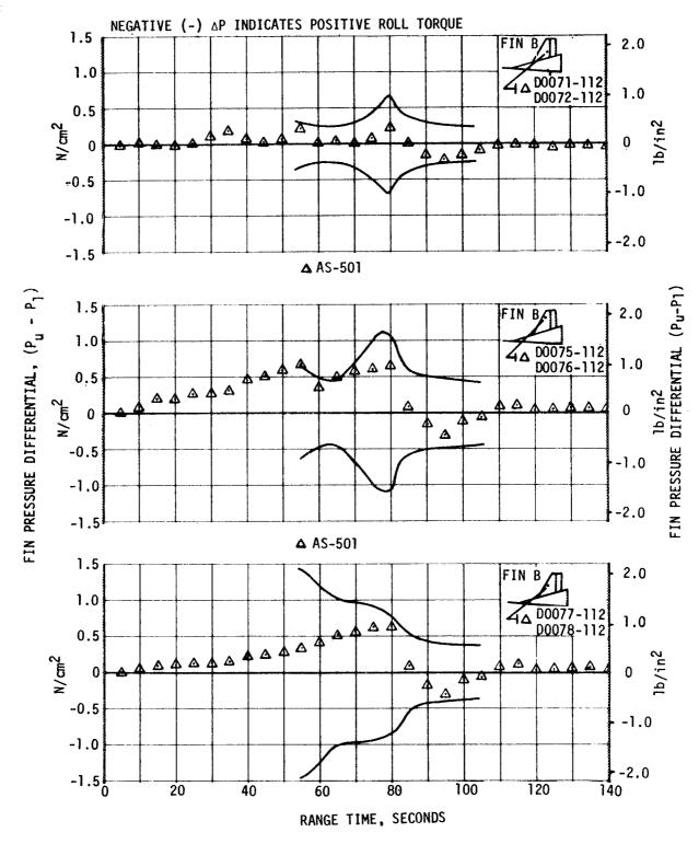
Figure 20-3. S-IC Fin Pressure Differential, Sheet 1 of 2
