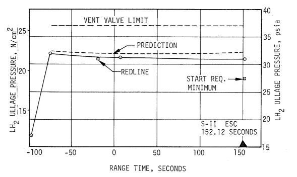
Figure 6-12. S-II LH<sub>2</sub> Tank Ullage Pressure During Prepress and S-IC Boost
