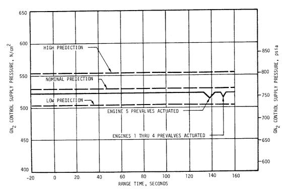
Figure 5-10. S-IC Pneumatic Control Regulator Outlet Pressure
