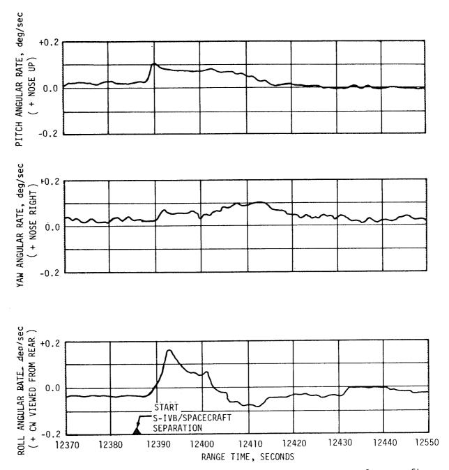
Figure 12-17. S-IVB Angular Rate During Separation from Spacecraft
