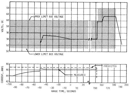
Figure 13-5. S-II Stage Recirculation DC Bus Voltage and Current
