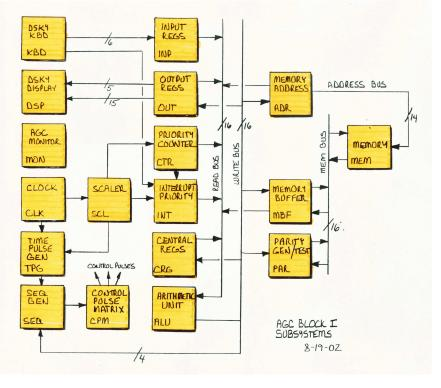
The MON, CLK, SCL, TPG, SEQ, and CPM subsystems generated the timing and control pulses that run all the other subsystems, so I gathered them into a CTL (control) module (in part 2).
