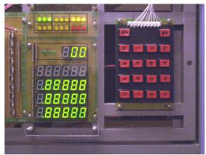
Load component 1 for dataset at octal address 50 with octal 123:
