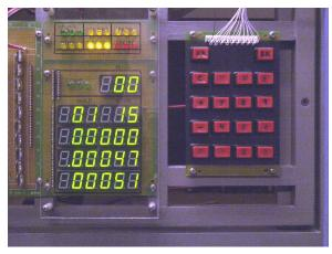
The octal word in address 51 is displayed in R1, incremented address in R3. <ENTER>
