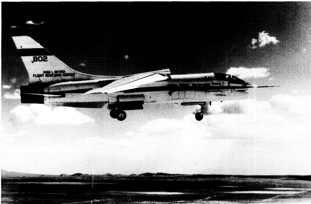
Figure 4-3. The F-8 aircraft that proved the redundant set configuration planned for the Shuttle would work. (NASA photo ECN-6988)
