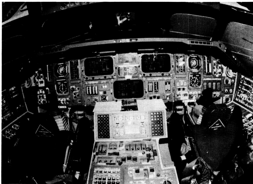
Figure 4-7. The forward flight deck of a Shuttle, with the three CRT screens and twin keyboards visible in the center. (NASA photo S80-35133)
