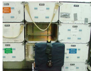
10. Open middeck locker MF43K for RSK 6, MF57K for RSK 7. (Figure shows MF57K open for RSK 7)
