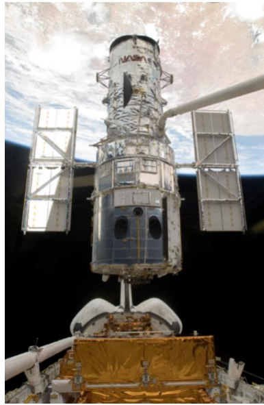
Figure 11. The HST Being Deployed from the Shuttle Using the RMS. (Courtesy NASA)
