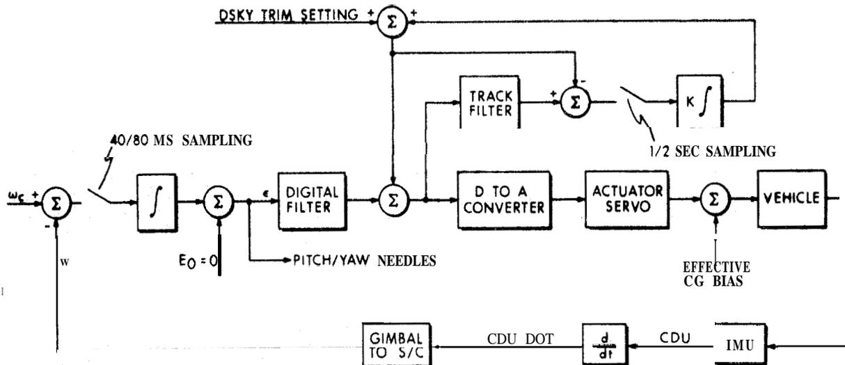
Figure 8. Powered flight autopilot
