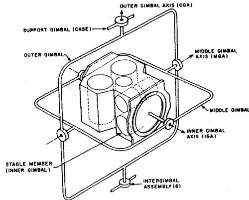
Figure 5. IMU schematic diagram
