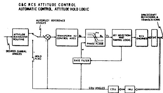
Figure 7. Coasting flight autopilot
