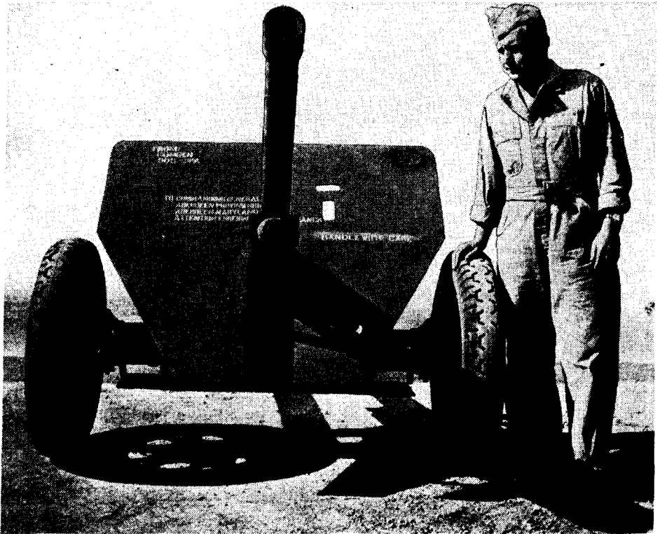
Figure 117.—Type 1 (1941) 47-mm antitank gun showing shape of shield.
