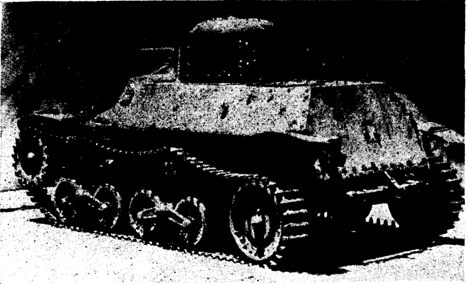
Figure 13.—Type 97 (1937) tankette, left rear three-quarters.
