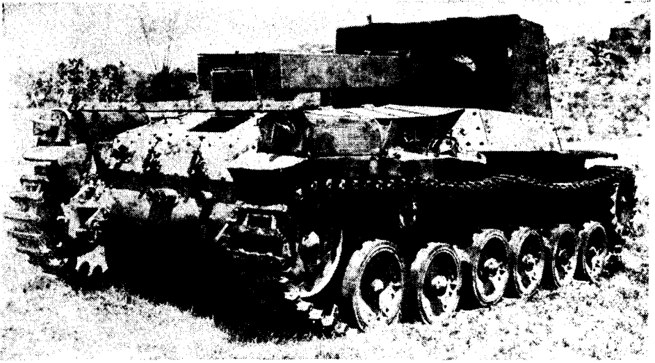
Figure 83.—Type 38 (1905) 15-cm howitzer mounted on Type 97 (1937) medium tank chassis, right rear three-quarters showing ammunition stowage box located above engine.
