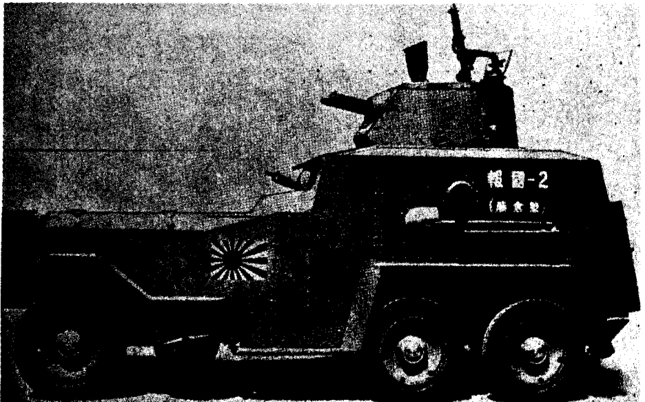
Figure 89.—Type 92 (1932) Navy armored car.
