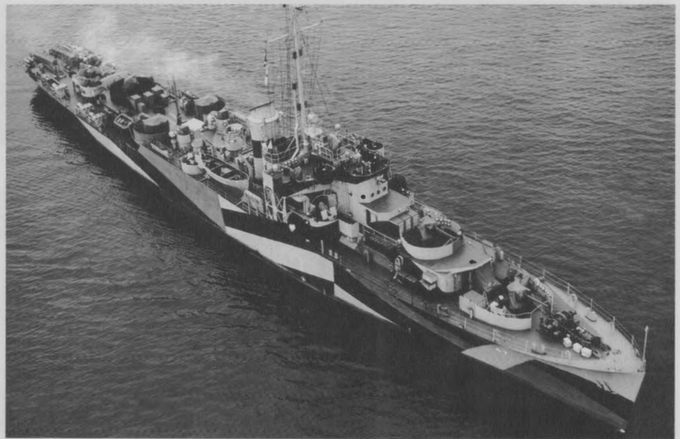
Gallup (PF 47) wearing camouflage at San Pedro, Calif., on 30 May 1944. BUSHIPS conceived this scheme (which involved dull black, ocean gray, light gray, and deck blue paint) specifically for the frigate.
