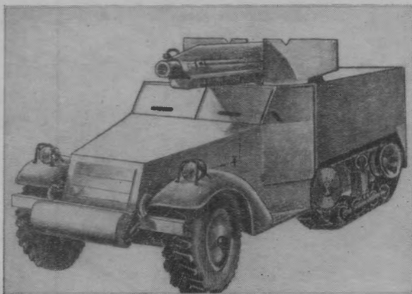
Figure 1. M3 T/2 mounting 75-mm howitzer.
