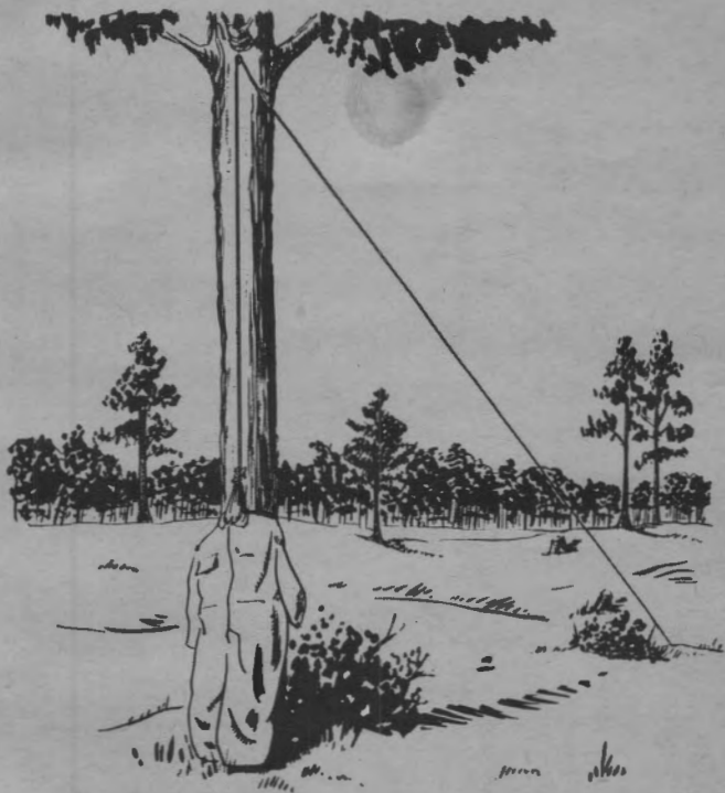
FIGURE 113.—Method of raising surprise target in tree (sniper).
