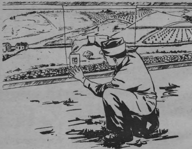
FIGURE 95.—Lining in scoring area (point target) with scoring template.
