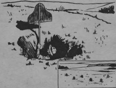
FIGURE 108.—Method of displaying surprise target to represent skirmishers. (Cut-away in rear of pit prevents ricochet rounds from rebounding into pit.)
