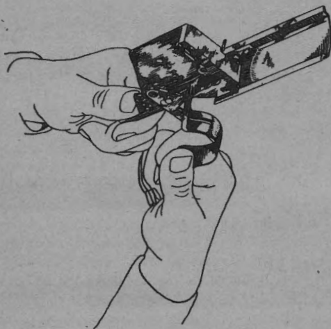
FIGURE 13.—Removing trigger guard from trigger housing group. from barrel, tap lightly (toward muzzle) on the bayonet stud. The front sight will not be dismounted from the gas cylinder assembly. Do not attempt to adjust the front sight.
