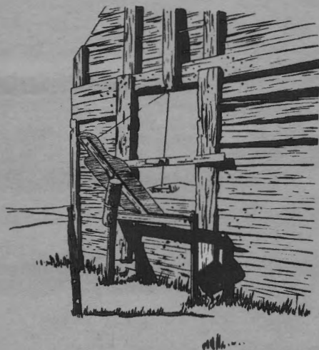
FIGURE 112.—Method of raising surprise target from pit.
