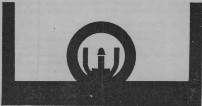
FIG. 9.—Alignment of sights and target, model 1917 rifle. Aiming at head target.
