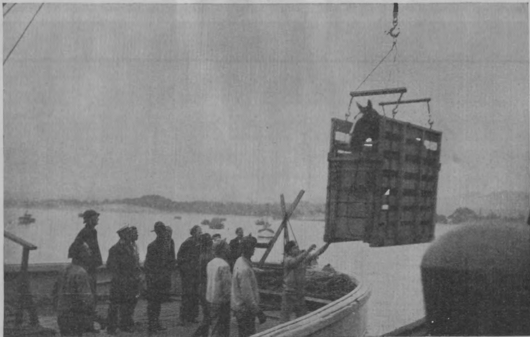
FIGURE 13.—Lowering animal from transport to motor launch by means of flying stall.
