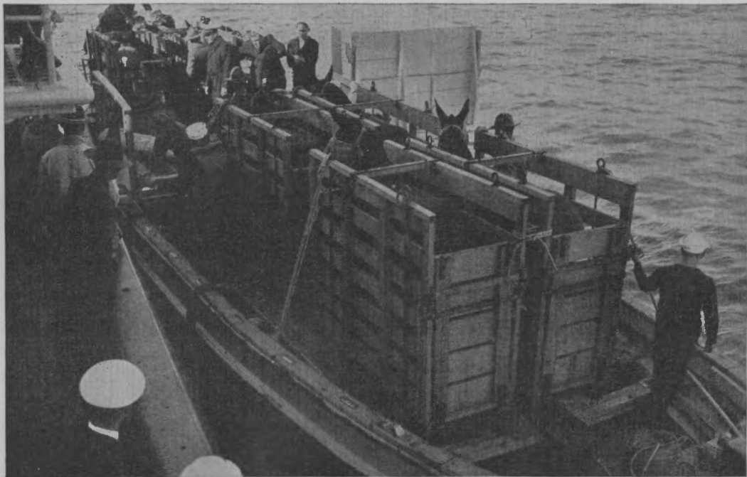
FIGURE 14.—Disposition of flying stalls on motor launch. Note dumping stall projecting over water at right.
