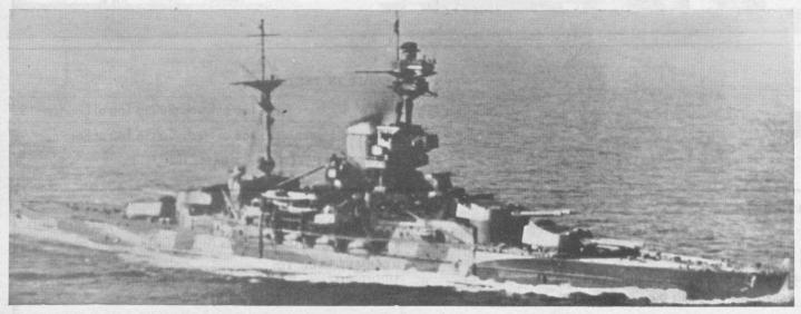
REVENGE 1941 The only unit with after edge of upper bridge extended towards the stack.
