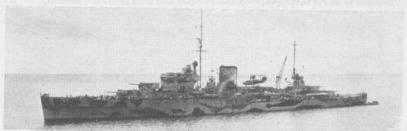
ACHILLES — tripod masts not fitted.
