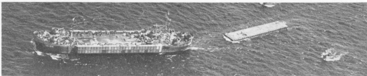
▼ LST carrying two "causeways," towing another
