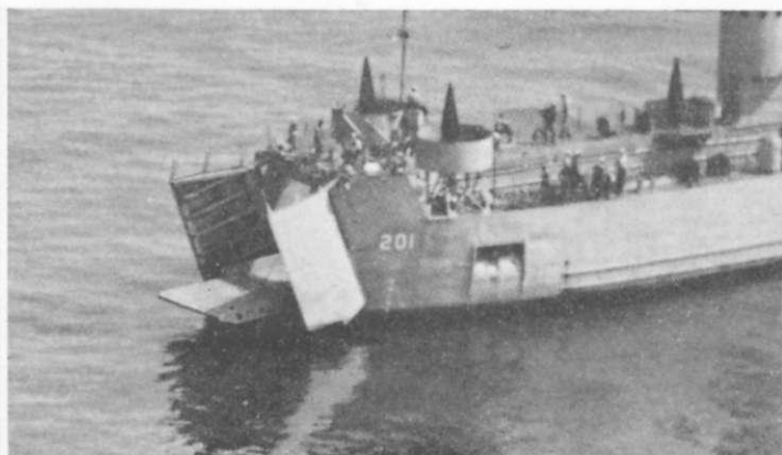
Note new 40 mm gun mount on bow ▲
