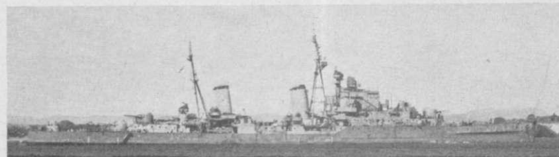
PHOEBE — note that two turrets forward have been removed.
