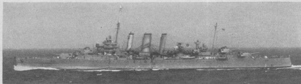
AUSTRALIA — the only unit with pole masts and her heavy A.A. battery mounted on the main deck instead of on the shelter deck.
