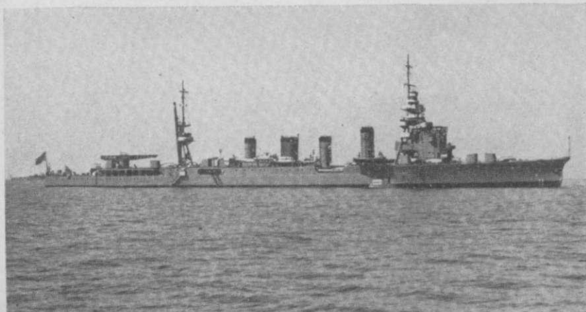
JINTSU—NAKA HAS MAINMAST TRIPOD REVERSED
