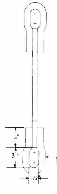
1" DIA ROD BENT TO TAKE CONNECTING SHACKLE
