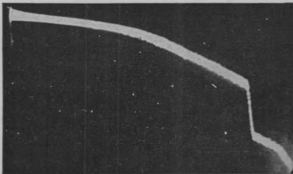
A. Air search radar A scope. The trace is wiped clean and is distorted by the overloading of the receiver.
