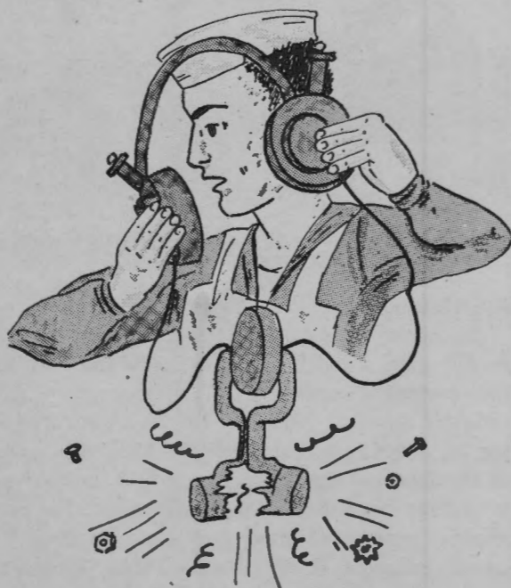
Figure 6-3. In case of casualty to the transmitter, speak into one earpiece and listen through the other.
