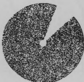
B. Bright sector caused by non-synchronous jamming.
