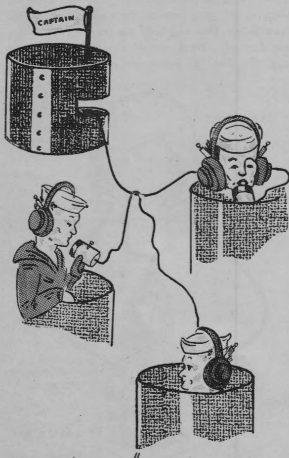
Figure 6-1. The JA circuit connects the Captain's battle station with control stations throughout the ship.
