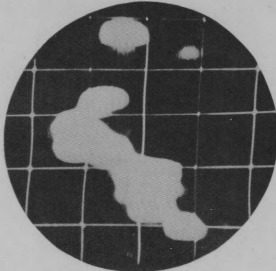
B. B scope showing enlarged presentation of targets seen within the brightened segment in A. The grid is formed by range and bearing lines.
