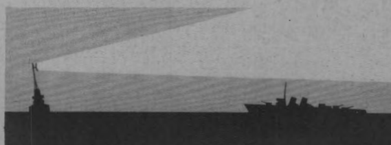
Figure 101—Effect of roll of ship on antenna coverage.
