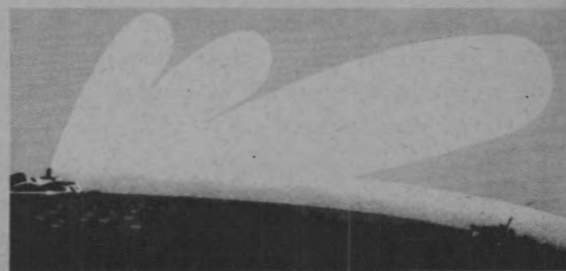
B. Radar lobe pattern in nonstandard atmosphere. . . . A duct has been formed on the surface and ship is detected.
