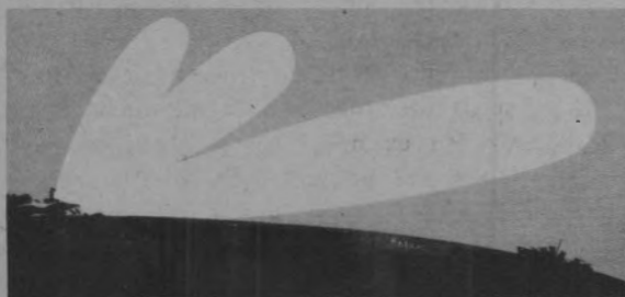
A. Radar lobe pattern in standard atmosphere. . . . Steady variation of temperature and humidity aloft.
