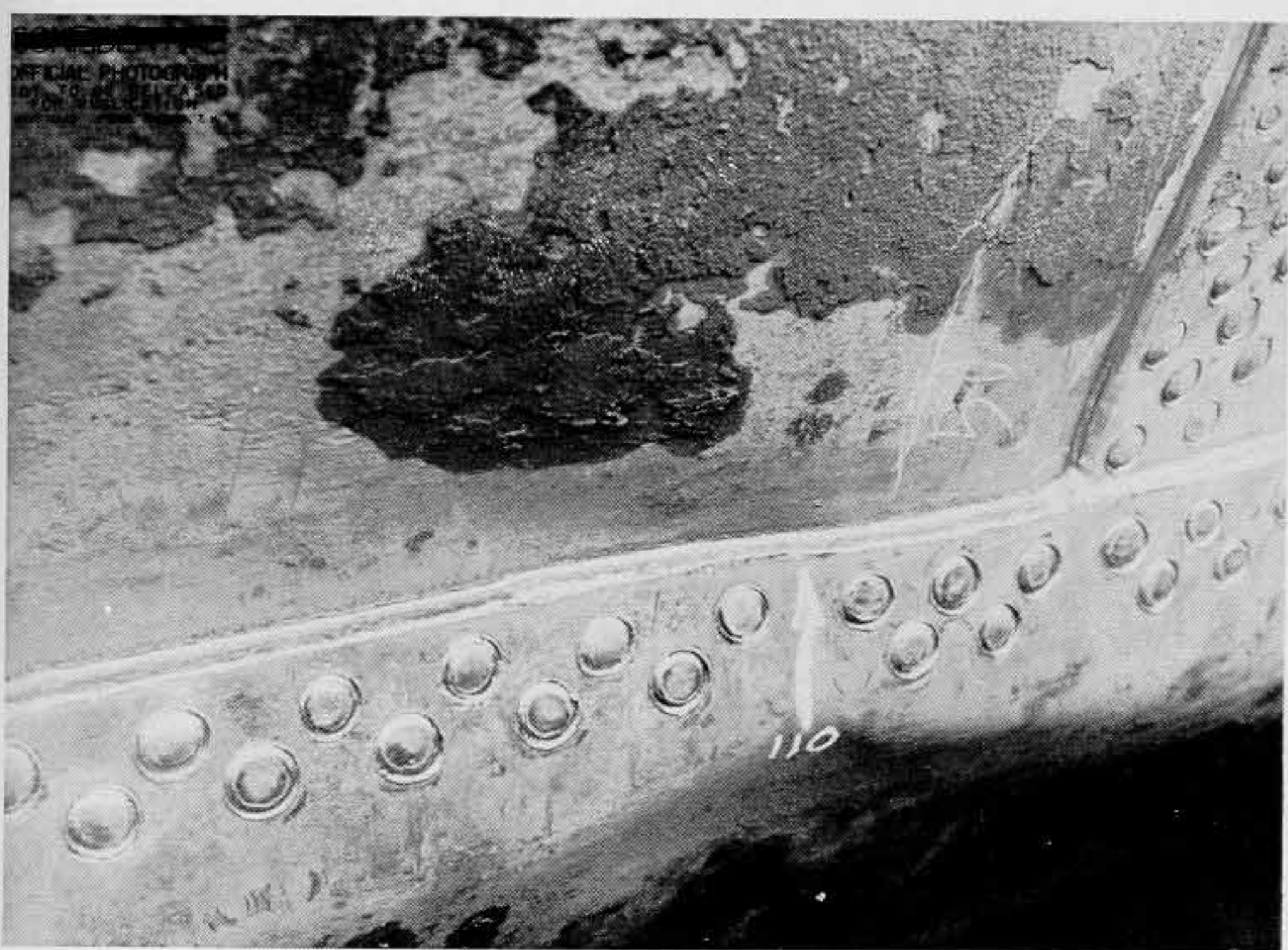
Photo 3: Bomb Damage to Port Shell, FR 110, details of temporary repairs.
