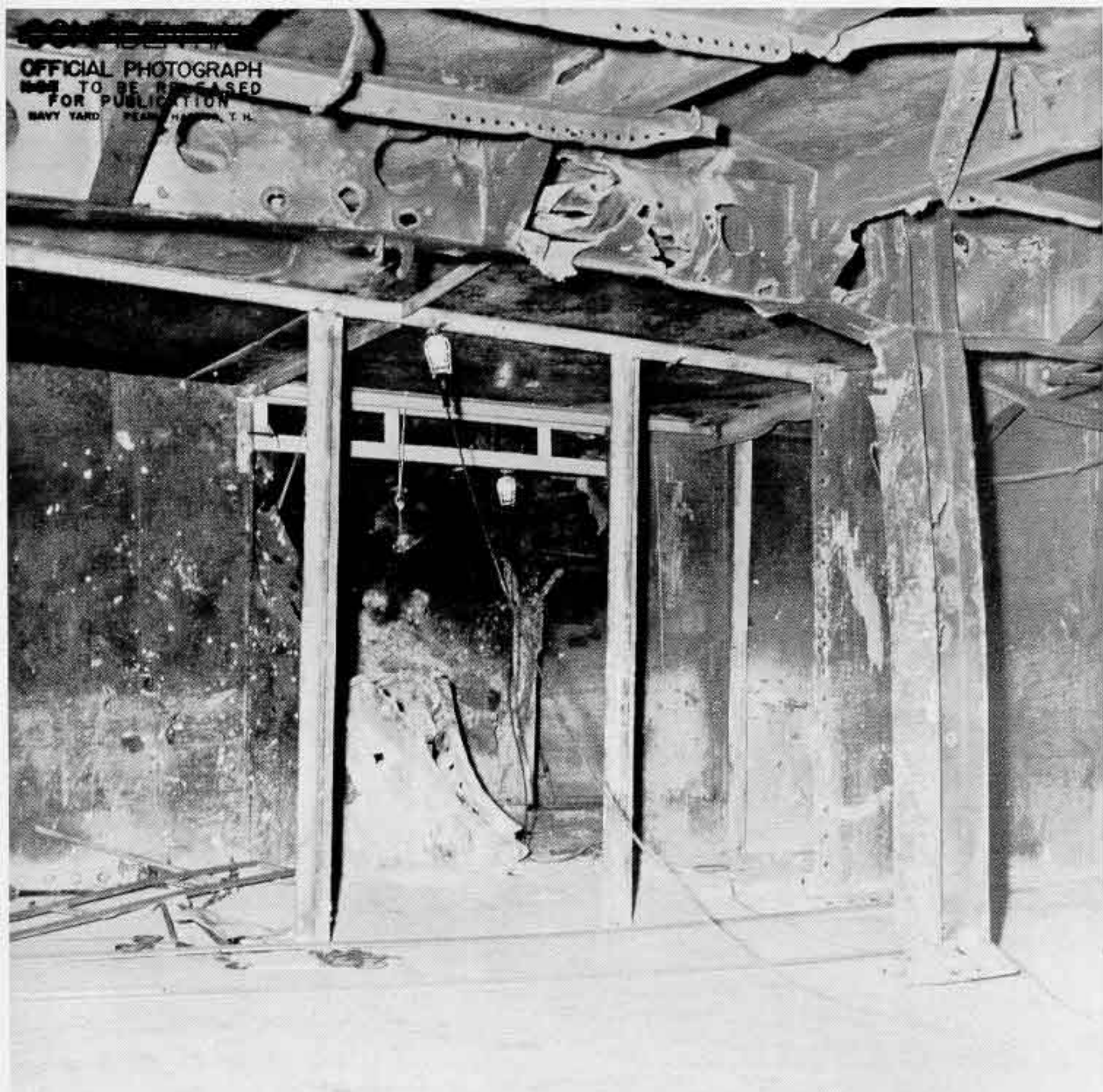
Photo 17: Between 4th and 3rd decks, looking forward and to starboard. Note that 4th (armored) deck is undamaged and that web frame 109 is virtually cut in two.
