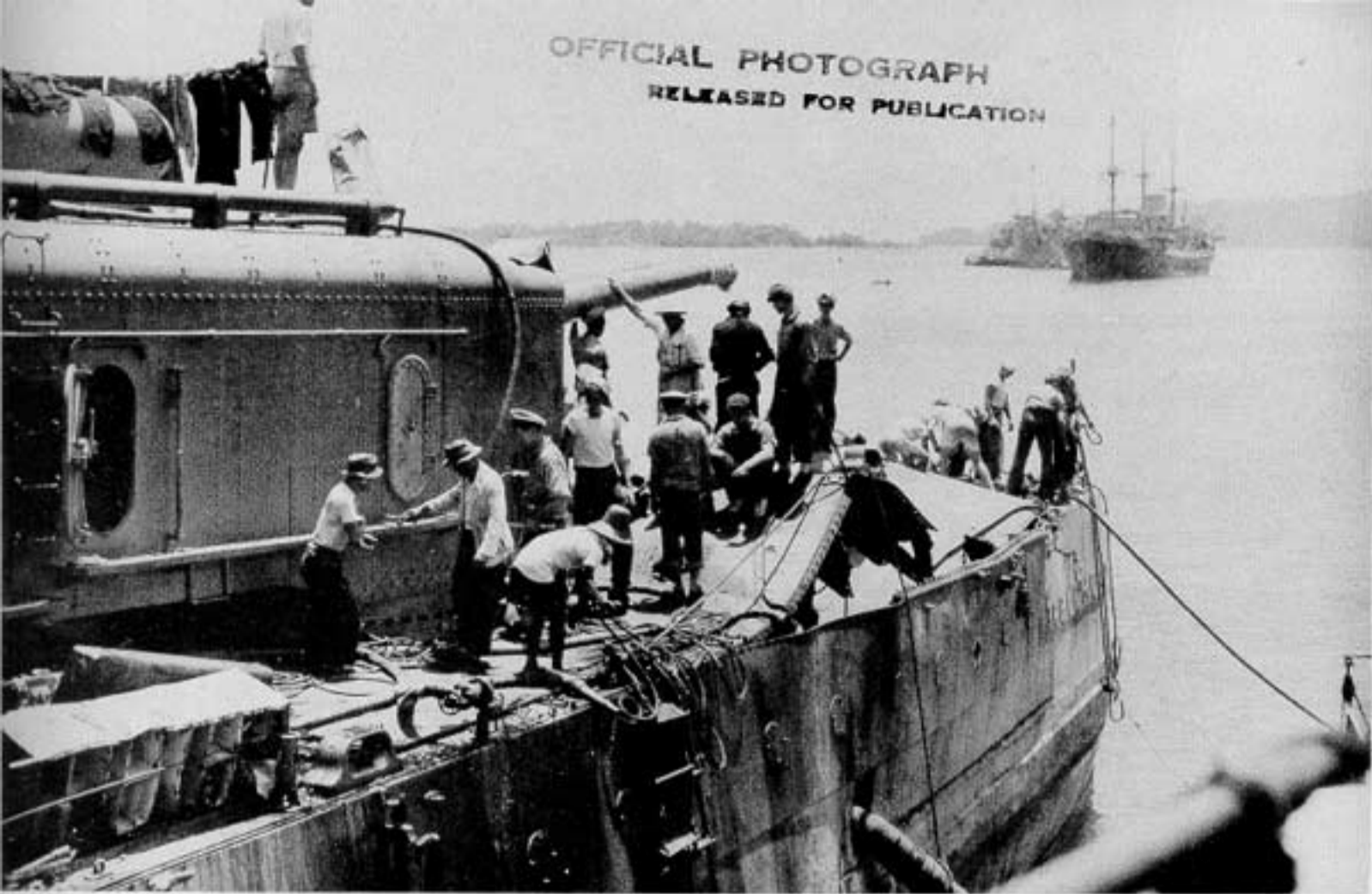
Photo 1: View of damage to main deck at fantail.
