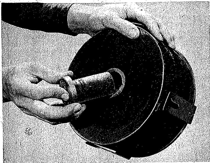
4. Make sure shear pin is in place.
