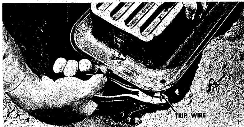
4. Search for booby traps. Cut any trip wires attached to hole in base flange. Lift mine.
