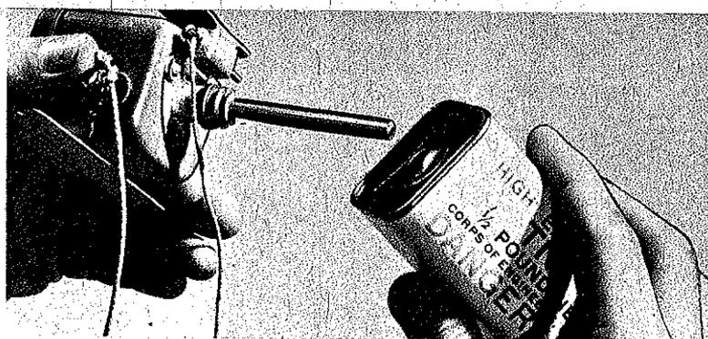
5. Insert cap in charge or, if detonating cord is used, tape one end to cap and run other end to charge.
