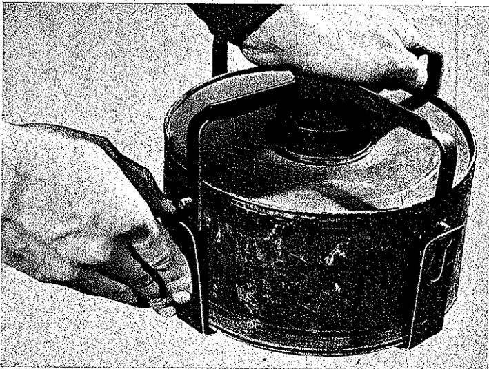
7. Replace spider, making sure pins engage in slots in straps.
