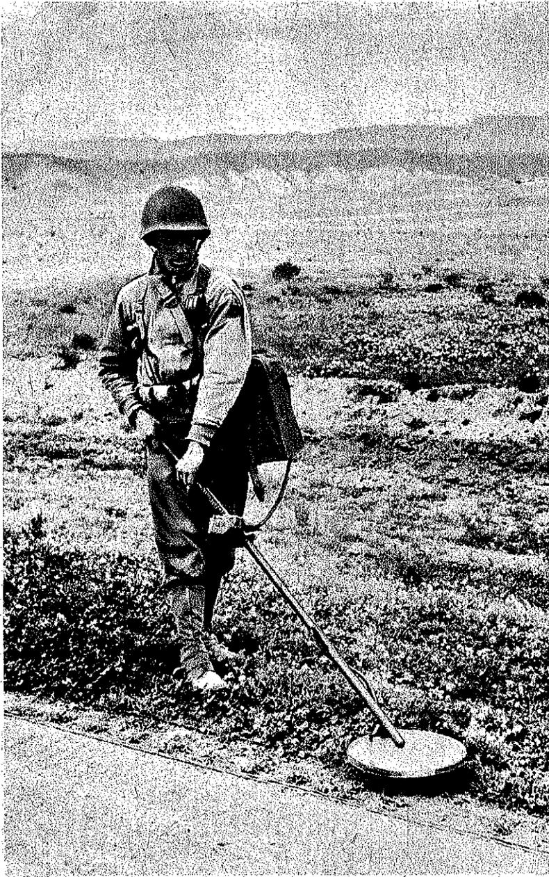
*Figure 1.2. Electrical mine detector.*
