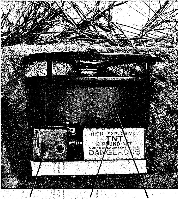
RELEASE FUZE M1      CHARGE      (AT) MINE M1. OR M1A1
