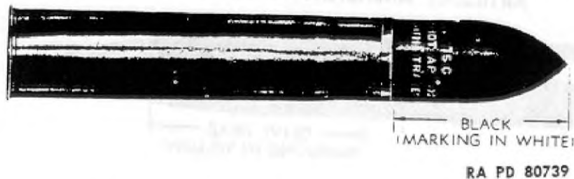
Figure 63 — SHOT, Fixed, A.P., M72, w/TRACER, 75-mm Gun
