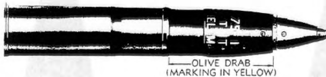
Figure 75 — SHELL, Semifixed, H.E., M41A1, w/FUZE, P.D., M48A2, SQ & 0.15-sec. Delay, 75-mm How., M1, M1A1, M2, and M3
