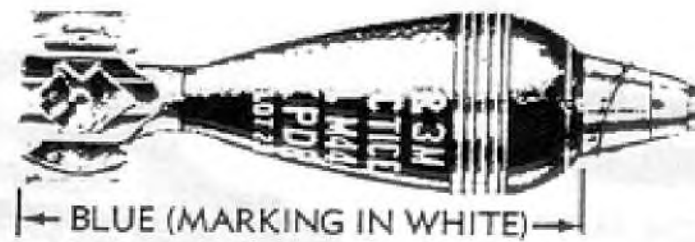
Figure 103 — SHELL, Practice, M44, w/FUZE, P.D., M52, 81-mm Mortar, Complete Round
