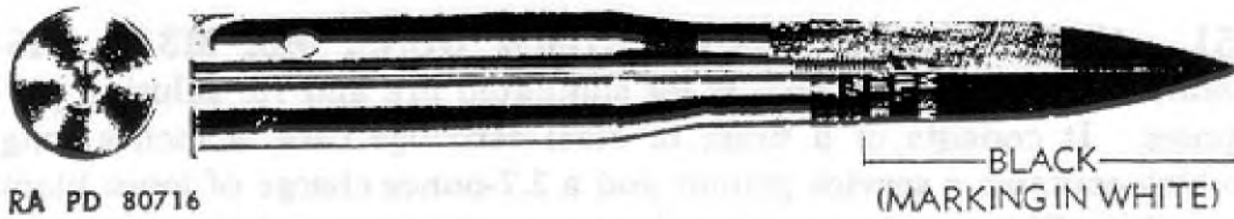
Figure 47 — CARTRIDGE, Drill, M13, 37-mm Guns, M3, M3A1, M5, M5A1, and M6
