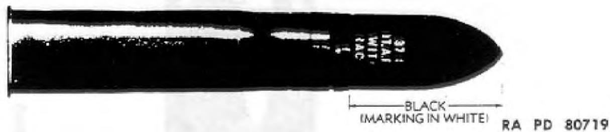
Figure 43 — SHOT, Fixed, A.P., M80, w/TRACER, 37-mm Auto. Guns, AN-M4 and M10 (Aircraft)
