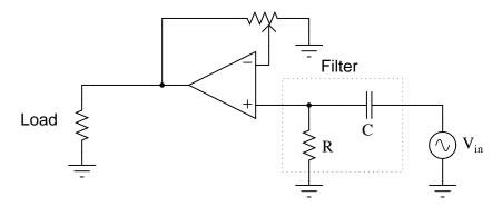
Determine the type (LP, HP, BP, BS) and cutoff frequency of this active filter circuit:
