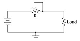
It should be obvious in this circuit that the load current decreases as variable resistance R increases. What might not be so obvious is that the aforementioned switched capacitor circuit *emulates* the variable resistor R in the second circuit, so that there is a mathematical equivalence between f and C in the first circuit, and R in the second circuit, so far as average current is concerned. To put this in simpler terms, the switched capacitor network behaves sort of like a variable resistor.
