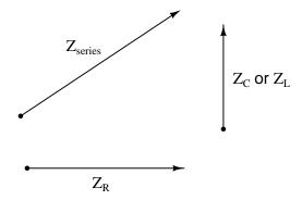
Since the phasor for resistive impedance  $(Z_R)$  has an angle of zero degrees and the phasor for reactive impedance  $(Z_C \text{ or } Z_L)$  either has an angle of +90 or -90 degrees, the *phasor sum* representing total series impedance will form the hypotenuse of a right triangle when the first to phasors are added (tip-to-tail).
