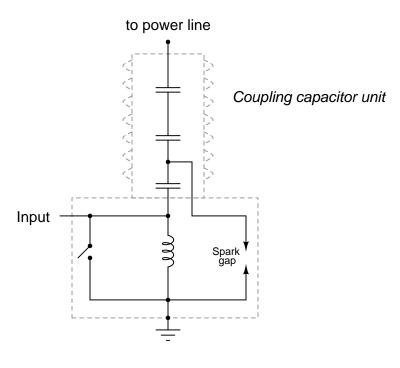
Explain how such a spark gap is supposed to work, and why it functions as an over-voltage protection device.
