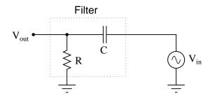
Give an exact equation predicting this filter circuit's cutoff frequency, and also identify what type of filter it is.
