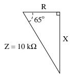
We know that the *sine* function relates the sides X and Z of this impedance triangle with the 65 degree angle, because the sine of an angle is the ratio of *opposite* to *hypotenuse*, with X being opposite the 65 degree angle. Therefore, we know we can set up the following equation relating these quantities together:
