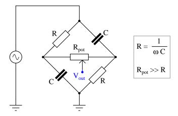
Suppose, though, that the output signal is stuck at  $-45^{o}$  lagging the source voltage, no matter where the potentiometer is set. Identify a likely failure that could cause this to happen, and explain why this failure could account for the circuit's strange behavior.
