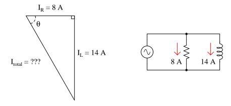
Calculate the total current and the angle  $\Theta$  of the total current, explaining your trigonometric method(s) of solution.
