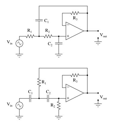
Determine which of these Sallen-Key filters is low pass, and which is high pass. Explain your answers.  $\underline{\text{file }00765}$
