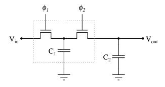
$$f_{-3dB} = \frac{f_{switch}C_1}{2\pi C_2}$$
