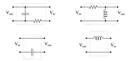
Identify what type of filter this circuit is, and calculate its cutoff frequency given a resistor value of 1  $k\Omega$  and a capacitor value of 0.22  $\mu$ F:
