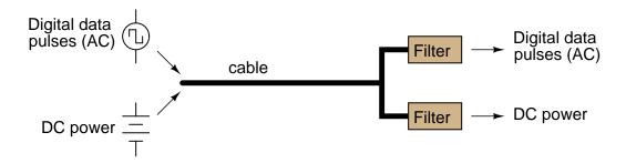
Filter circuits are also necessary on the transmission end of the cable, to prevent the AC signals from being shunted by the DC power supply's capacitors, and to prevent the DC voltage from damaging the sensitive circuitry generating the AC voltage pulses.
