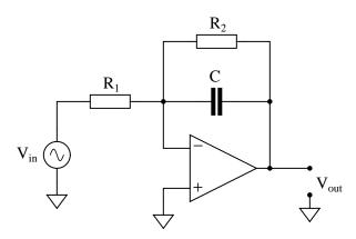
These are both low pass filters. The circuit with the shunt capacitor is the more practical one, because its voltage gain remains finite for all possible input signal frequencies:
