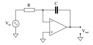
Also, describe what result the change in impedances will have on the op-amp circuit's voltage gain. If the input signal amplitude remains constant as frequency increases, what will happen to the amplitude of the output voltage? What type of filtering function does this behavior represent?
