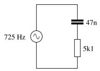
Also, calculate the total impedance  $(Z_{total})$  of this circuit, expressing it in both rectangular and polar forms.
