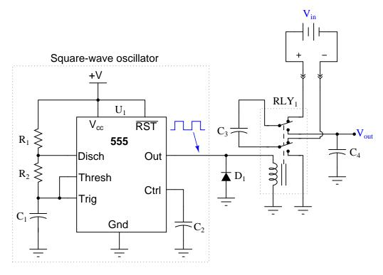
This type of circuit is often referred to as a *flying capacitor* circuit, with  $C_3$  being the "flying" capacitor. Explain why this is, and what possible benefit might be realized by using a flying capacitor circuit to sample a voltage.
