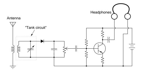
The "tank circuit" formed of a parallel-connected inductor and capacitor network performs a very important filtering function in this circuit. Describe what this filtering function is. file 00611
