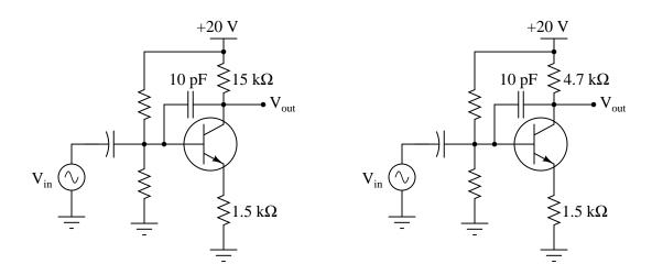
A common problem encountered in the development of transistor amplifier circuits is unwanted oscillation resulting from parasitic capacitance and inductance forming a positive feedback loop from output to input. Often, these parasitic parameters are quite small (nanohenrys and picofarads), resulting in very high oscillation frequencies.
