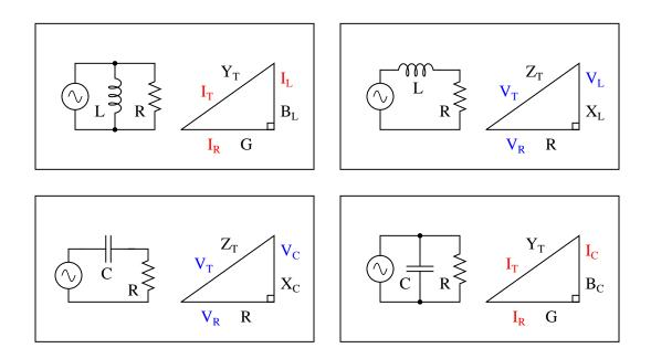
$X = 105 \Omega$ , as calculated by an algebraically manipulated version of the Pythagorean Theorem.
