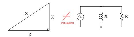
Examine the following circuits, then label the sides of their respective triangles with all the variables that are trigonometrically related in those circuits:
