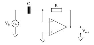
Also, describe what result the change in impedances will have on the op-amp circuit's voltage gain. If the input signal amplitude remains constant as frequency increases, what will happen to the amplitude of the output voltage? What type of filtering function does this behavior represent?
