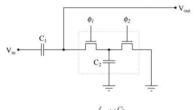
$$f_{-3dB} = \frac{f_{switch}C_2}{2\pi C_1}$$
