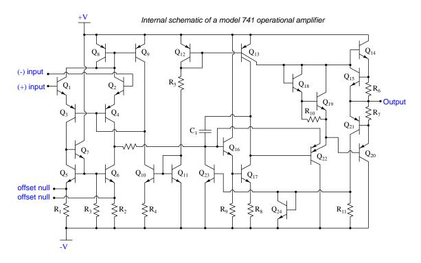
Explain how active loading creates the constant slew rate exhibited by operational amplifier circuits such as the 741. What factors account for the *linear* ramping of voltage over time? file 02603
