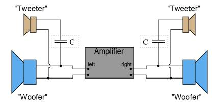
Follow-up question: what type of capacitor would you recommend using in this application (electrolytic, mylar, ceramic, etc.)? Why?
