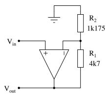
Algebraically manipulate the gain equation to solve for  $R_2$ , then determine the necessary value of  $R_2$  in this circuit to give it a voltage gain of 6.8.
