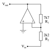
Algebraically manipulate the gain equation to solve for  $R_2$ , then determine the necessary value of  $R_2$  in this circuit to give it a voltage gain of 4.9.
