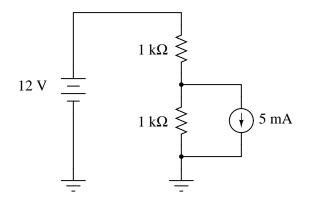
Hint: it may help you to set up the necessary equation by labeling the current through the lower resistor as I and the current through the upper resistor as I + 0.005. file 03116
