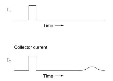
The instantaneous effect of the first pulse (precisely timed with the closure of the switch) is not the most interesting facet of this experiment. Rather, the second (delayed) pulse is. Explain what caused this second pulse, and why its shape depended on  $V_{drift}$ . file 02044
