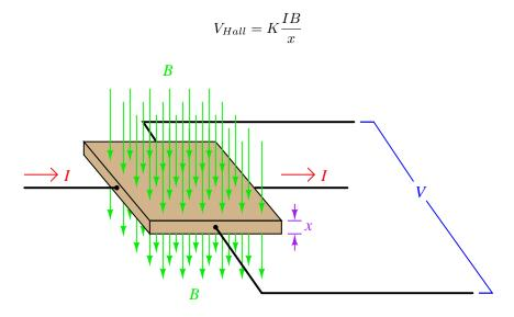
Explain what this equation means with regard to the effect of each variable (I, B, and x) on the Hall voltage generated. Identify whether each of the variables has a *direct* or an *inverse* effect on the output voltage.
