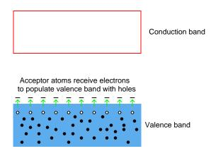
In either case, the addition of impurities to an otherwise pure semiconductor material increases the number of available charge carriers.
