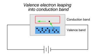
With sufficient thermal energy, these electron-hole pairs will form spontaneously. At room temperature, however, this activity is slight.
