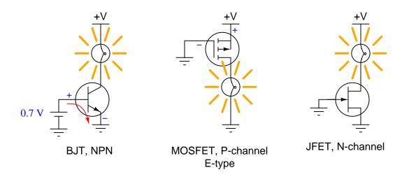
Follow-up question: for the JFET, which is already "on" with zero voltage applied to the gate, describe what would be necessary to force it into the "off" state.
