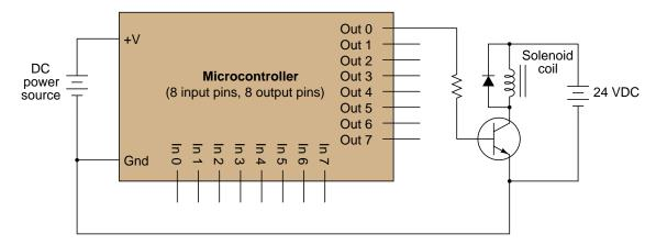
Unfortunately, a single BJT does not provide enough current gain to actuate the solenoid. With 20 mA of output current from the microcontroller pin and a  $\beta$  of only 25 (typical for a power transistor), this only provides about 500 mA to the solenoid coil.
