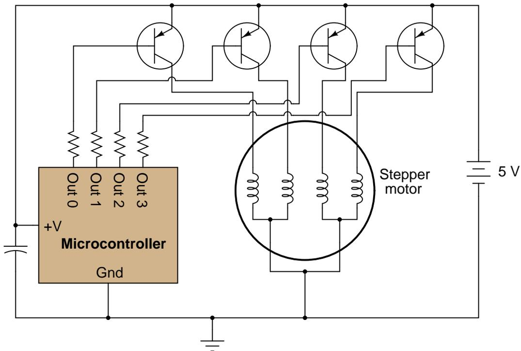
Each motor coil draws a relatively heavy current when energized, necessitating transistors to "interpose" between the microcontroller outputs and the motor coils.
